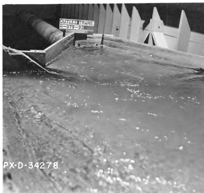
A. Mildly turbulent water surface. Q = 2.4 , V_p = 3.0 , depth = 0.8D .
