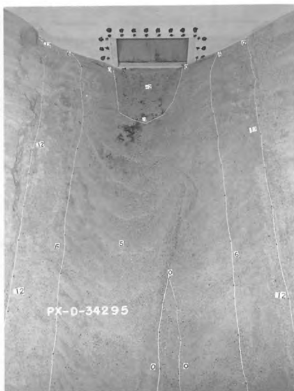
B. Scour after 1 hour operation. Canal depth = 1.00D .
