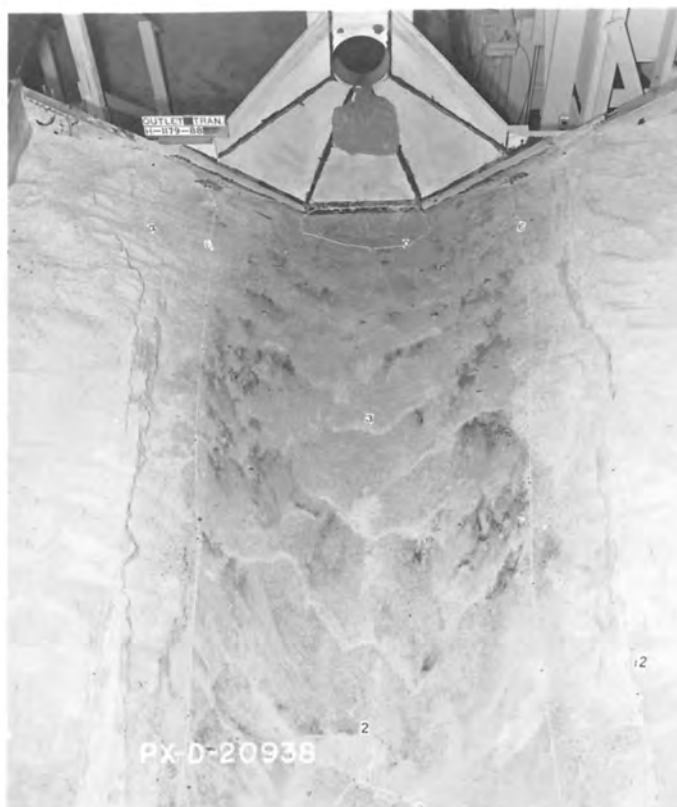
B. Scour after 30 minutes operation each at flow velocities in pipeline of 2, 2.5, and 3 f/s. Depth = 0.8D .
