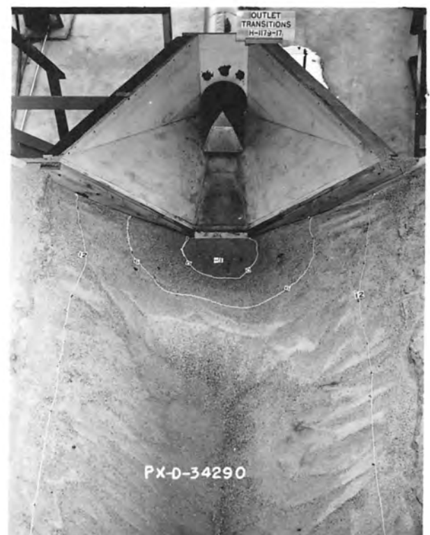
C. Scour 75 minutes operation with hump. Q = 2.4 , V_p = 3.0 , depth = 1.5D .
