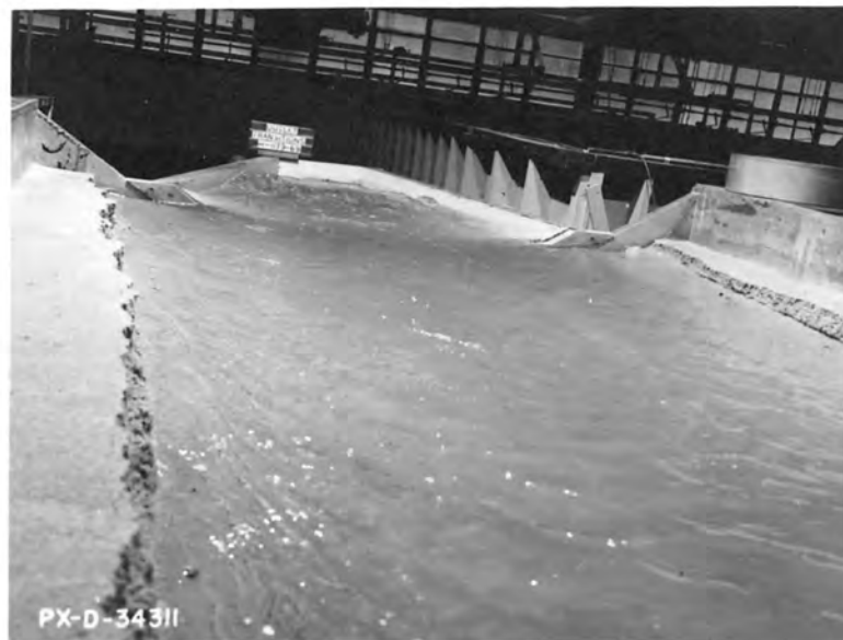
A. A hump occurs in the water surface above the Design 2, hump-like deflector on the floor. Q = 4.7 , V_p = 6.0 , canal depth = 1.3D .
