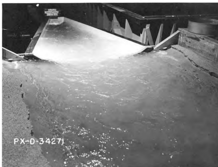
A. The water surface is mildly turbulent. Q = 4.7 cfs, V_p = 6.0 f/s, depth = 1.3D .
