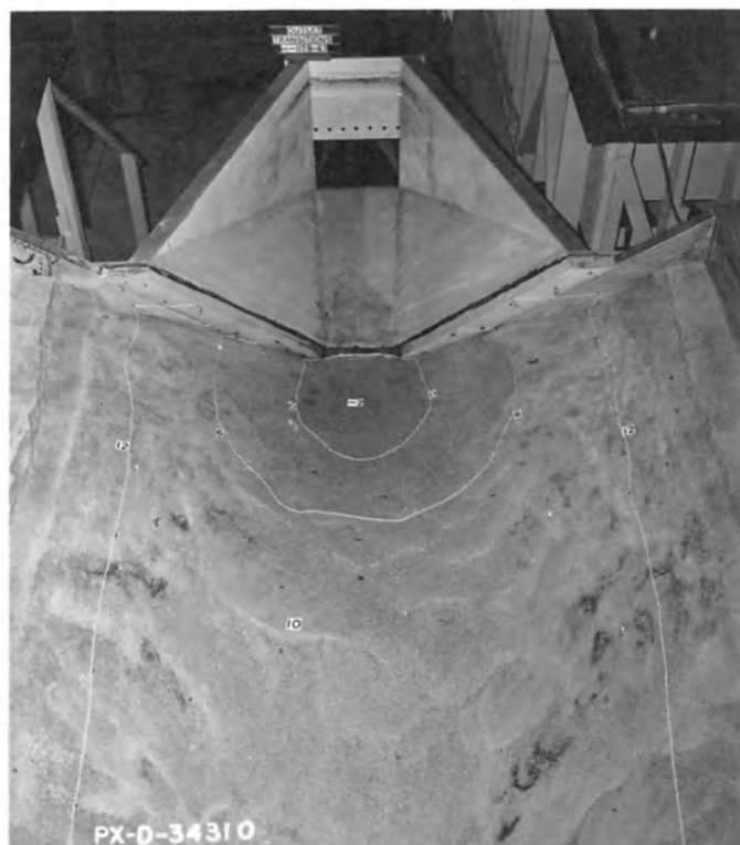
B. Scour after 1 hour operation. Q = 4.7 , V_p = 6.0 , canal depth = 1.3D .
