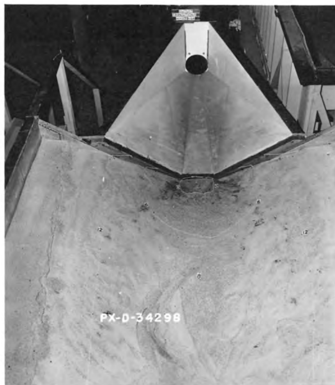
B. Scour after 1 hour operation. Q = 4.7 , V_p = 6.0 , depth = 1.3D .
