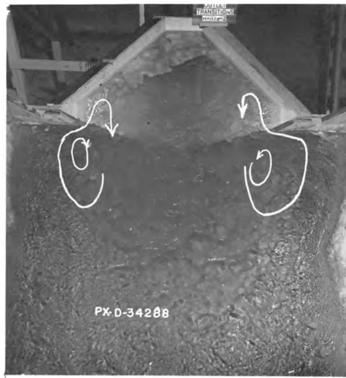
A. Flow is confined mainly to passage center. Eddies occur at sides. Q = 3.0 , V_p = 3.8 , canal depth = 1.5D .
