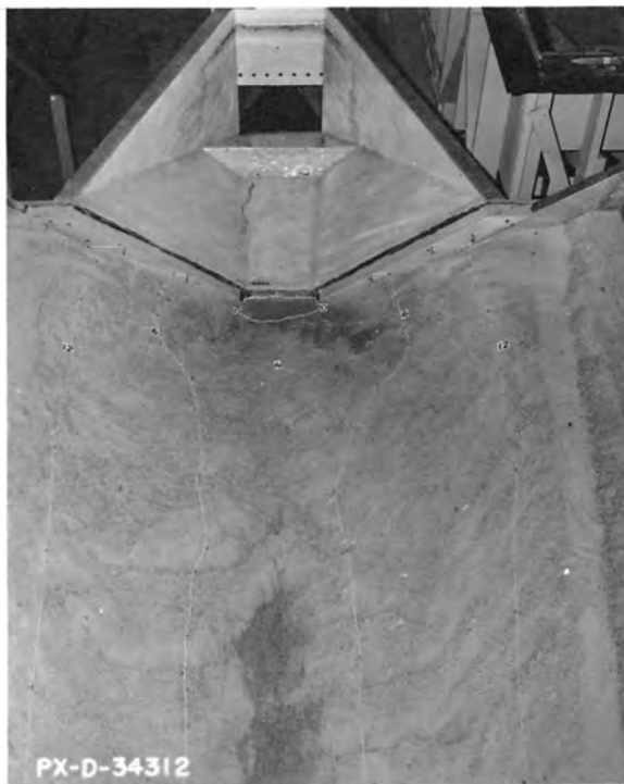
B. Scour after 1 hour operation 6-3/8-inch-high deflector. Q = 4.7 , V_p = 6.0 f/s.
