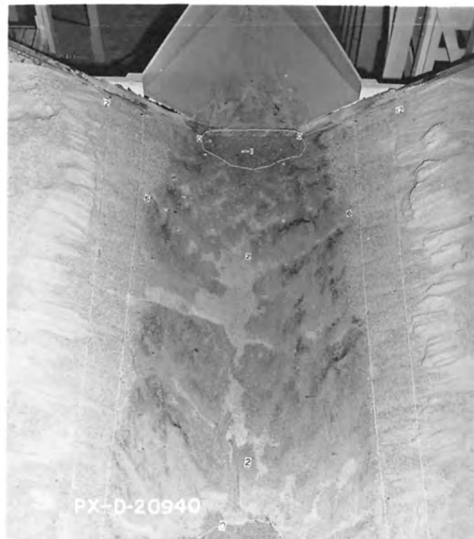
B. Scour after 2-1/2 hours, V_p = 2, 2.5, and 3 \text{ f/s} ; canal depths of 8, 10, and 12 inches. Pipeline on 2:1 slope, depth = 0.8D .
