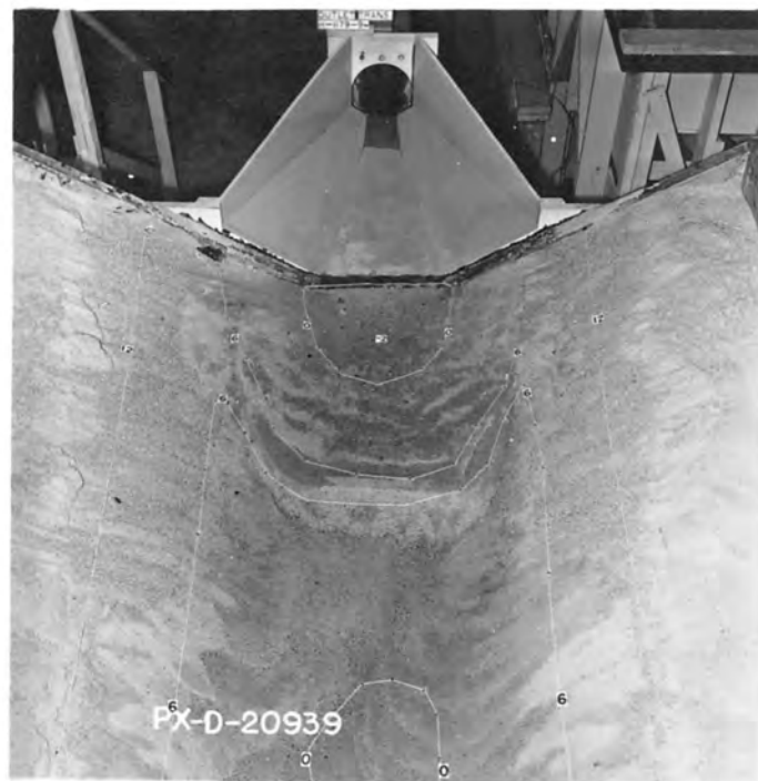
A. Scour after 2-1/2 hours, V_p = 2, 2.5, and 3 \text{ f/s} ; canal depths of 8, 10, and 12 inches. Pipeline horizontal.
