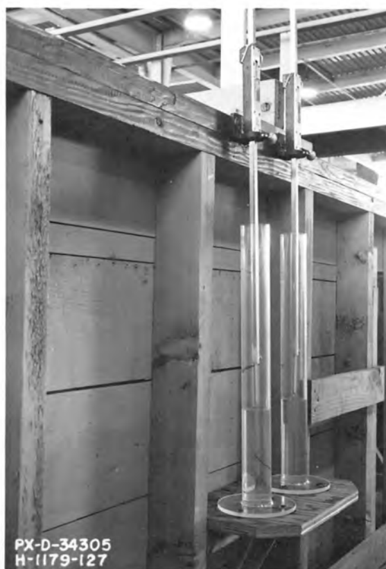
B. Stilling wells and point gages for determining hydraulic grade in 12-inch pipeline.
