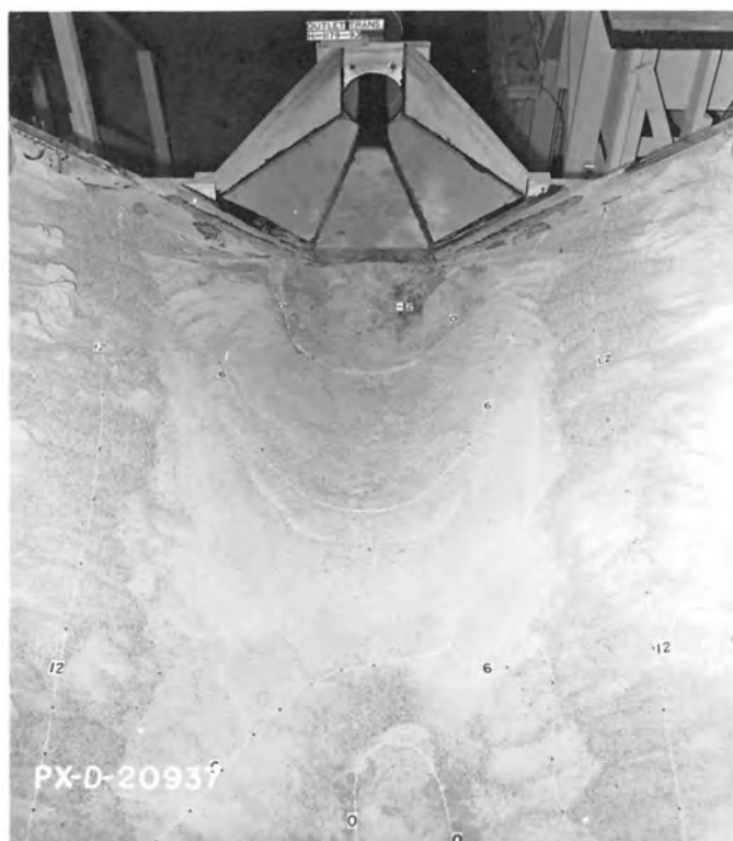
B. Scour after 30 minutes operation each at flow velocities in pipeline of 2, 2.5, and 3 f/s. Depth = 0.8D .
