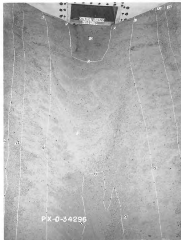
C. Scour after 1 hour operation. Canal depth = 1.25D .
