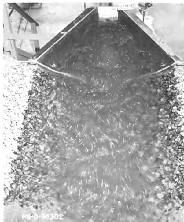
B. Flow conditions. Q = 4.7 , V_p = 6 f/s. Scour occurs at end of riprap.
