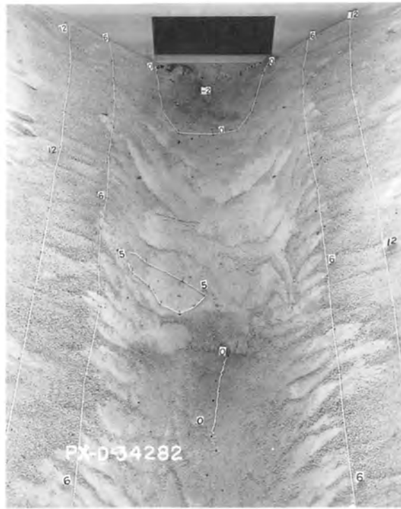
A. Scour after 2 hours operation. Q = 3.1 , V_p = 4.0 , canal depth = 1.0D .
