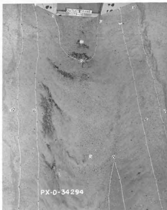
A. Scour after 1 hour operation. Canal depth = 0.83D .
