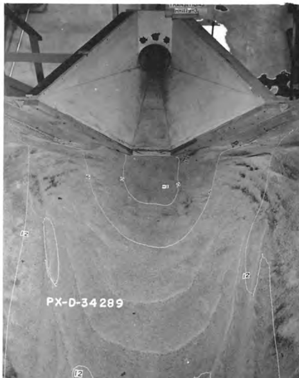
A. Flow is confined mainly to passage center. Eddies occur at sides. Q = 3.0 , V_p = 3.8 , canal depth = 1.5D .
