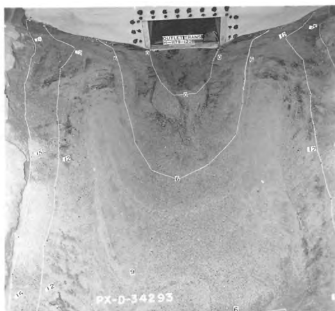
C. Erosion after 1 hour, 1.25D depth.
