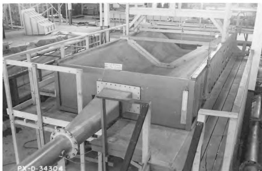
A. Canal model with template in place for shaping sand bed. Closed conduit transition installed with horizontal approach pipe.
