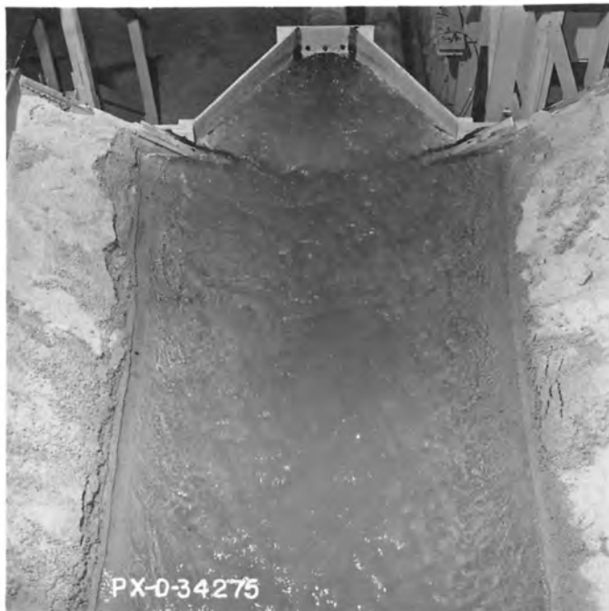
A. Mildly turbulent water surface. Q = 2.4 , V_p = 3.0 , depth = 0.8D .
