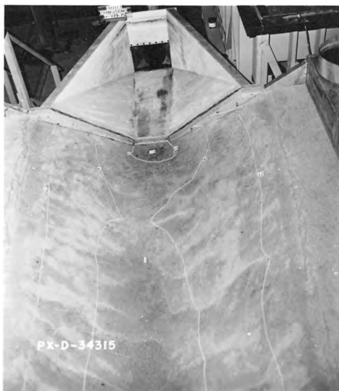
B. Scour after 1 hour. Q = 4.7 , V_p = 6.0 , canal depth = 1.3D .
