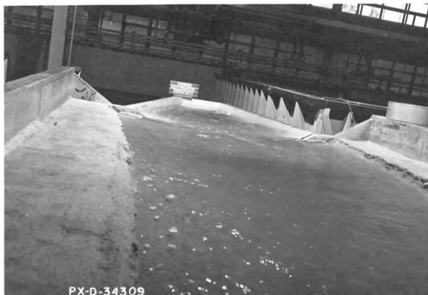
A. Water surface is mildly turbulent in transition, but smooth in canal. Q = 4.7 , V_p = 6.0 , canal depth = 1.3D .
