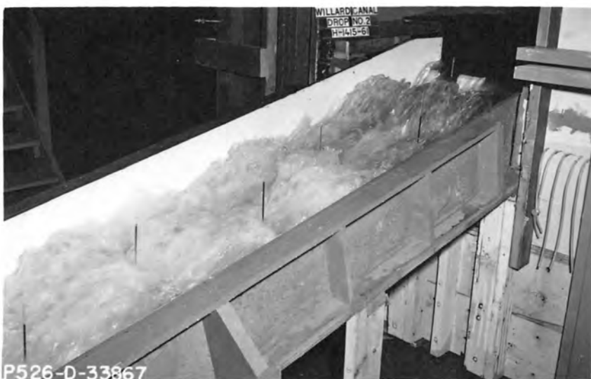
WILLARD PUMPING PLANT NO. 1 BAFFLED APRON DROP NO. 2 Flow Appearance with 13.5-Foot Row Spacing 1:10 scale model
