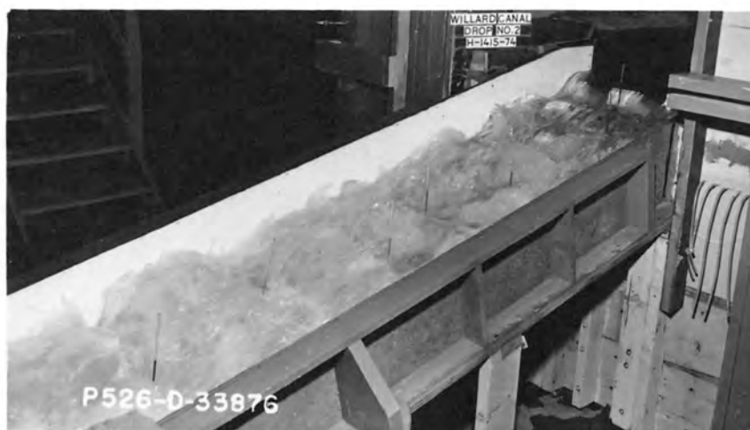
WILLARD PUMPING PLANT NO. 1 BAFFLED APRON DROP NO. 2 Flow Appearance with Second Modification (Rows 1-7 spaced 9 feet apart, 7-12 spaced 13.5 feet apart) 1:10 scale model
