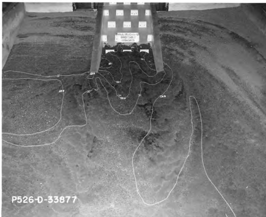
EROSION AFTER 8 HOURS OPERATION AT 950 CFS DISCHARGE
