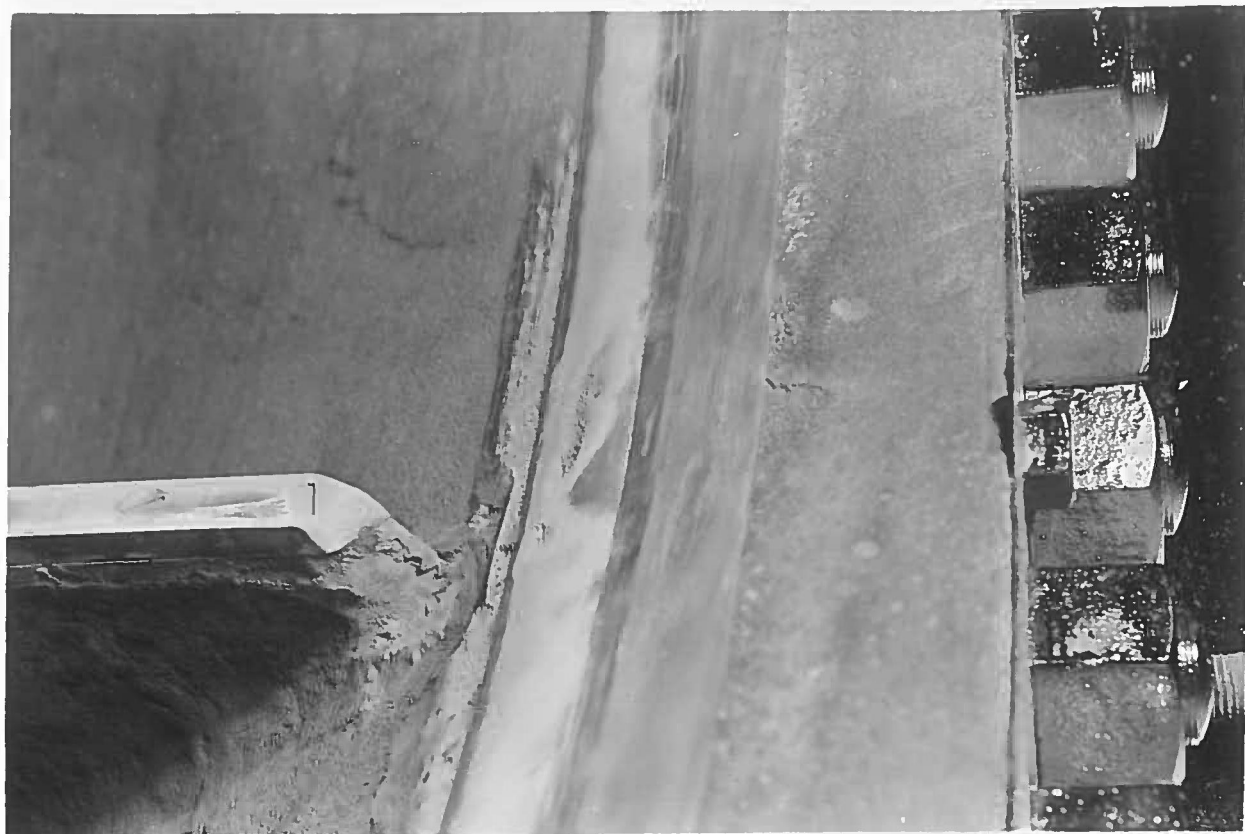
A. CAVITATION AT DOWNSTREAM END OF NEEDLE GUIDE.
