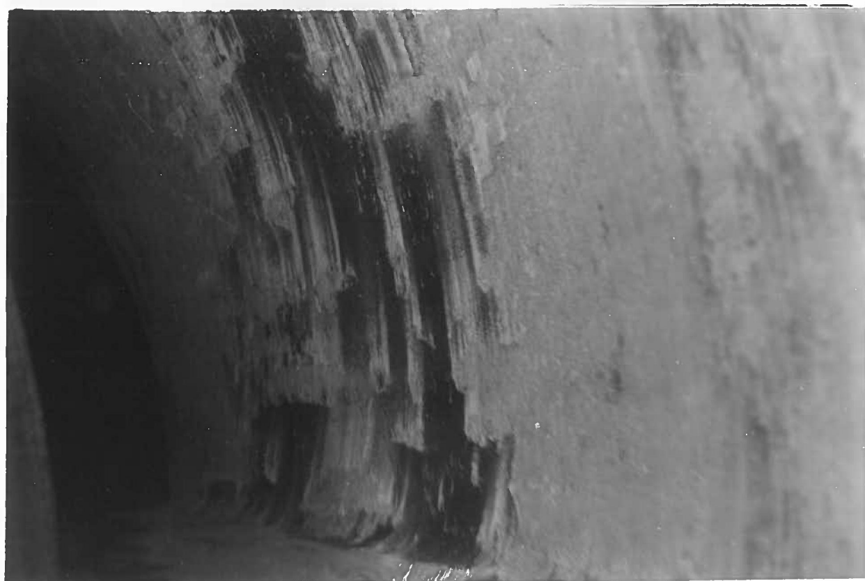
B. FLOW LINES IN RUST ON INSIDE OF NEEDLE VALVE BODY.
