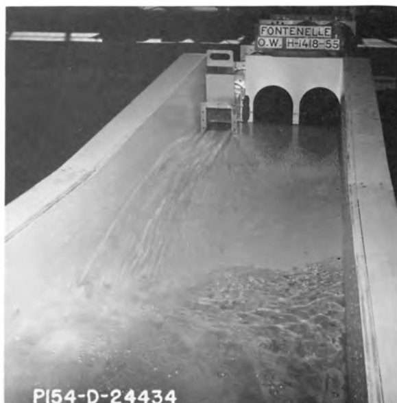
Discharge = 1,200 second-feet Tailwater Elevation = 6401.9
