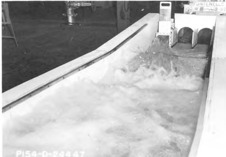
C. Penstock Outlet Horizontal and Turned 3° to the Left (Fourth Modification) Discharge = 4,734 cfs Tailwater Elevation = 6402.3
