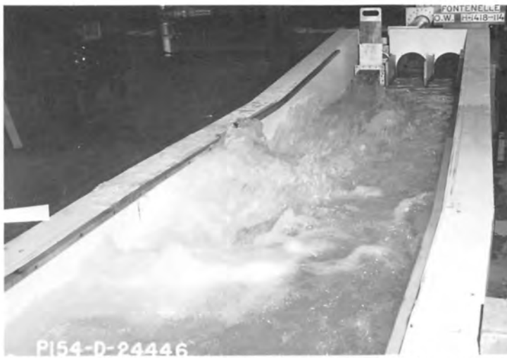
B. Penstock Outlet Horizontal and Turned 2° to the Left (Third Modification) Discharge = 4,734 cfs Tailwater Elevation = 6402.3
