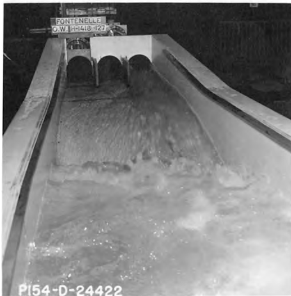
Left tunnel only operating Discharge = 6,233 cfs
