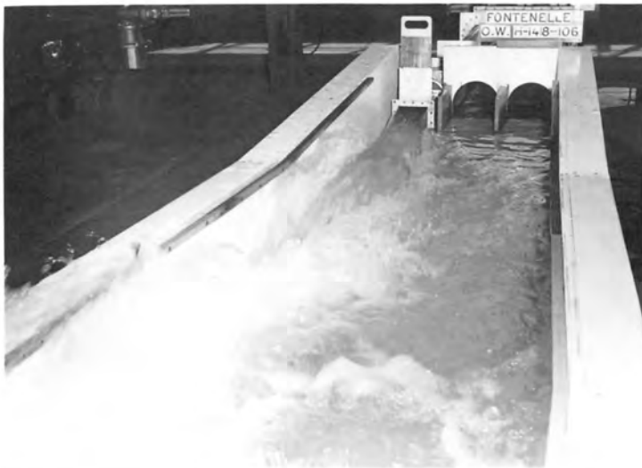
A. Penstock Outlet Horizontal and Pointed Downstream (Second Modification) Discharge = 4,734 cfs Tailwater Elevation = 6402.3
