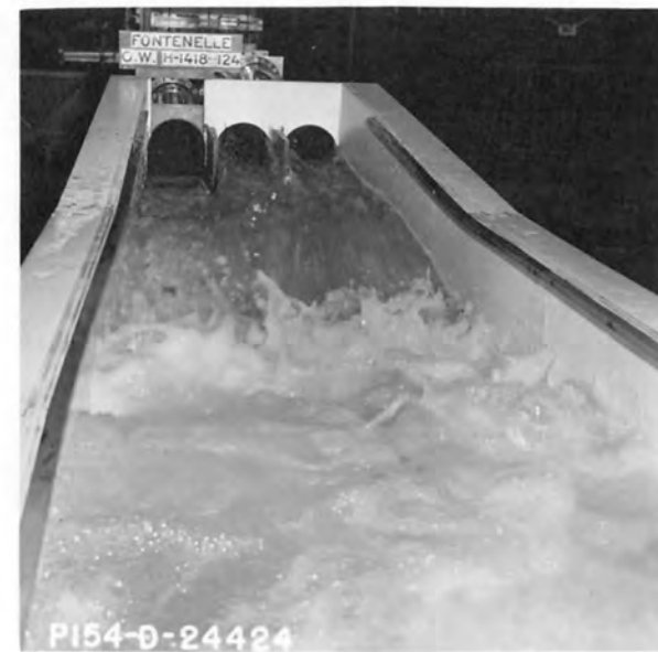
Center and left tunnels operating Discharge = 12,467 cfs
