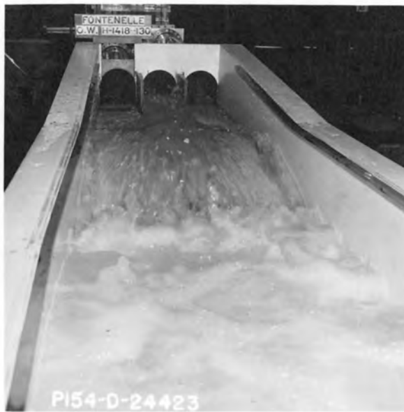
Center tunnel only operating Discharge = 6,233 cfs
