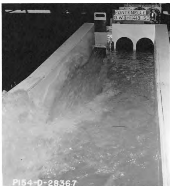
Discharge = 1,200 second-feet Tailwater Elevation = 6401.9
