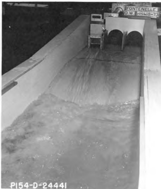
Discharge = 1,200 cfs Tailwater Elevation = 6401.9
