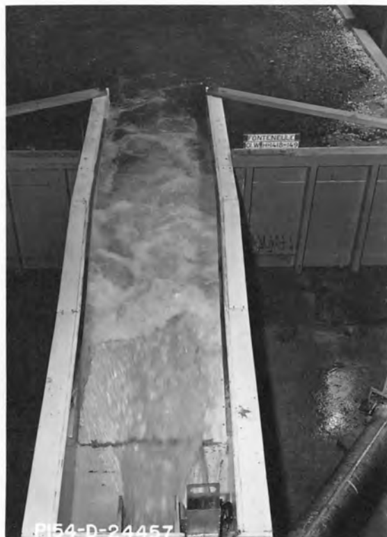
Penstock Outlet Discharge = 2,400 cfs Left Conduit Closed Center Conduit Discharge = 6,233 cfs Tailwater Elevation = 6402.8
