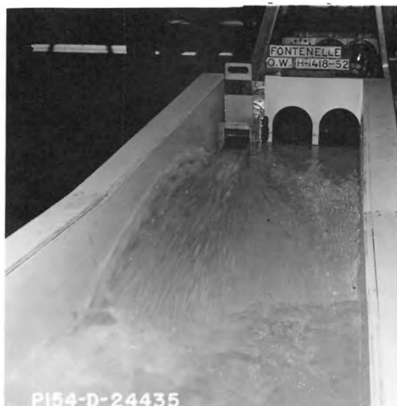
Discharge = 2,400 second-feet Tailwater Elevation = 6402.1
