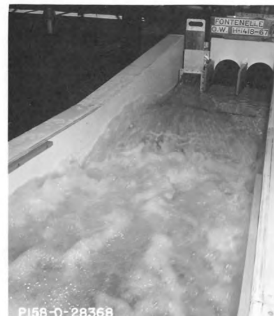
Discharge = 4,734 cfs Tailwater Elevation = 6402.3
