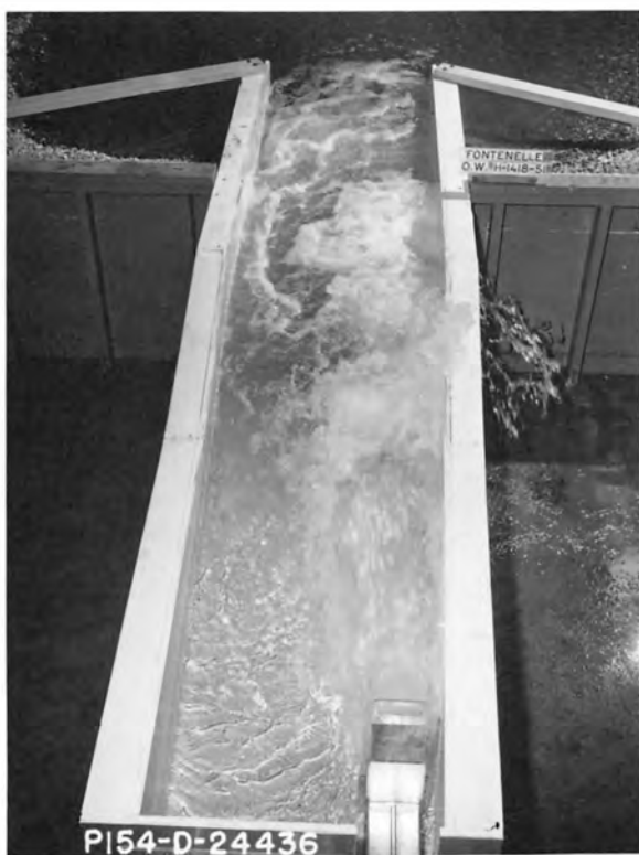
Discharge = 2,400 second-feet Tailwater Elevation = 6402.1
