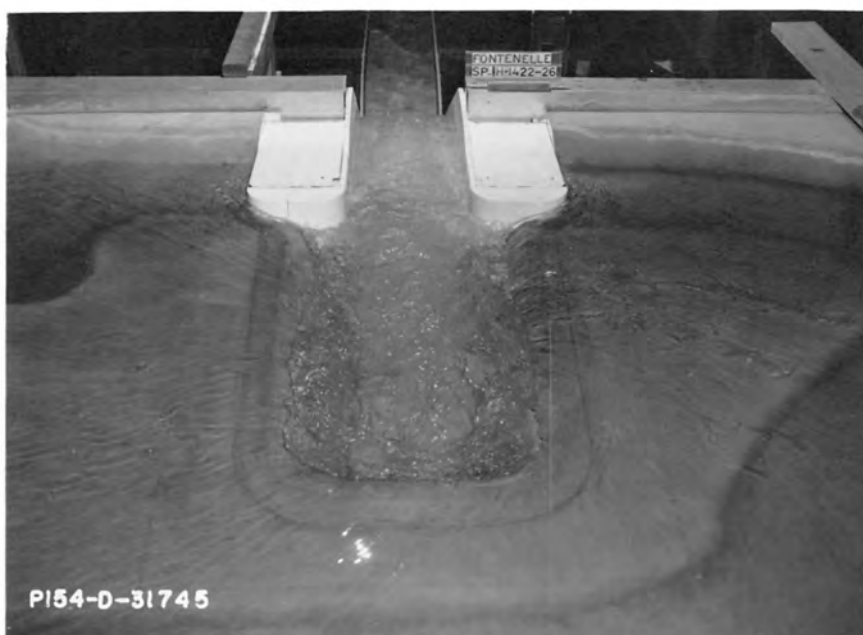
A. 4- by 4-foot Deflector Wall on Basin Floor First Modification
