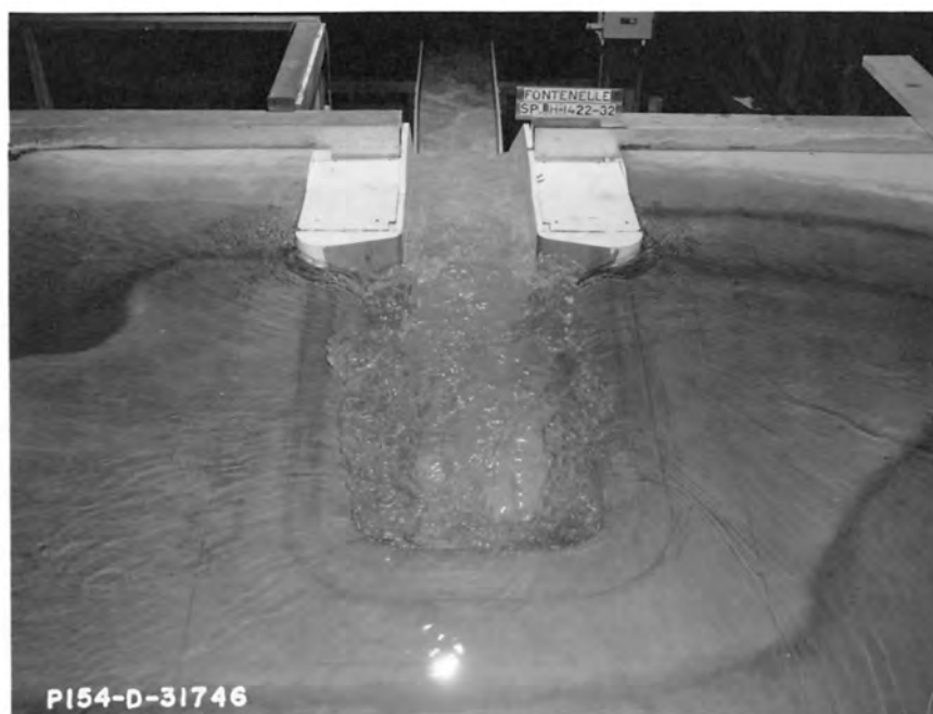
B. Stepped Deflector Wall on Basin Floor 15-foot Radius on Side Piers Second Modification
