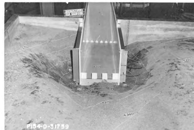
Erosion after 8 hours
