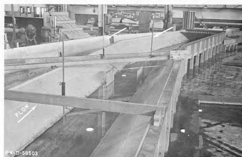
B. Two capacitance probes used for wave height measurements near bridge piers--Point gage for flow depth measurement upstream from piers.
