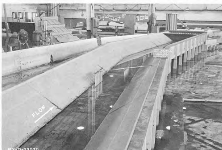
A. Bridge piers in 2-foot bottom width trapezoidal channel, 1.2-foot depth.
