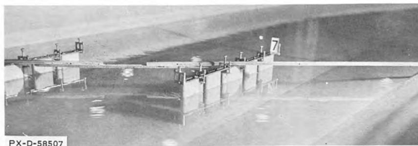
D. Wave action reduced by 15-inch cylinders in spaces.
