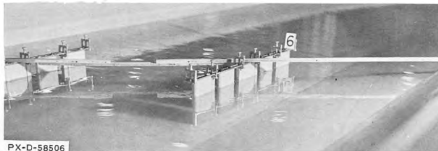
C. Wave action reduced by four, 12- by 12-inch timbers in spaces.
