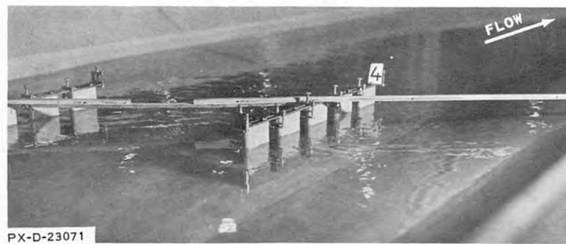
A. Wave action for segmented piers having 32-inch spaces.
