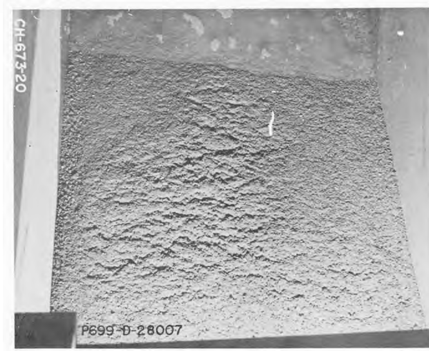
Surface Cracks Forming Just Above Waterline When Drawdown Rate Was 2 ft/hour. Looking Down The Slope East Bench Canal Drawdown Tests 1:1 Scale Sectional Model
