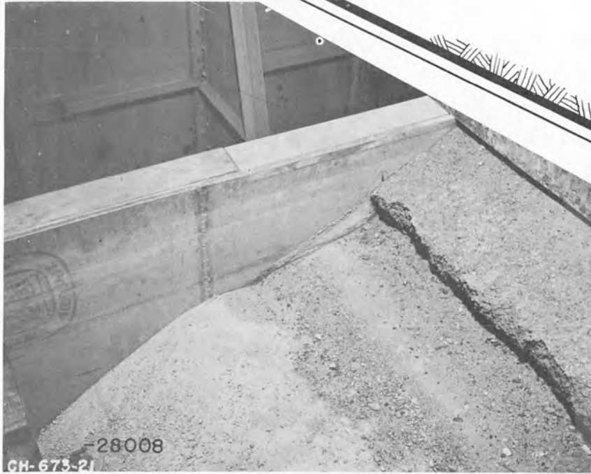
BEACHING EROSION PRODUCED BY SMALL WAVES EAST BENCH CANAL DRAWDOWN TEST 1:1 SCALE SECTIONAL MODEL
