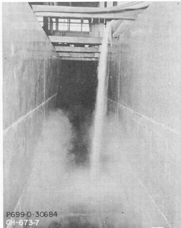
Placing Cover Material Over Asphalt Membrane Material Is Dropped Simulating Placement By Dragline East Bench Canal Drawdown Tests 1:1 Scale Sectional Model
