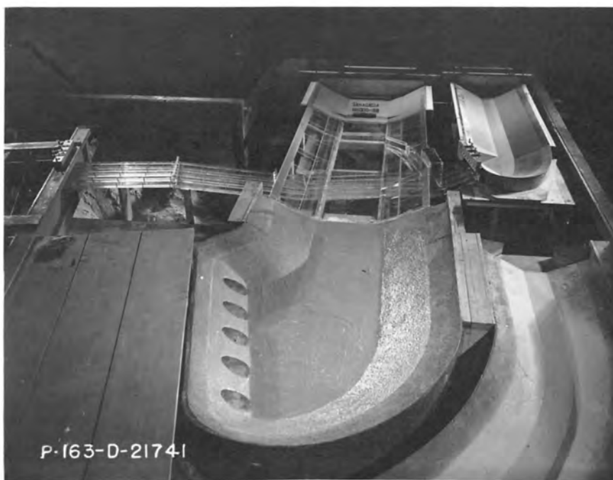
(b) Model Siphon Looking Downstream from Near Low Flow Channel Headworks
