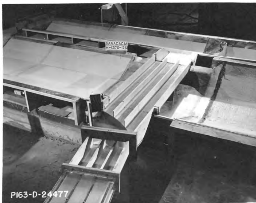
(b) Model Flume Showing Sluice Area from Canal
