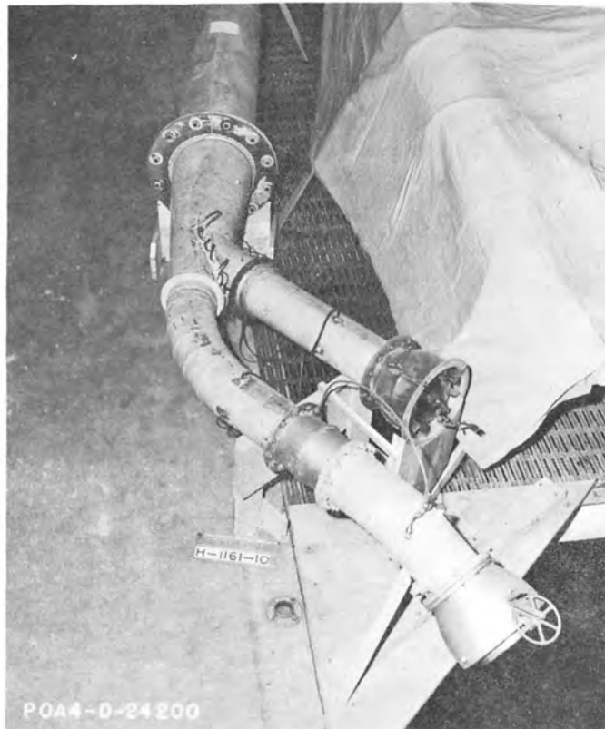
Mexican Outlets Right Outlet Complete Left outlet--Laboratory control valve in position of left butterfly valve Model scale 1:15
