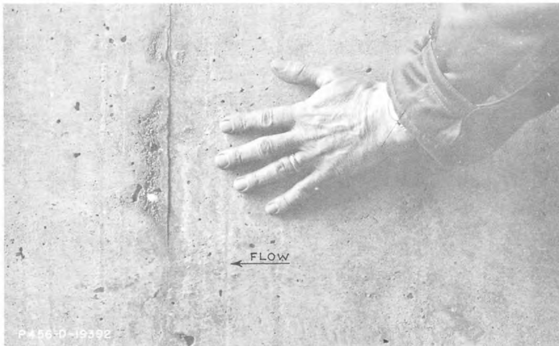
Figure 4--Cavitation-erosion downstream from 1/8 inch into-the-flow offset, atmospheric fluid pressure, and velocity of 100 feet per second--Palisades Dam Outlet Works.
