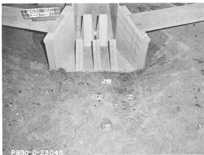
B. Scour after 1/2-hour model operation shown above.
