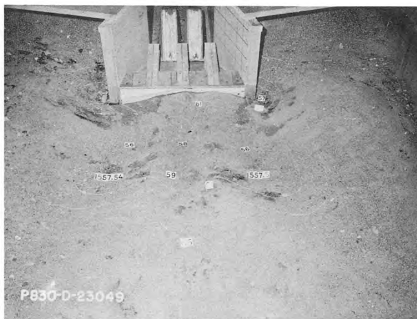
B. Scour after 1/2-hour model operation of Q = 4410 cfs, TW = el 1567
