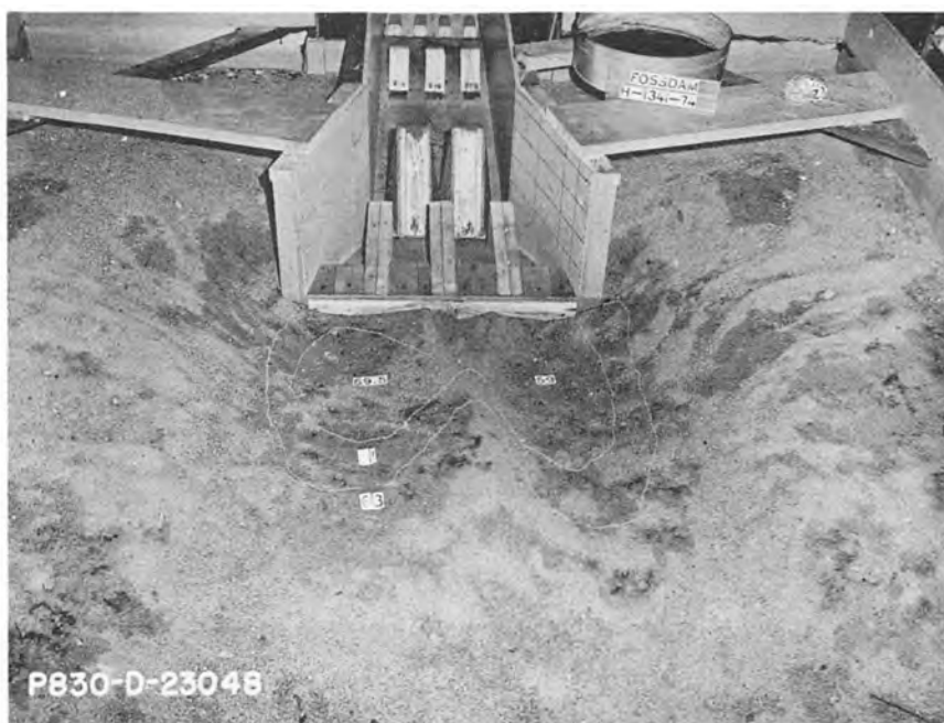
A. Scour after 1/2-hour model operation of Q = 4410 cfs, TW = el 1581.3
