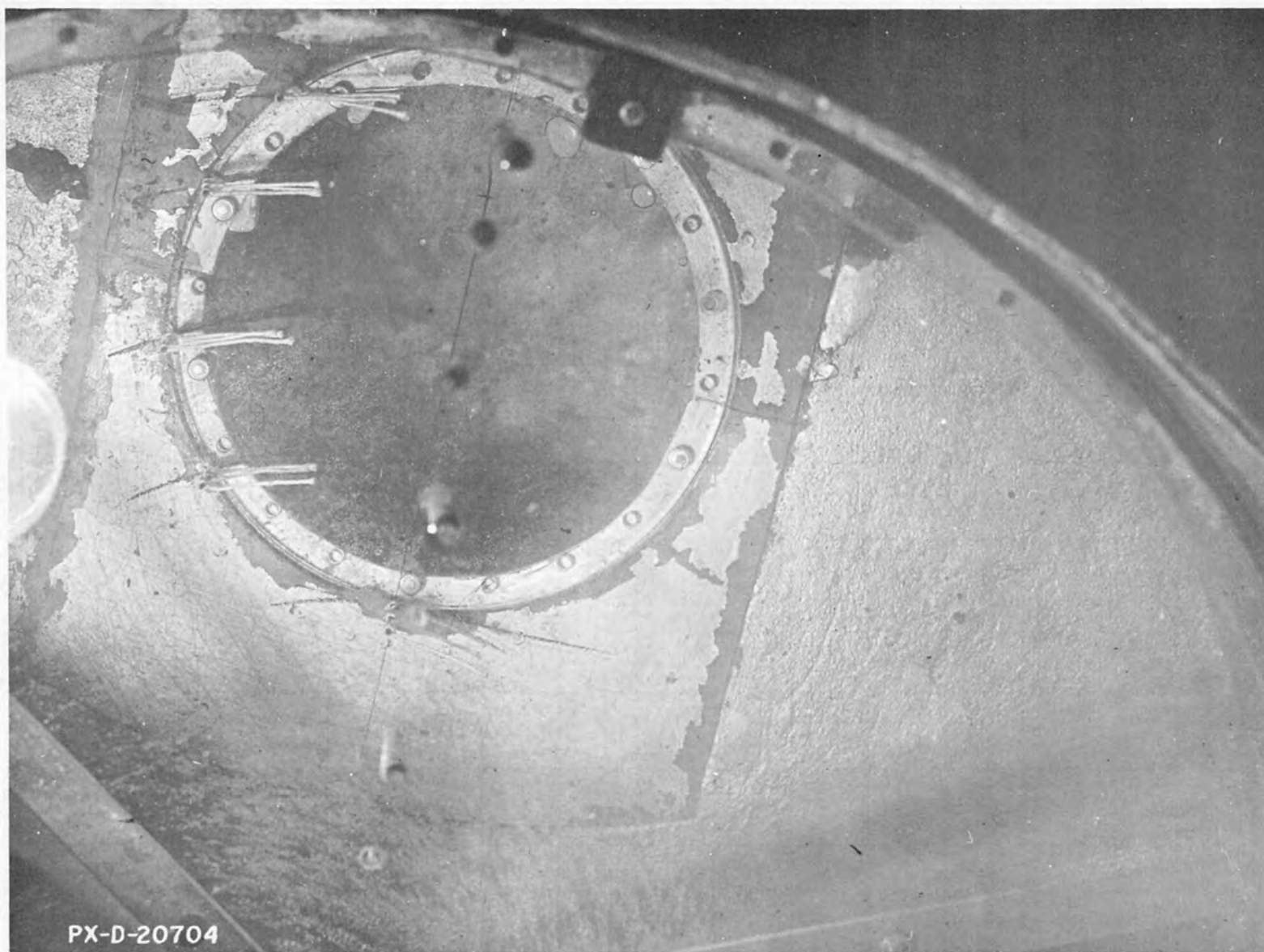
LOWER COST CANAL LINING TRACTIVE FORCE FIELD AND LABORATORY STUDY STRINGS SHOWING DIRECTION OF FLOW ACROSS SAMPLE IN TRACTIVE FORCE TANK - V_r = 24.5 rpm
