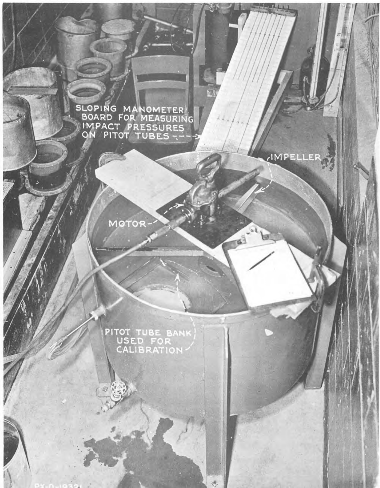
LOWER COST CANAL LINING TRACTIVE FORCE FIELD AND LABORATORY STUDY ARRANGEMENT FOR CALIBRATING TRACTIVE FORCE TANK
