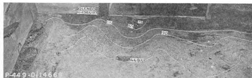
C. Scour pattern in original design after 1-hour operation, at 83% gate opening. Q=10,000 cfs. TW=4505.2'
