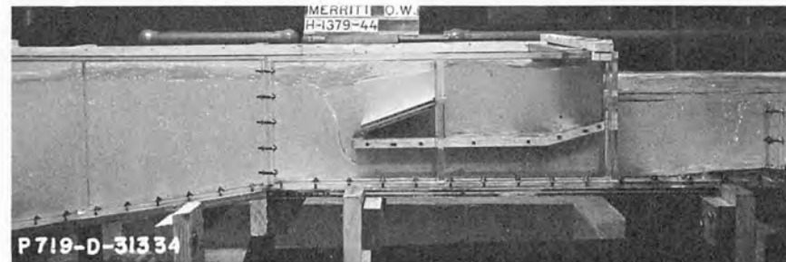
A. 1,340 cfs--Two gates--100 percent open Note the vortex immediately upstream from the wave suppressor.
