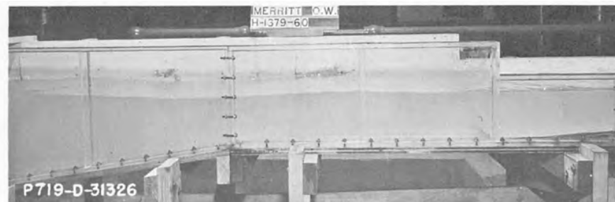
A. Two gates 38 percent open Froude number at Station 17+41.85 = 11.9
