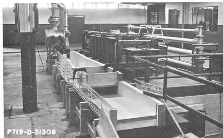
Wave suppressor, held in place with clamps to facilitate removal from model, helps to produce smooth water surface at measuring station downstream.
