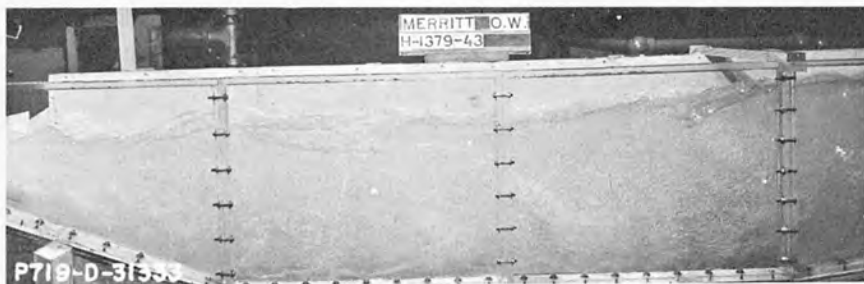
A. 1,340 cfs--Two gates--100 percent open Note the vortex immediately upstream from the wave suppressor.
