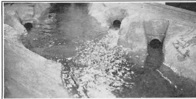
A. Powerhouse 15,000 Second-Feet, Arizona Tunnel Plug Outlet 23,000 Second-Feet, Normal Tailwater
