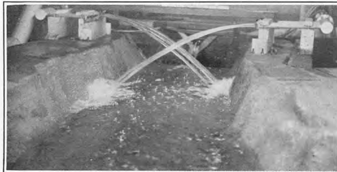
C. Normal Tailwater, Powerhouse 15,000 Second-Feet, Canyon Wall Outlets 21,000 Second-Feet
