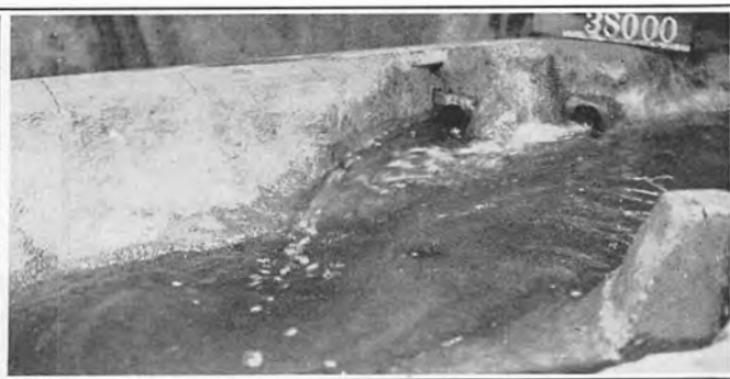
B. Powerhouse 15,000 Second-Feet, Nevada Tunnel Plug Outlet 23,000 Second-Feet, Normal Tailwater
