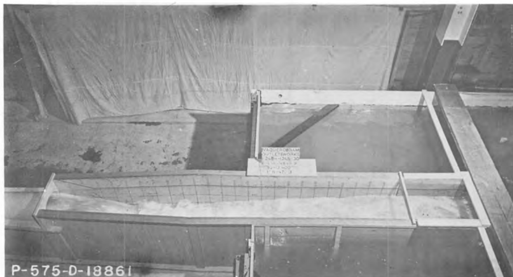
A. Q = 13,400 cfs; T.W. Elev. = 470.3 Both Gates Opened 100%
