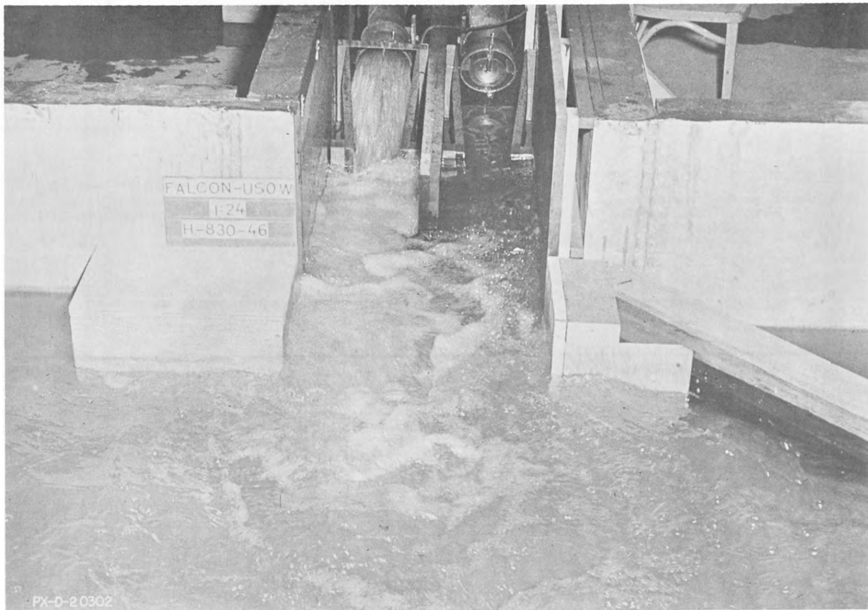
UNITED STATES OUTLET WORKS - FALCON DAM 72-INCH RIGHT VALVE DISCHARGING 100 PERCENT OPEN 1600 CFS - RES. ELEV. 310 APPROX. - T. W. ELEV. 180.5 1:24 SCALE MODEL
