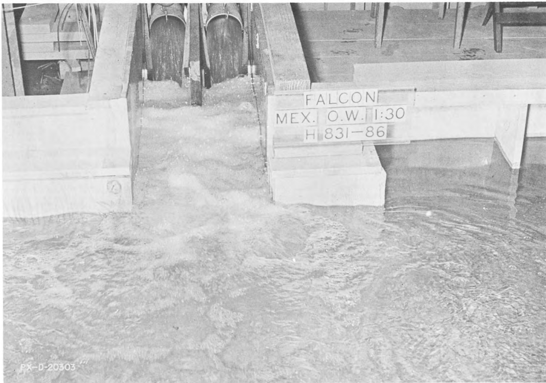
MEXICAN OUTLET WORKS - FALCON DAM 90-INCH VALVES 100 PERCENT OPEN 4,570 CFS - RES. ELEV. 300 APPROX. - T. W. ELEV. 181.2 1:30 SCALE MODEL
