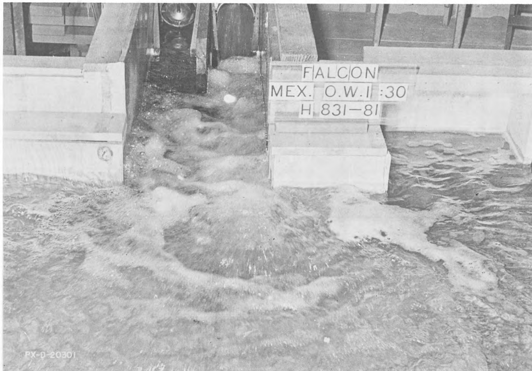
MEXICAN OUTLET WORKS - FALCON DAM 90-INCH LEFT VALVE DISCHARGING 100 PERCENT OPEN 2,400 CFS - RES. ELEV. 300 APPROX. - T. W. ELEV. 181.2 1:30 SCALE MODEL
