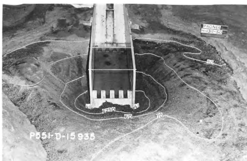
PAONIA DAM SPILLWAY PERFORMANCE OF PRELIMINARY STILLING BASIN 1:36 SCALE MODEL
