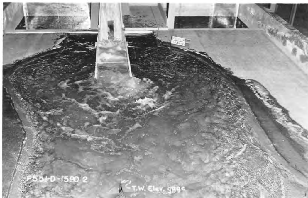
PAONIA DAM SPILLWAY PRELIMINARY SPILLWAY--12,600 CFS 1:36 SCALE MODEL
