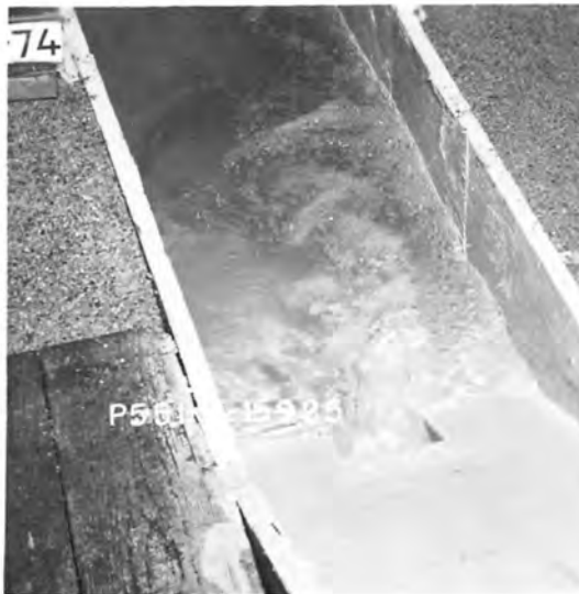
A. Outlet works discharge 700 cfs. Note: The flow veers to either the right or the left. No spillway discharge.
