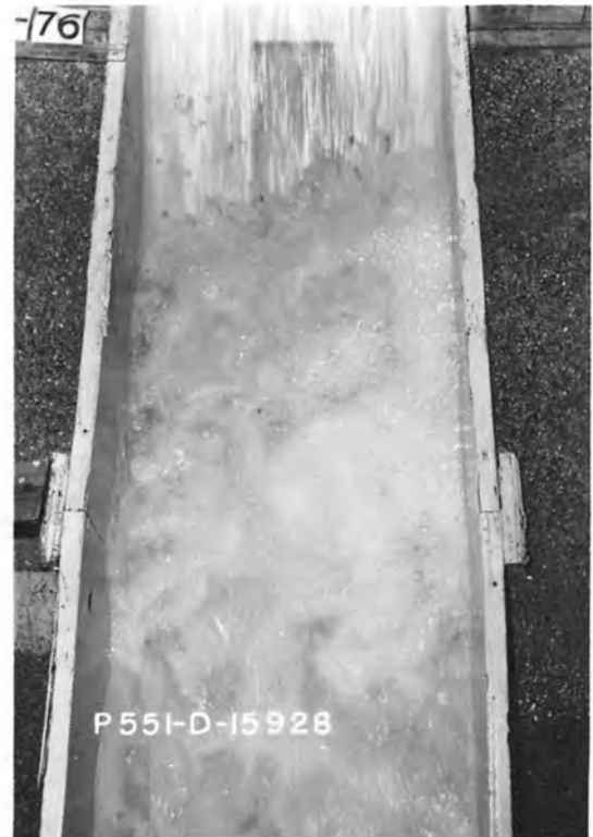
C. Spillway discharge 12,600 cfs
