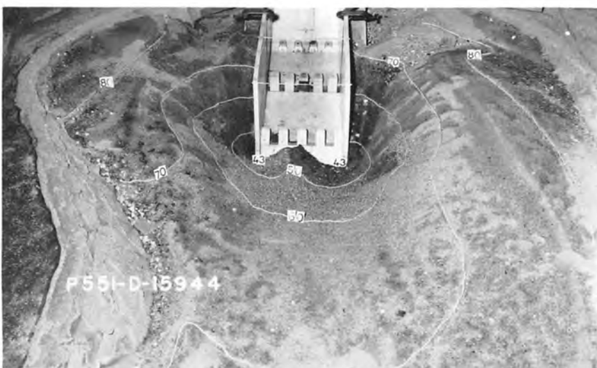
PAONIA DAM SPILLWAY PERFORMANCE OF RECOMMENDED STILLING BASIN DISCHARGING 12,600 CFS 1:36 SCALE MODEL
