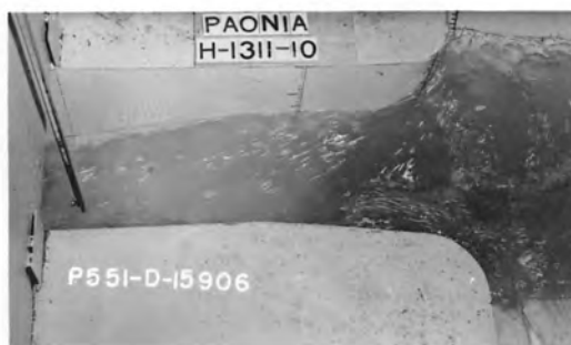
C. Flow from the basin into the chute.
