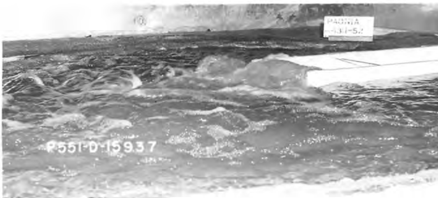
Note boil has moved upstream. Compare with Figure 26.
