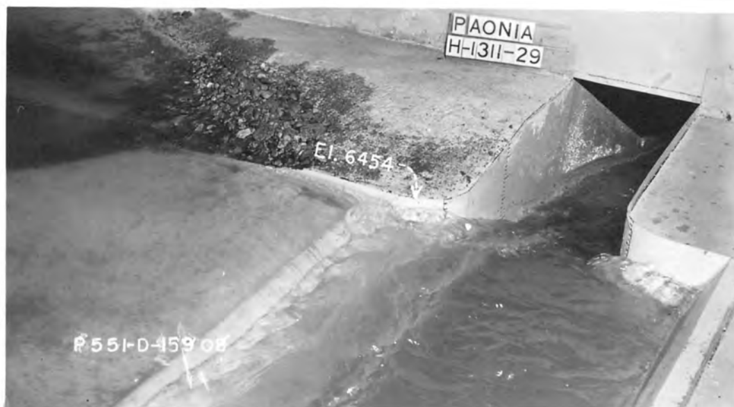
B. Rock fill was effective in reducing turbulence near left wall but flow fluctuations sometimes overtopped the wall.
