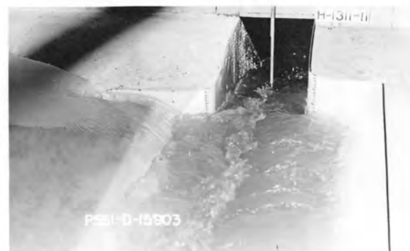
B. Turbulence occurs at left approach wall.
