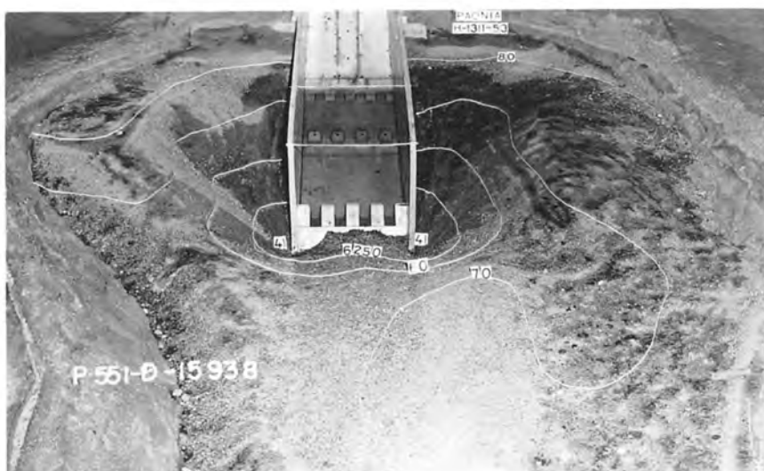
Erosion after one hour model test run.
