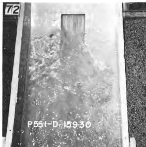
B. Outlet works discharge 1,200 cfs No spillway discharge Note: Flow veers to the left.
