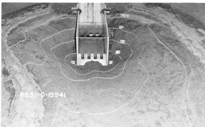
PAONIA DAM SPILLWAY PERFORMANCE OF STILLING BASIN MODIFICATION NO. 2 1:36 SCALE MODEL
