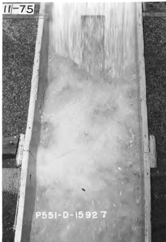
B. Spillway discharge 10,200 cfs Outlet works discharge 1,400 cfs
