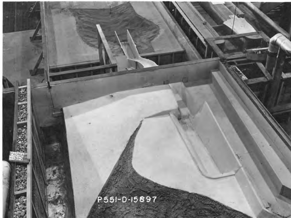
A. Side channel spillway entrance. Note step up from side channel basin floor to chute floor.
