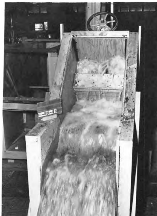
A. 10 cfs flow at 80 fps with 100 foot head
