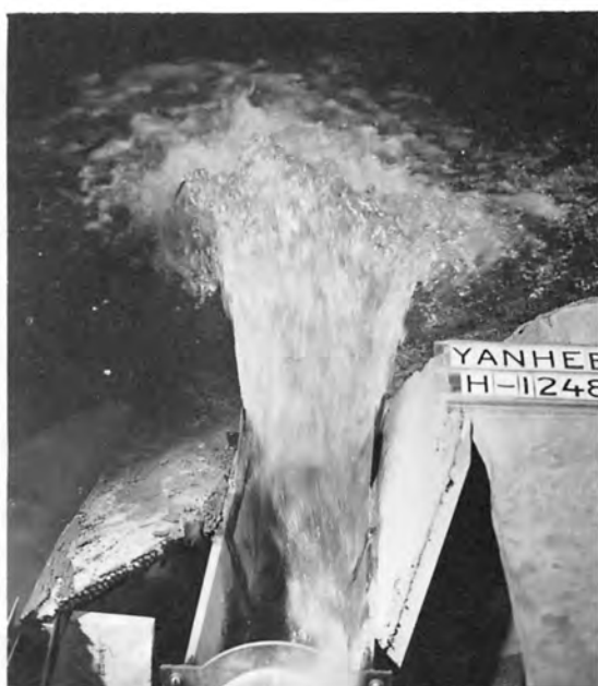
A. Extreme right gate open - other gates closed.
