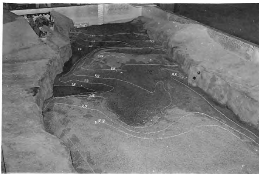
B. Recommended bucket design. Sand elevation before test was 128 m.
