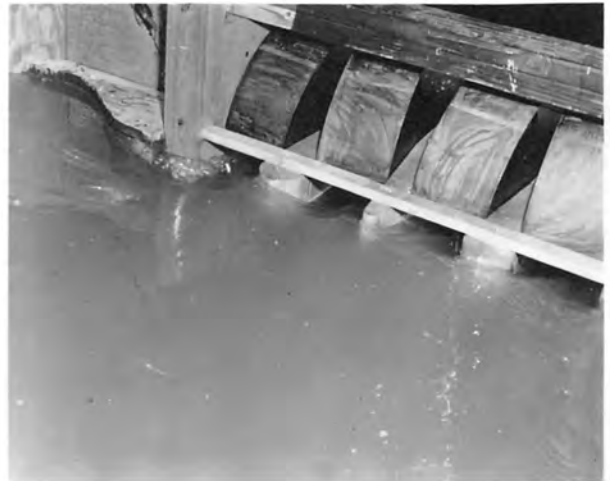
C. Flow disturbance at left pier.
