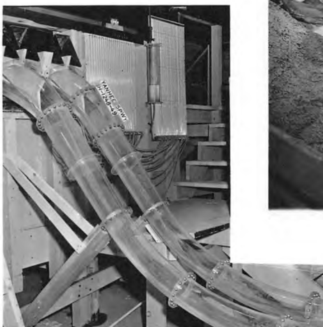
C. Flow in spillway tunnels.
