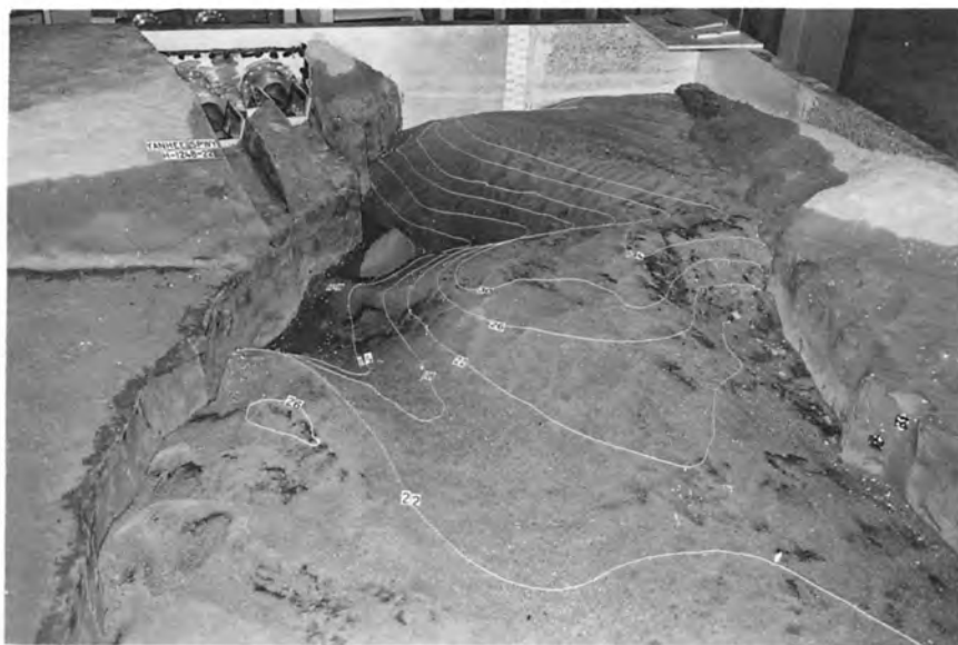
A. Preliminary bucket design. Sand elevation before test was 136 m.
