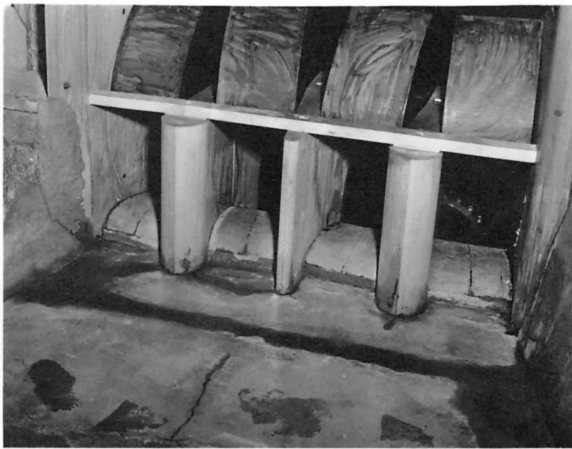
A. Modified left pier nose and flow disturbance - Design A.
