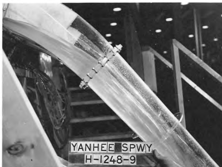
B. Discharge = 2000 CMS. Gates partially closed at maximum reservoir elevation.
