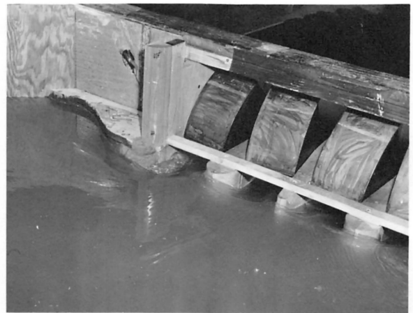
A. Modified left pier nose and flow disturbance - Design A.
