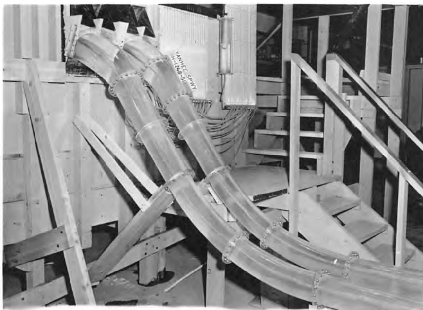
A. Flow through tunnels. Recommended transition in left tunnel and preliminary transition in right tunnel.
