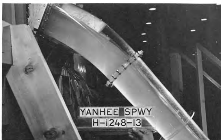
A. Maximum discharge = 6000 CMS. Note hump in water surface at downstream end of transition.
