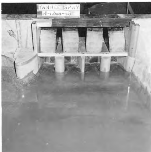
A. Flow entering spillway.
