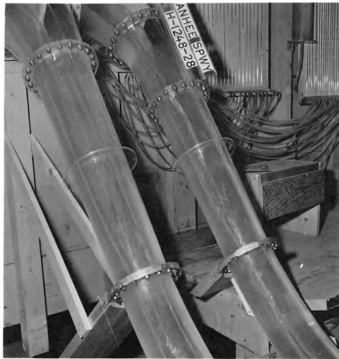
A. Recommended transition in left tunnel and preliminary transition in right tunnel. Note absence of fin of water in right tunnel.
