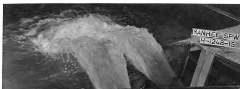
C. Note right jet striking 1/4:1 slope.
