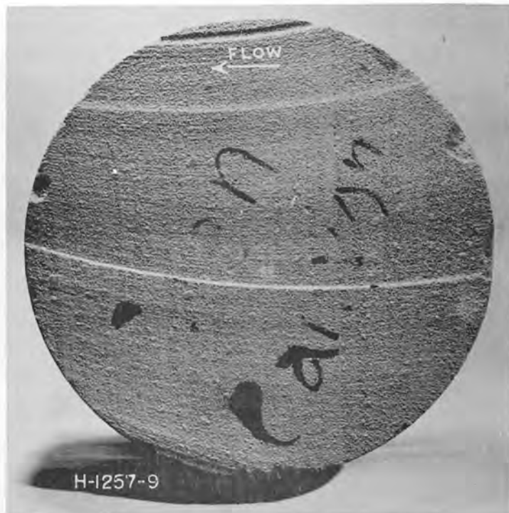
B. Erosion after 4 hrs. at 20 fps, 25½ hrs. at 40 fps, 16 hrs. at 58 fps, and 7½ hrs. at 72 fps with flow parallel to surface.
