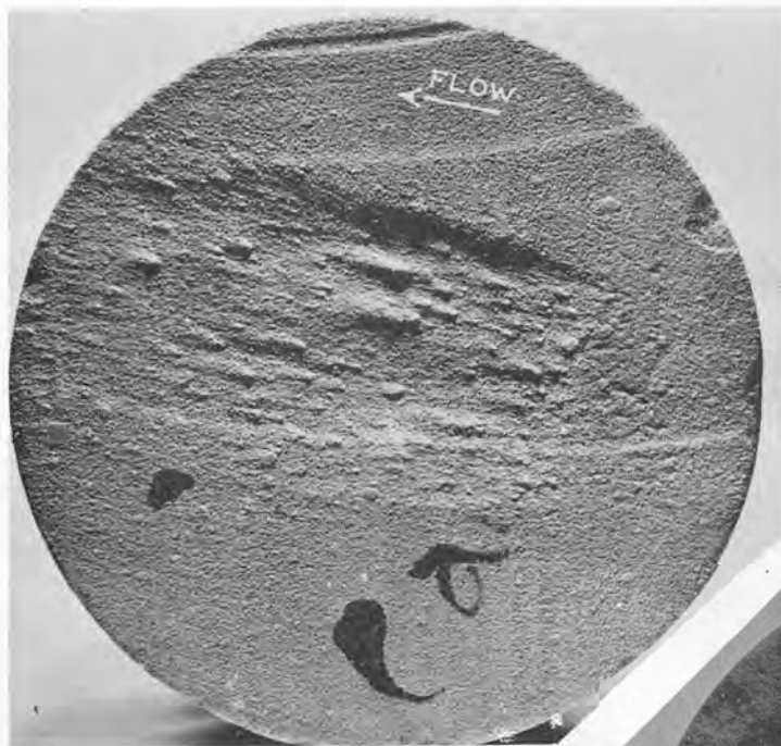
A. 4 hour test at 20 fps removed 5.2cc of sandstone. Sediment concentration - 214 ppm.
