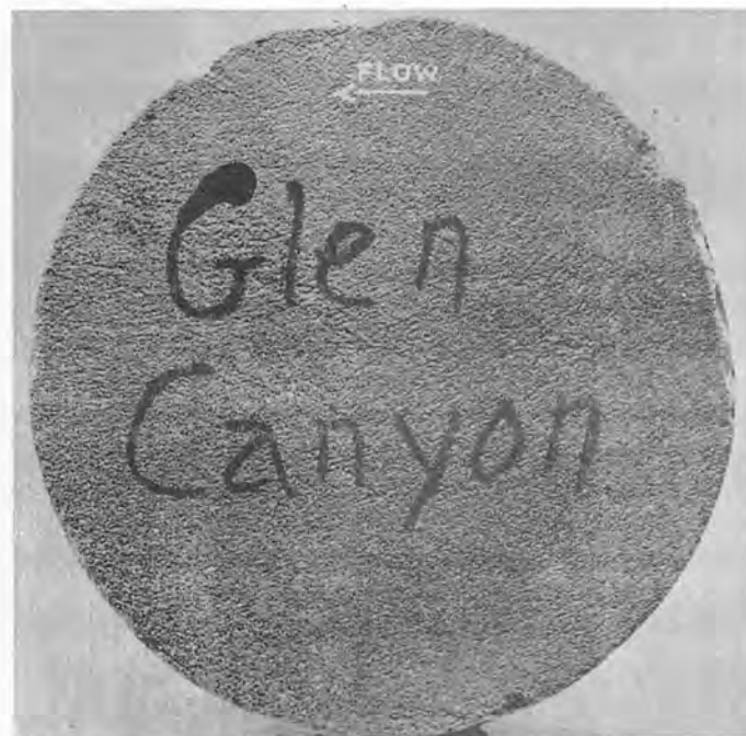
C. Erosion after above test plus 24 hours at 72 fps with flow impinging at 25^{\circ} .
