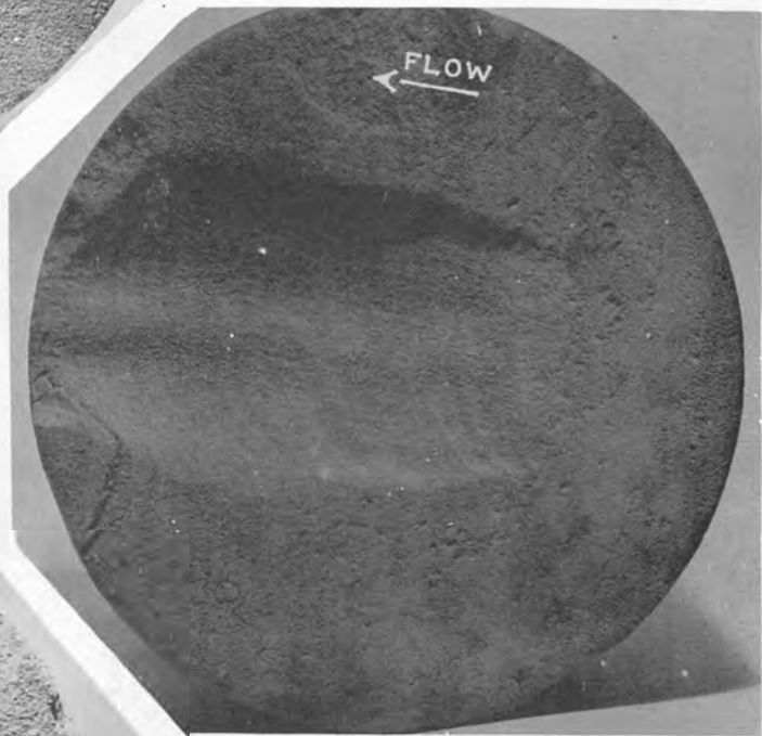
B. 4 hour test at 30 fps removed 38.1cc of sandstone Sediment concentration - 911 ppm.
