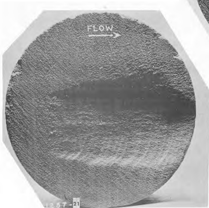
C. 4 hour test at 40 fps removed 25.5cc of sandstone Sediment concentration-2,370 ppm.
