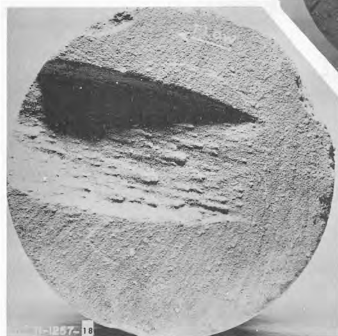
C. 4 hour test at 40 fps removed 52.5 cc of sandstone Sediment concentration - 632 ppm. GLEN CANYON SANDSTONE EROSION STUDIES
