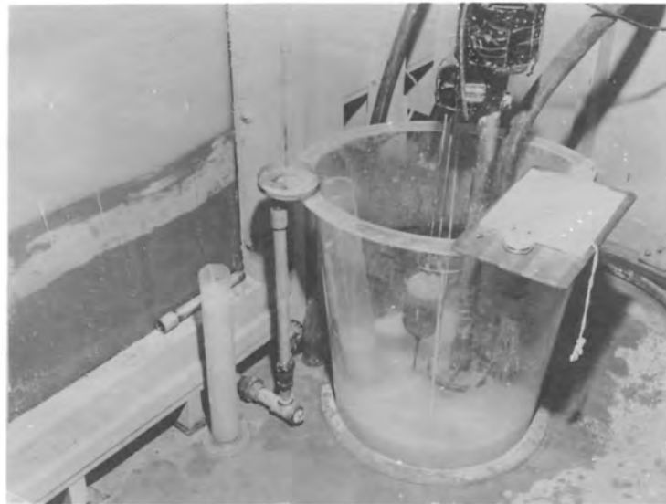
Seepage outlet from soil compartment with overflow into plastic tank
