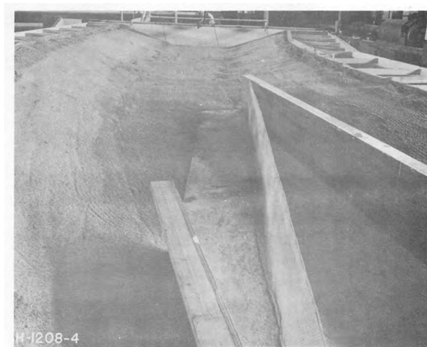
(B) Sand movement in downstream channel following test at discharge representing 4860 cfs, W. S. Elev. +2.0.
