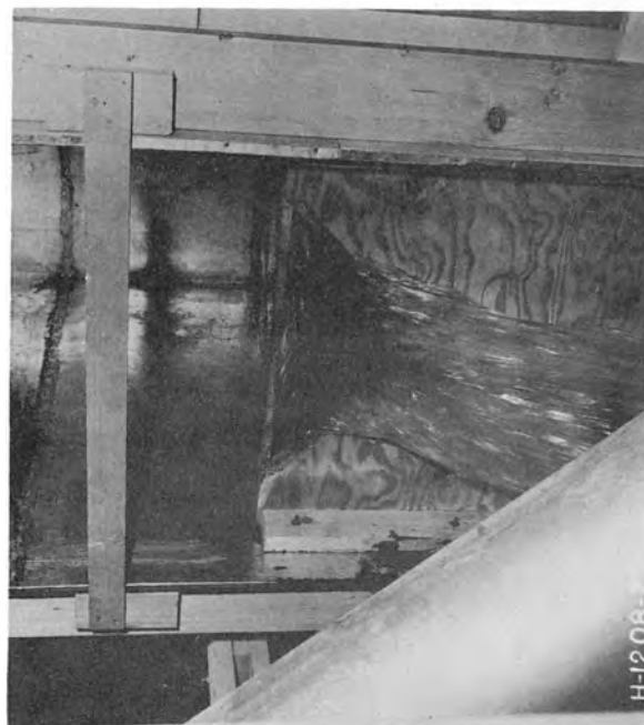
(C) 90° V-notch weir in tailbox for measurement of discharge through bypass
