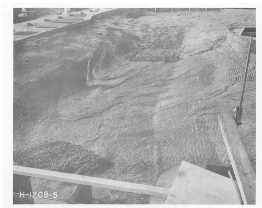
(A) Sand movement in upstream channel following test at discharge representing 4860 cfs, W. S. Elev. +2.0, for a time of approximately 2 hours.
