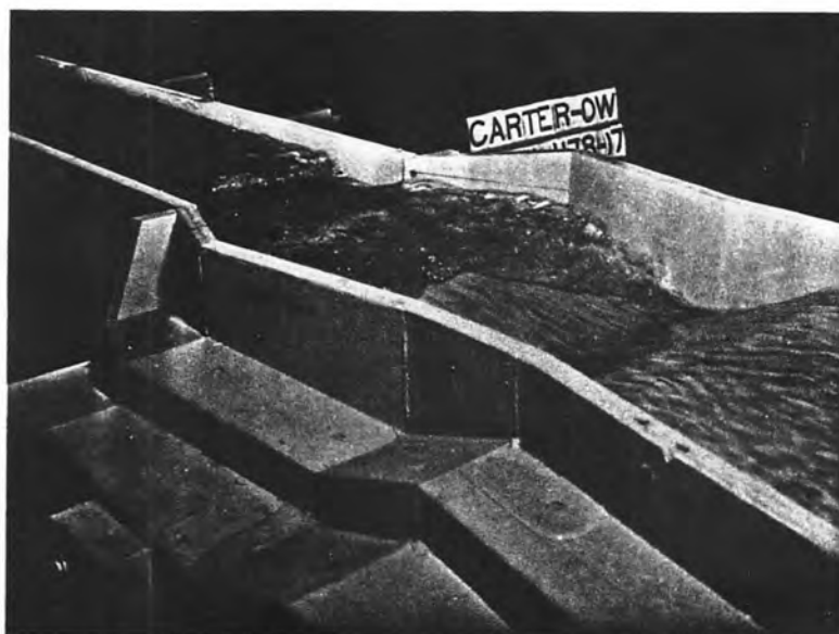
Sill, one-foot square in cross-section, at entrance to rectangular flume reduces wave heights downstream from Parshall flume
