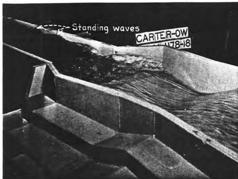
Waves occur downstream from Parshall flume without sill
