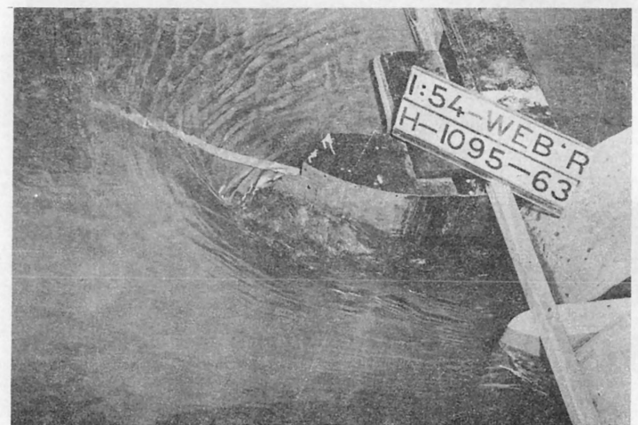
D. Design 4--136,000 second-feet. Note disturbance but not excessive drawdown
