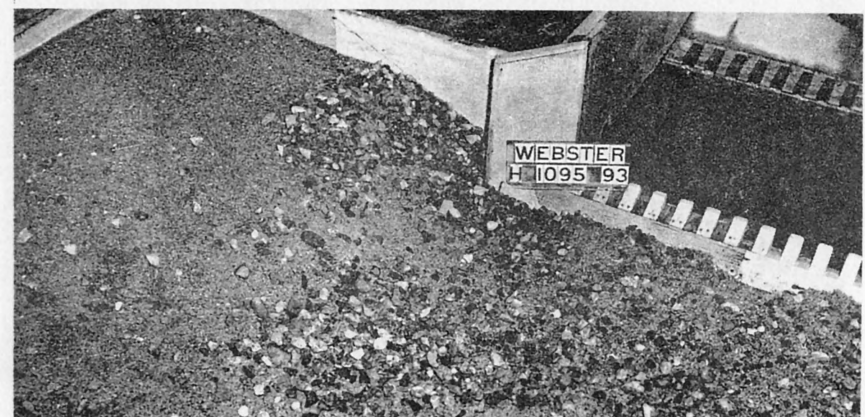
D. Test in (C) continued 4 more hours with maximum discharge. Note right bank riprap failed
