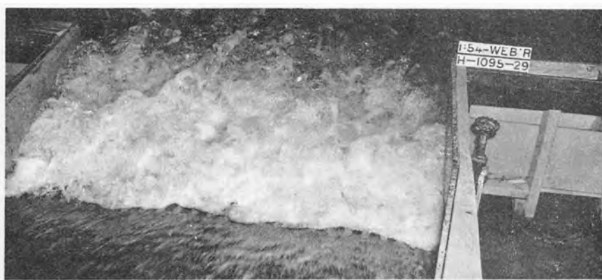
B. Preliminary basin-tail water elev. 4 feet below normal
