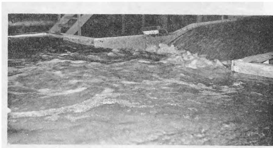
A. Erosion test in progress, normal tail water water elevation. Discharge 136,000 second-feet
