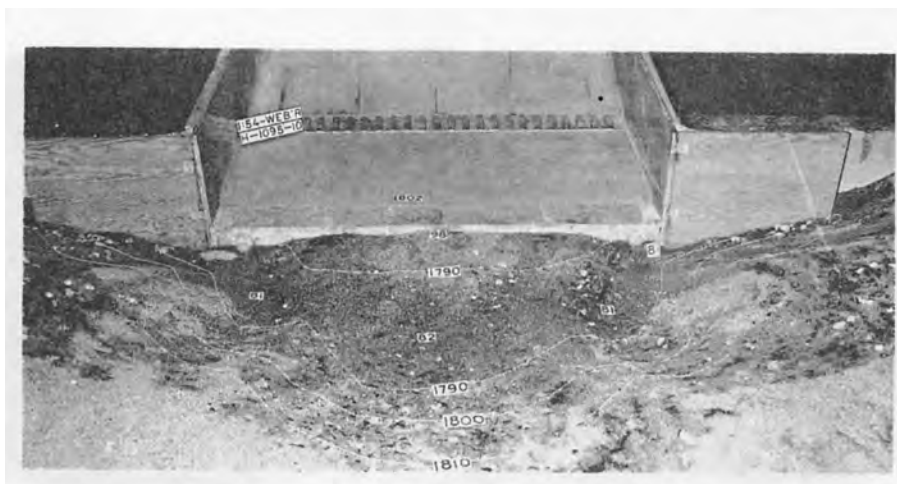
B. Scour pattern after 30 minute model erosion test
