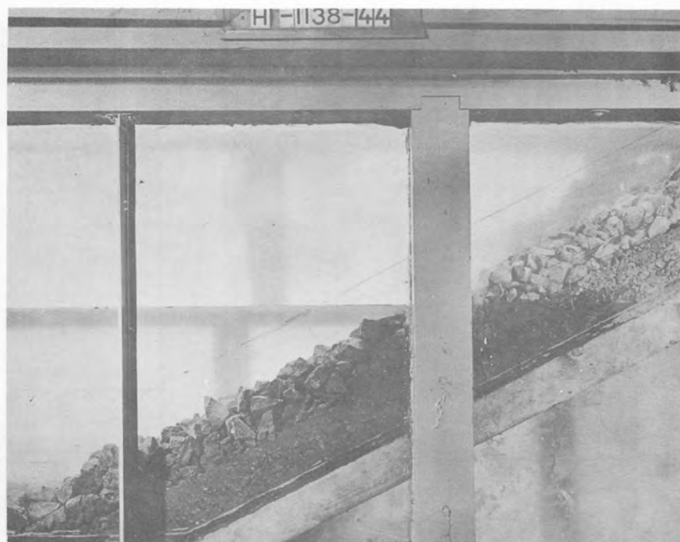
(b) Test 9--Prepared for operation-- Recommended cover - talus separated on 3/4-inch screen
