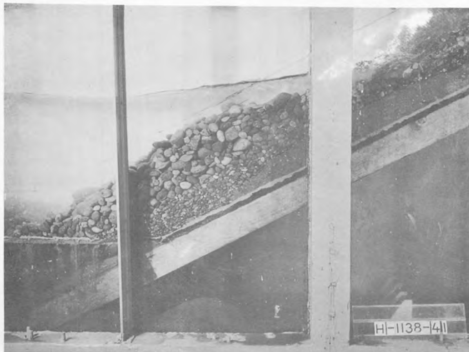
(a) Test 6--After 23 hours of operation 2.7 ft. depth--42 waves per minute-- wave height 0.43 ft.
