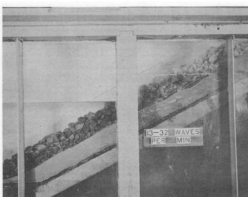
(a) Test 12--after 1 hour of operation at 2.7 ft. depth--32 waves per minute--wave height 0.26 ft.
