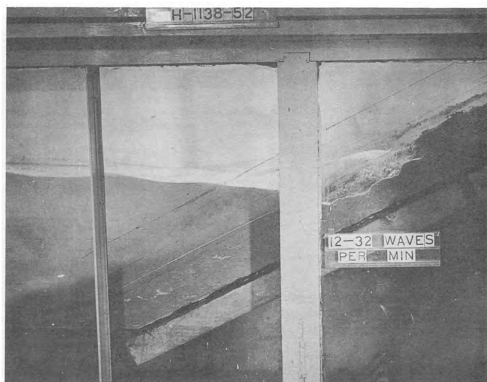
(b) Two minutes after operation started at 2.7 ft. depth and 32 waves per minute--wave height 0.26 ft.
