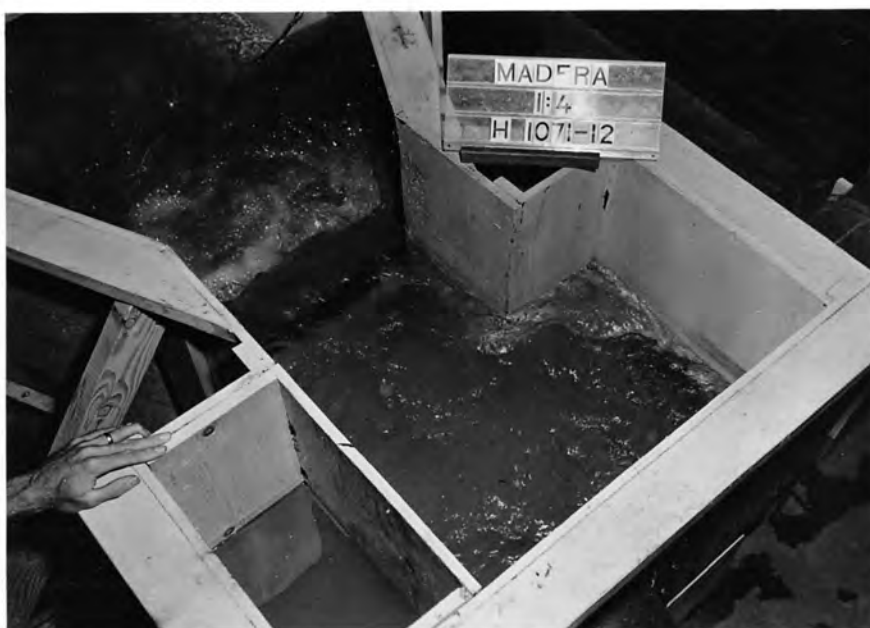
(B) Ell-shaped Forebay--60 cfs Total Discharge with Turnout at Right Operating
