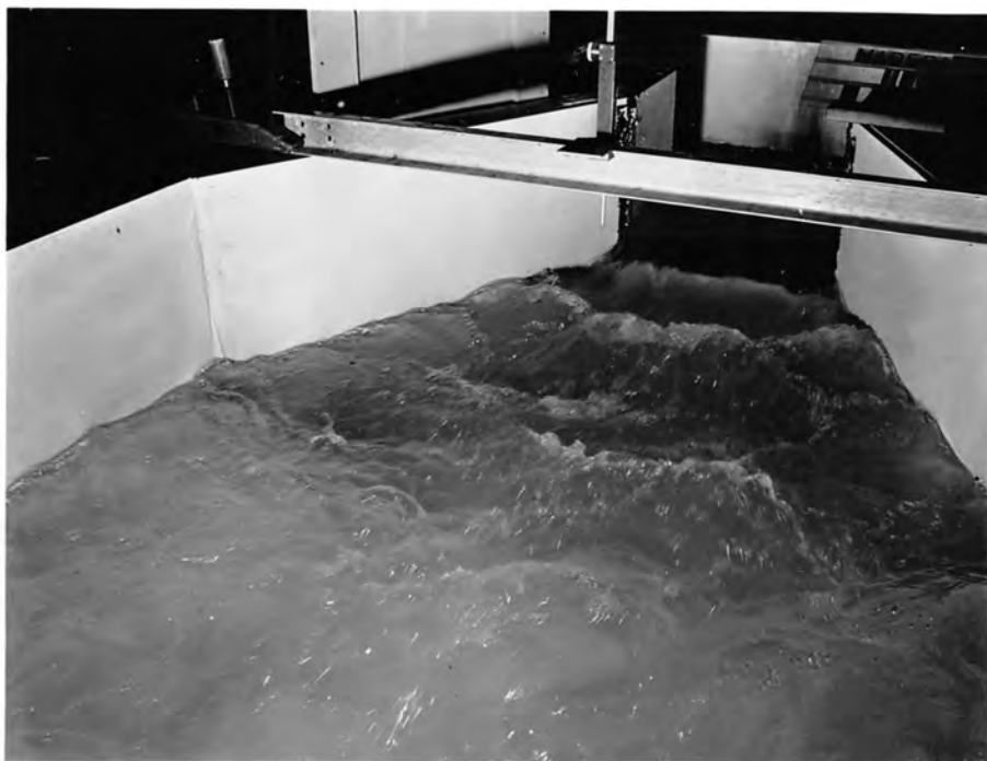
(A) Recommended Stilling Basin--Discharging 60 cfs
