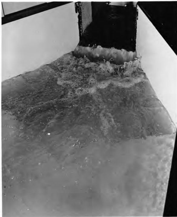
(A) In-Line Forebay--60 cfs Total Discharge with Right Outlet Operating
