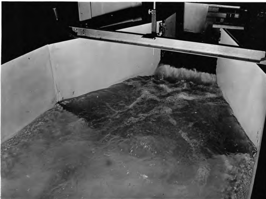
(B) Normal Maximum Tailwater--Discharging 60 cfs
