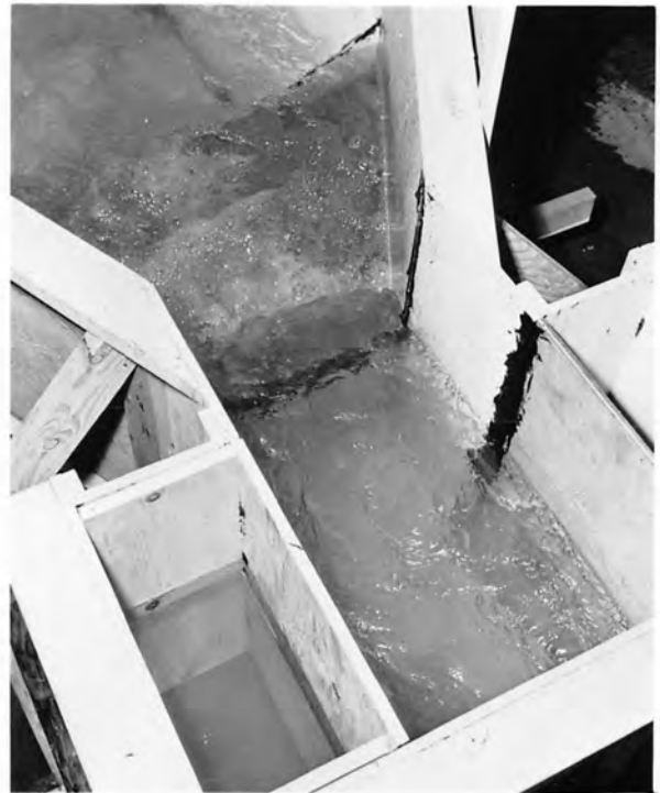
(A) In-Line Forebay--60 cfs Total Discharge with Right Outlet Operating
