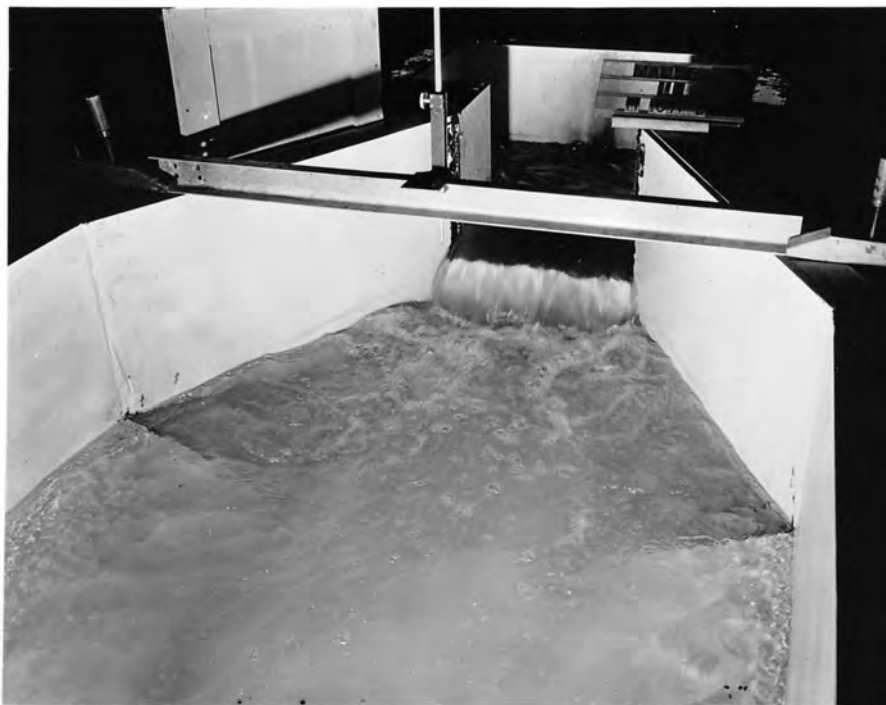
"Broken-Back" Stilling Basin with Sloping Floor and Discharging 60 cfs STILLING BASIN WITH "BROKEN BACK" TRANSITION AND SLOPING FLOOR
