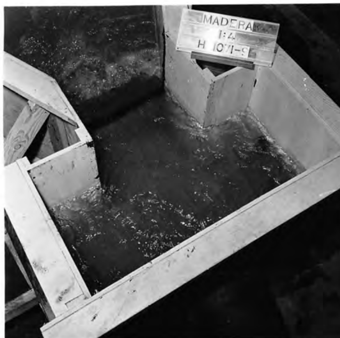
(A) Tee-Shaped Forebay--60 cfs Total Discharge with Right Turnout Operating
