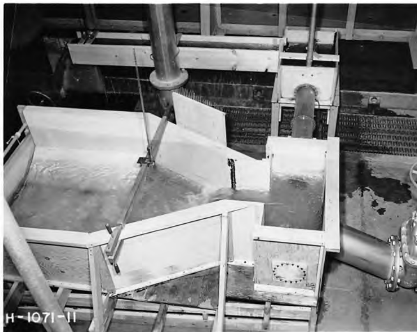
(B) Over-all View with Tee-shaped Forebay--60 cfs Total Discharge with Right Outlet Operating
