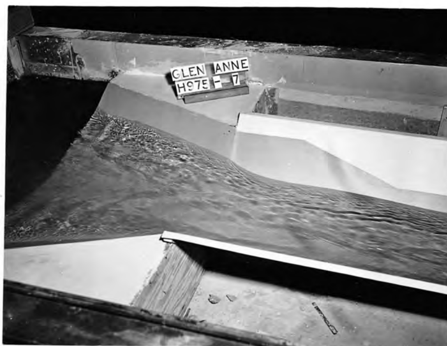
(b) Recommended design - 910 cfs.
