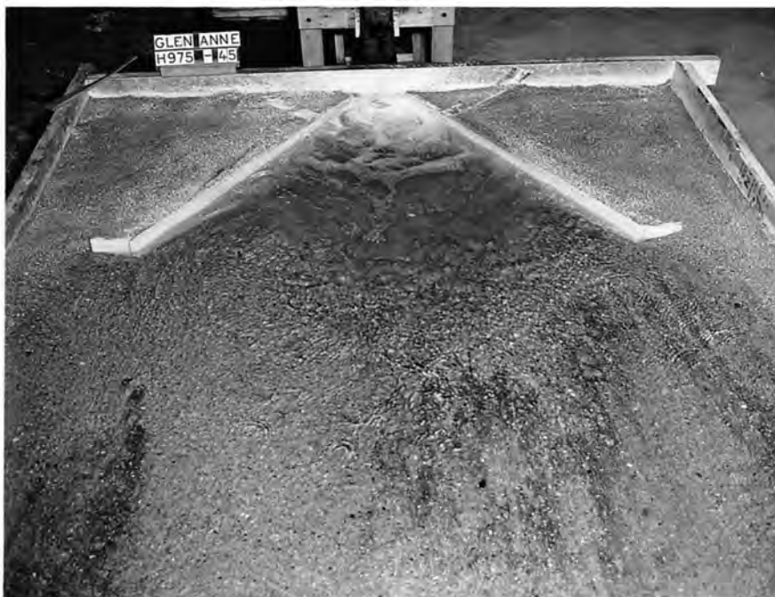
(a) Water Leaving Stilling Basin - 400 cfs
