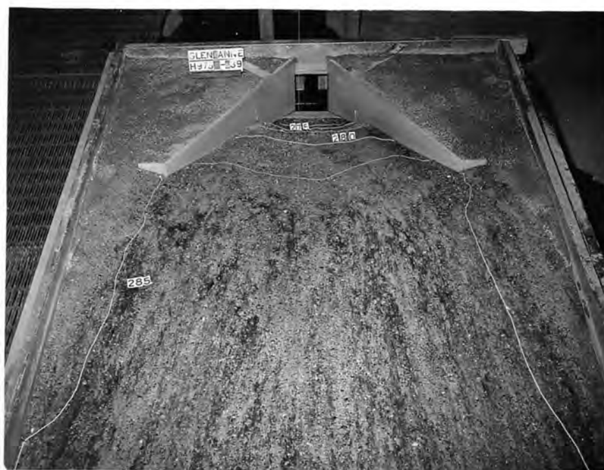
(b) Scour After 30 Minutes of Model Operation
