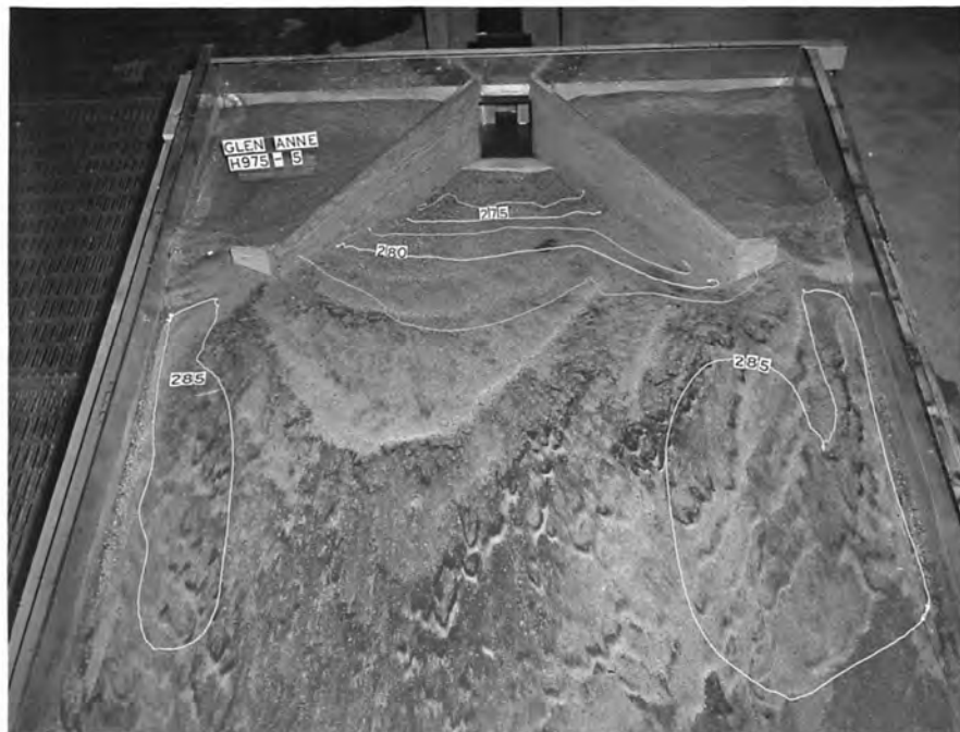
(b) Scour after 30 minutes of model operation
