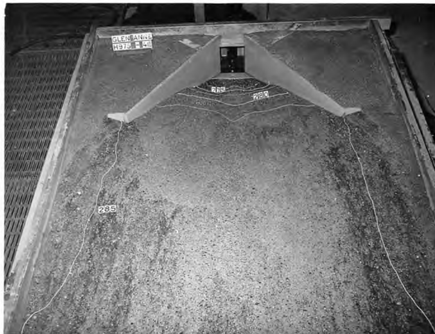
(a) Water Leaving Stilling Basin - 910 cfs
