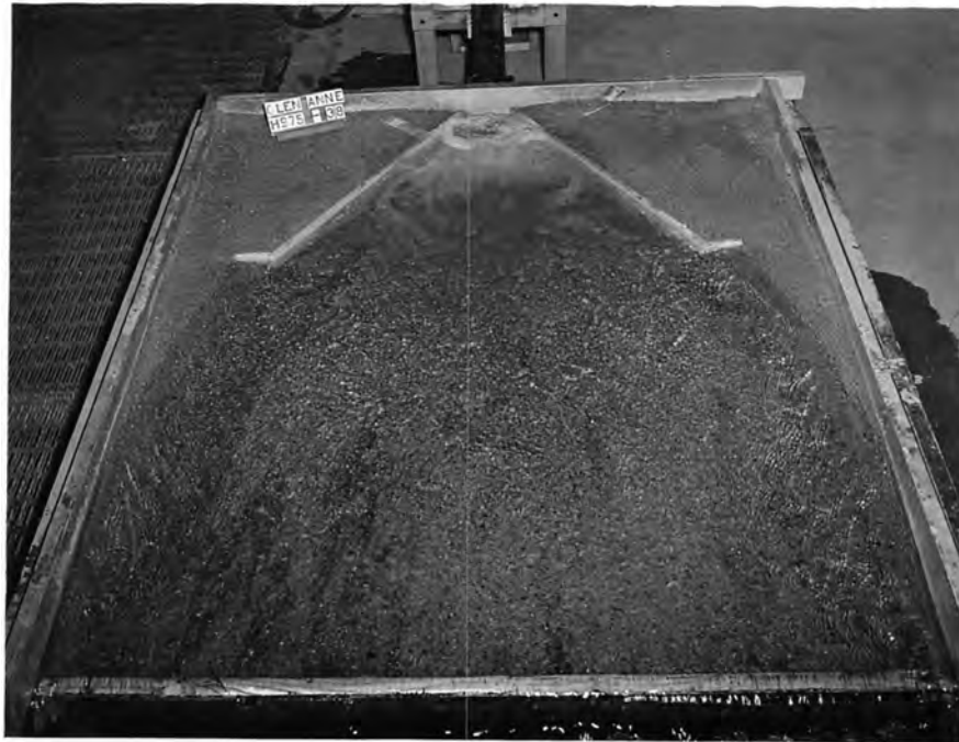
(a) Water Leaving Stilling Basin - 910 cfs.
