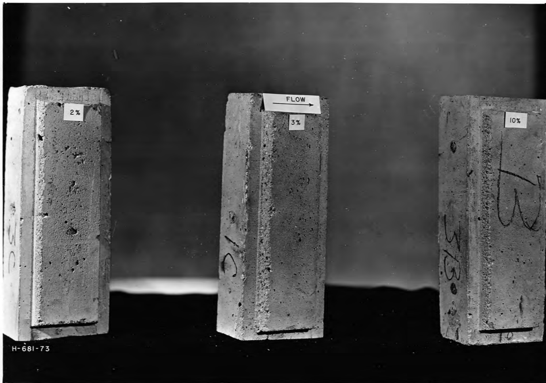
GLENN ANNE DAM SPILLWAY AND STILLING BASIN Cachuma Project EFFECTS OF ENTRAINED AIR ON CAVITATION DAMAGE (2 to 10%)
