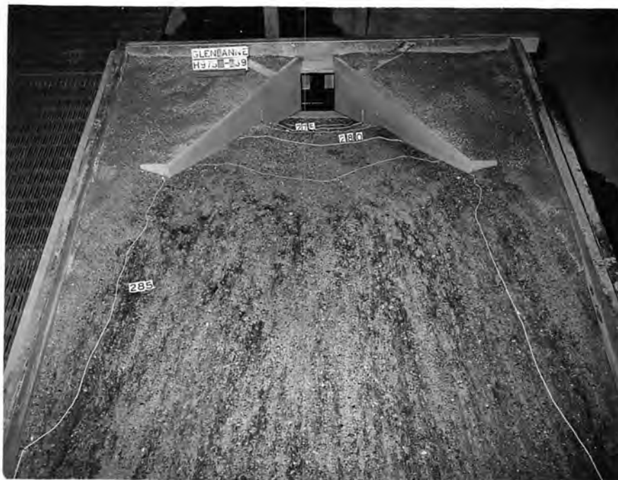
(a) Water Leaving Stilling Basin - 910 cfs.
