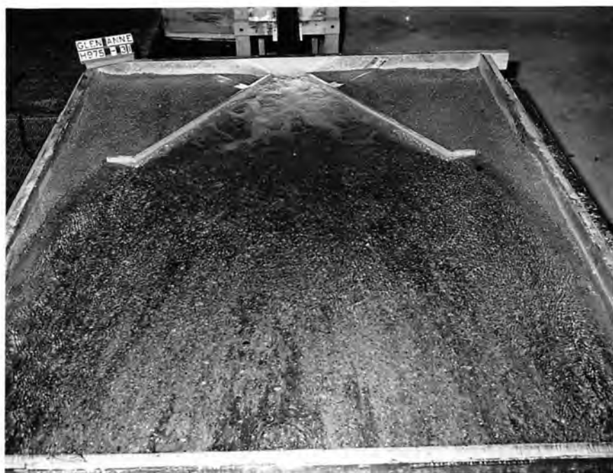
(a) Water Leaving Stilling Basin - 910 cfs.
