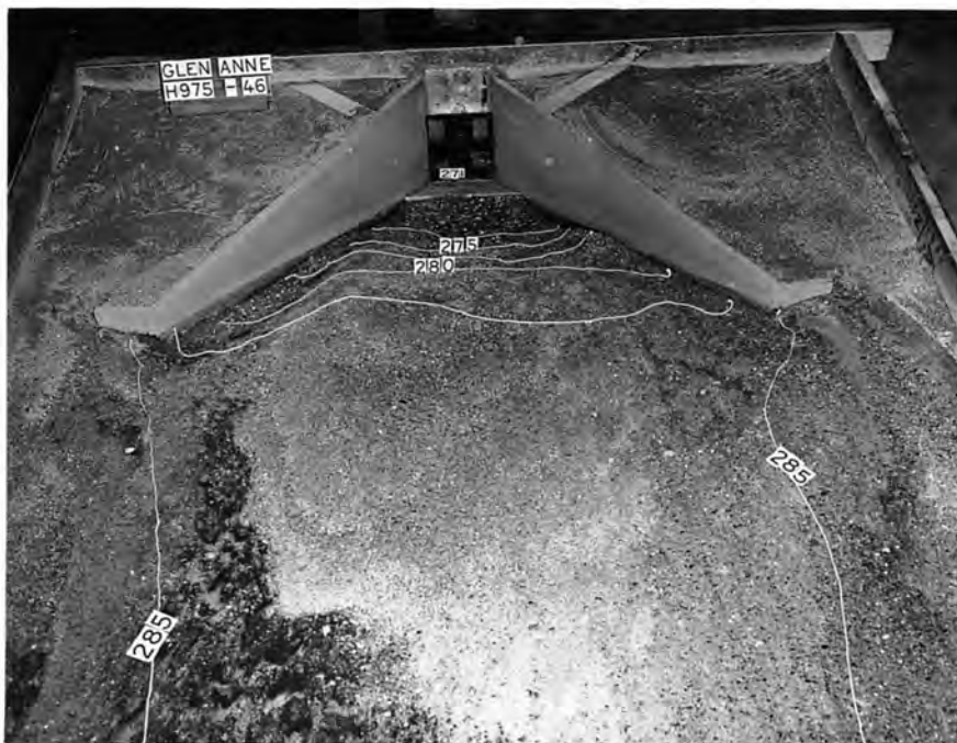
(b) Scour After 30 Minutes of Model Operation at 910 cfs
