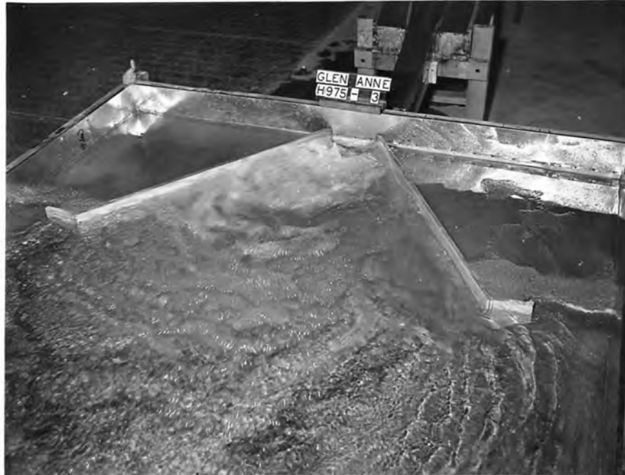
(a) Water leaving preliminary stilling basin - 840 cfs.
