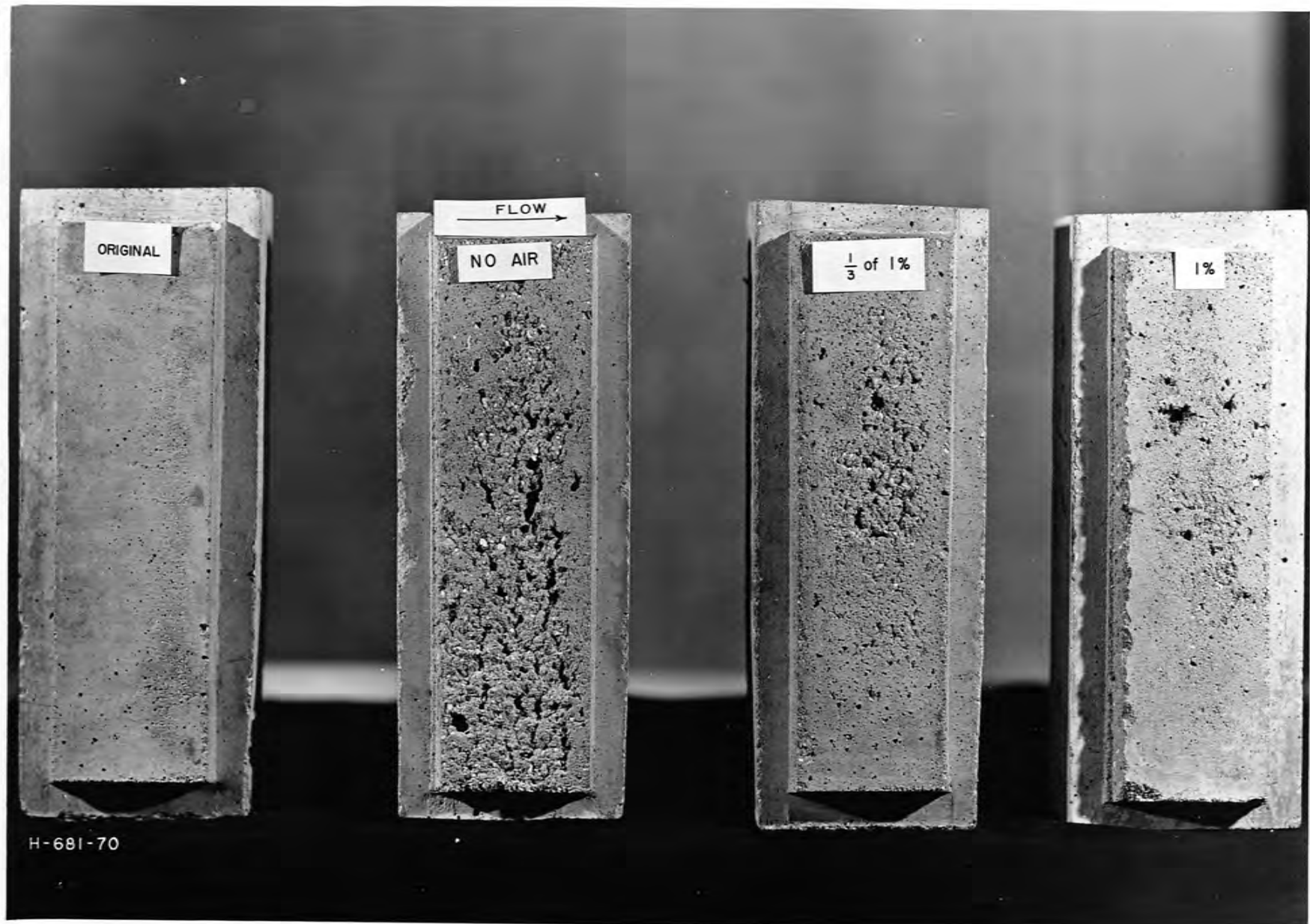
GLEN ANNE DAM SPILLWAY AND STILLING BASIN Cachuma Project EFFECTS OF ENTRAINED AIR ON CAVITATION DAMAGE (0 to 1%)
