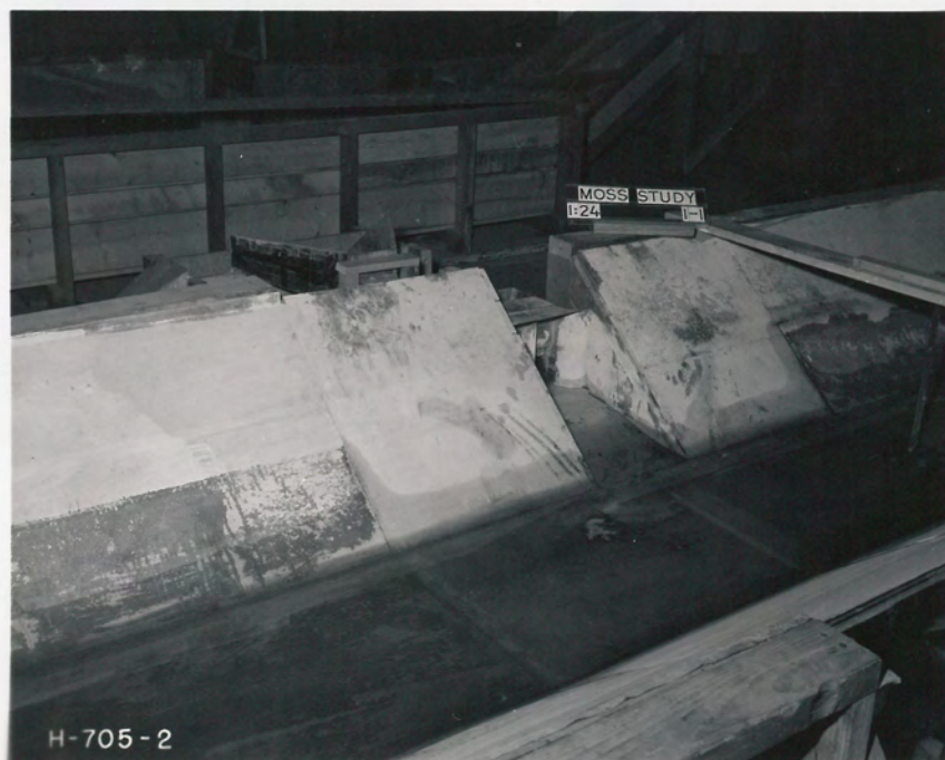
View of model canal showing box turnout.
