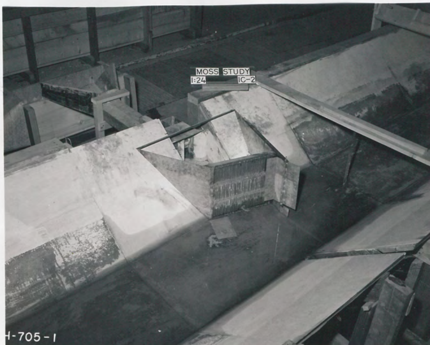
Device C in place and ready for testing. Flow is from right to left.
