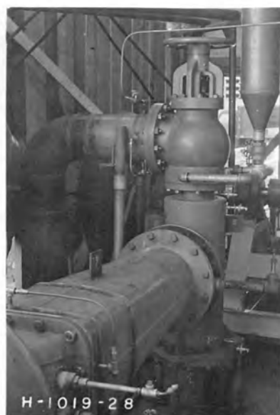
A. Three-stage energy absorber installed for testing.
