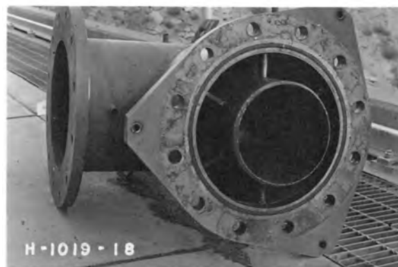
C. Stage 2 of absorber with bottom cover removed.
