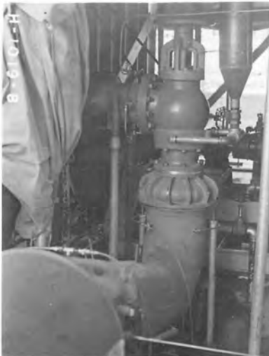
A. Pelton energy absorber installed for testing.
