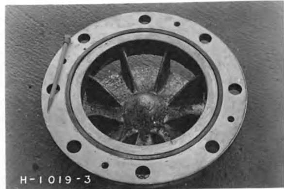
B. Flow spreader looking downstream.
