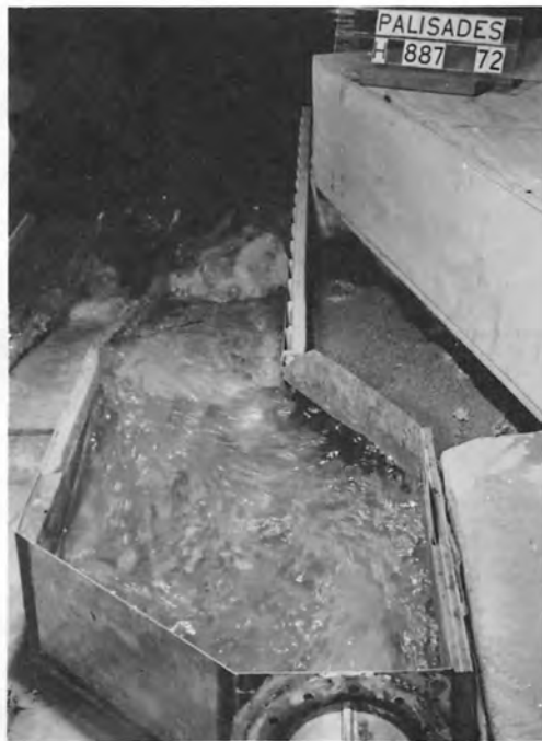
C. Penstock diversion Deflector wall 1--Discharge 18,000 cfs
