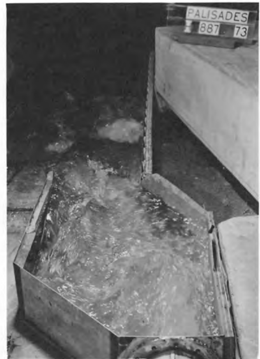
D. Penstock diversion--Deflector wall 1--Discharge 23,000 cfs
