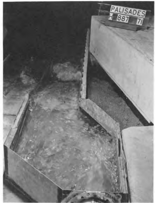
B. Penstock diversion--Deflector wall 1--Discharge 13,000 cfs
