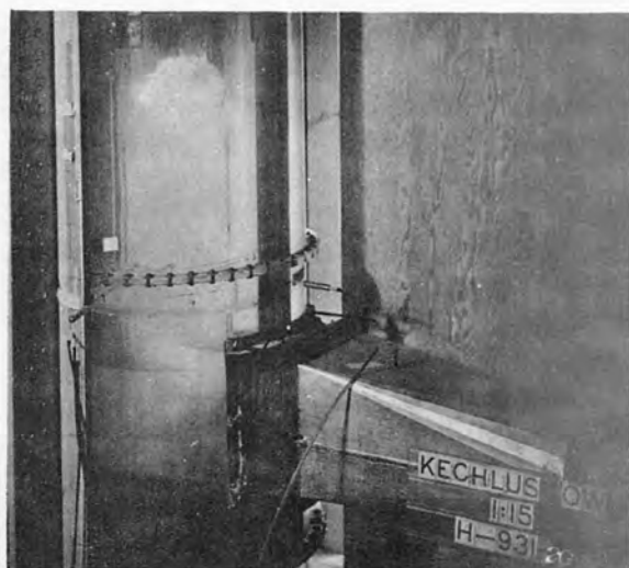
VIBRATION STUDIES - KEECHELUS OUTLET WORKS Flow disturbance in model gate tower--Discharge 2720 cfs Reservoir Elevation 2520--Lower ring gate 50 percent open
