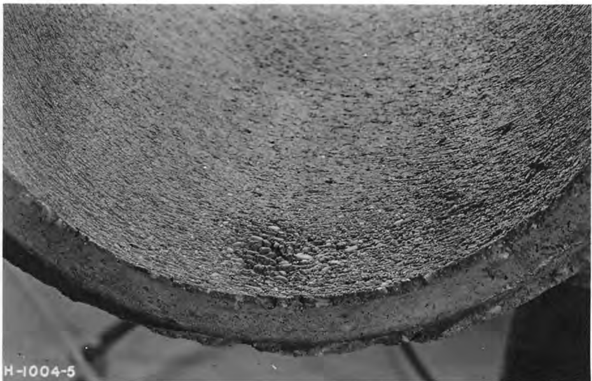
B. Upstream end of pipe section after valve was operated 23 percent open for 33 hours under head of 81 feet.
