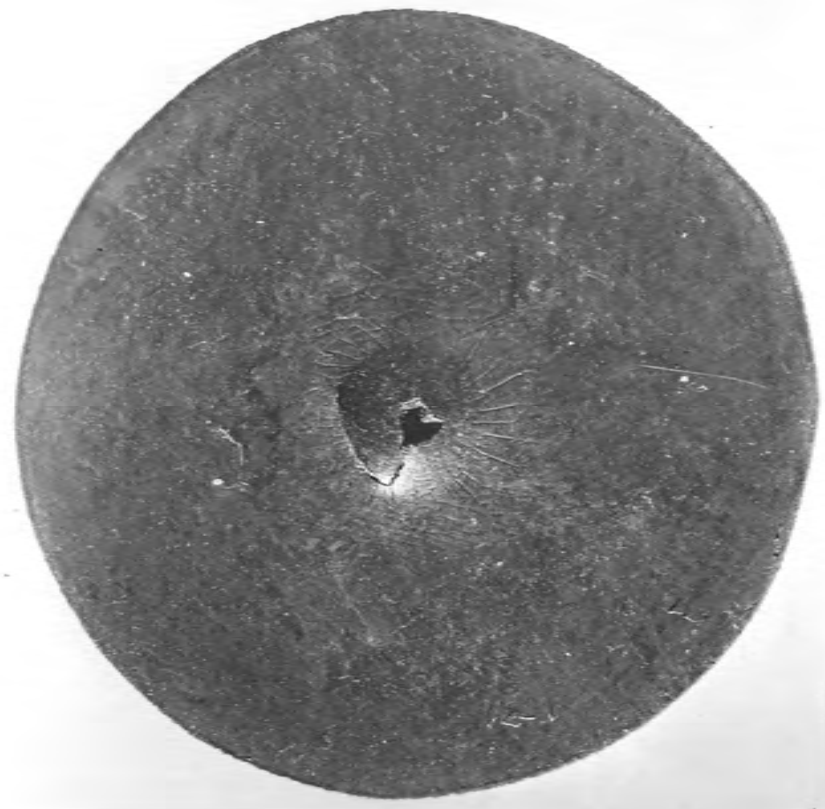
B. Surface of 3/16-inch thick rubber specimen after 5 hours in magnetostriction oscillator.
