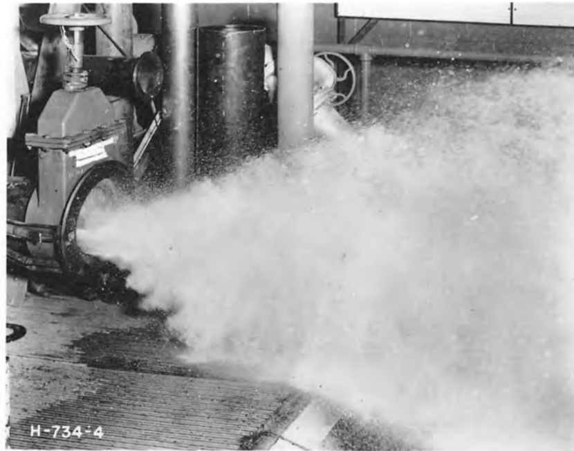
A. Gate valve with 6.1 cfs free discharge at 125-foot head - valve 17.5 percent open.
