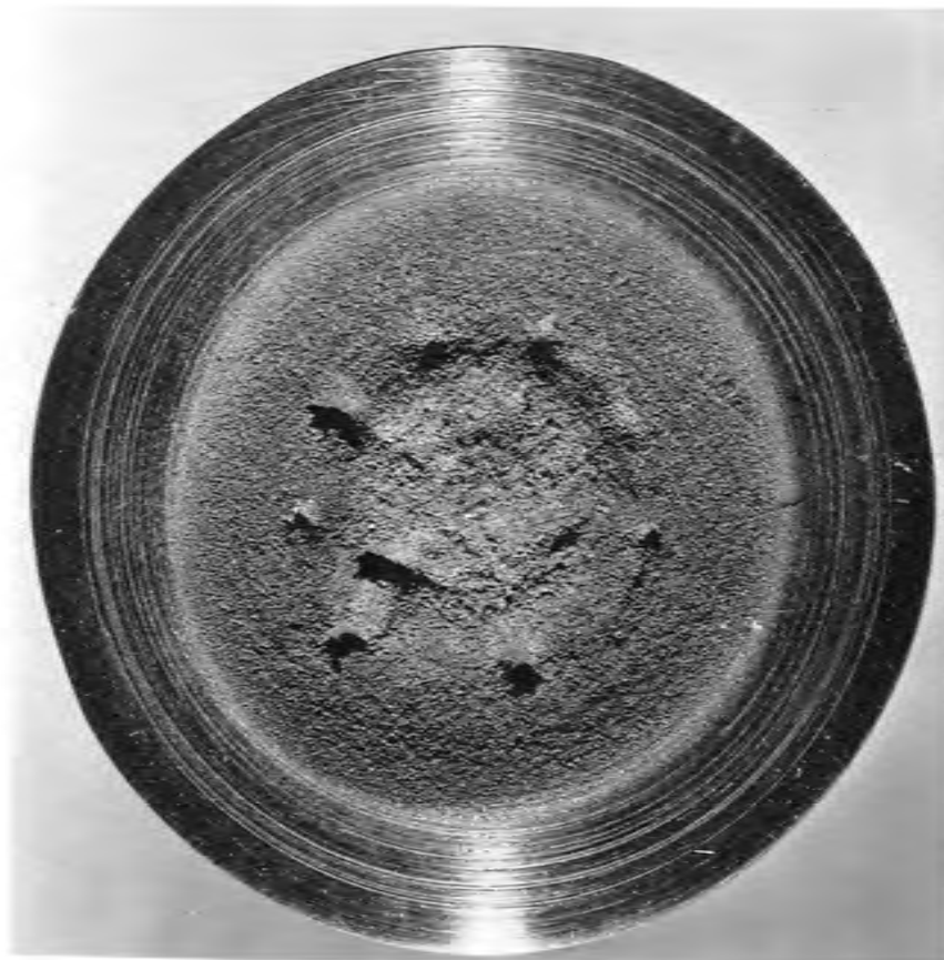
B. Surface of steel specimen after 10 hours in magnetostriction oscillator.
