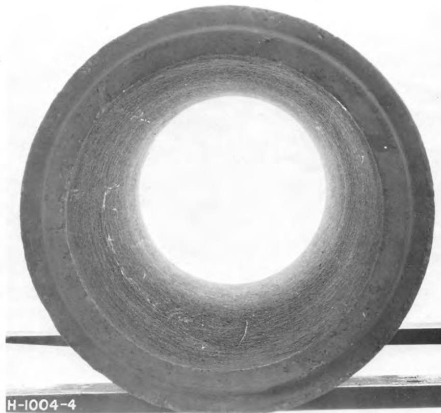
A. Section of 12-inch concrete pipe before test.
