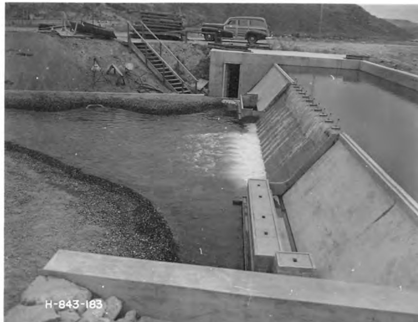
B. 1:60 Model of Grand Coulee Dam operating at a discharge representing 346,000 cfs
