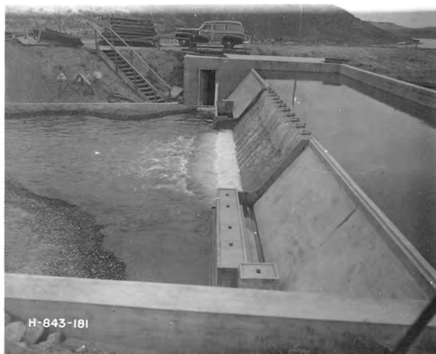
A. 1:60 Model of Grand Coulee Dam operating at a discharge representing 500,000 second feet
