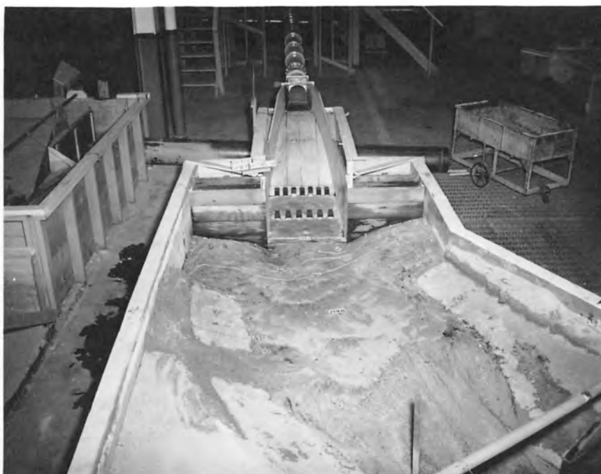
B. Scour after 1 hour at 5,000 second-feet Tailwater elevation 2204.5
