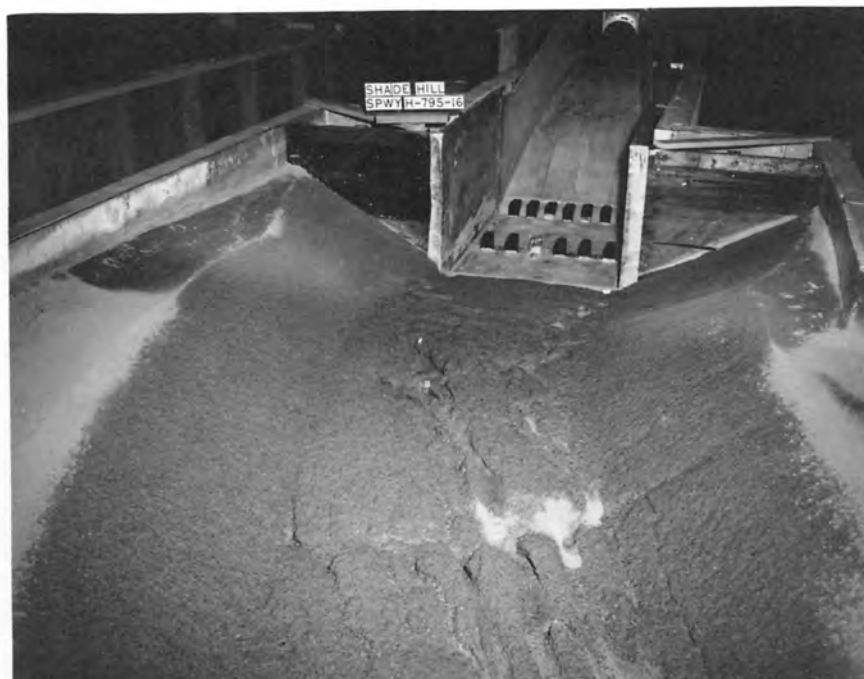
B. Scour after 7 hours at 5,000 second-feet with stabilized sand--closeup view
