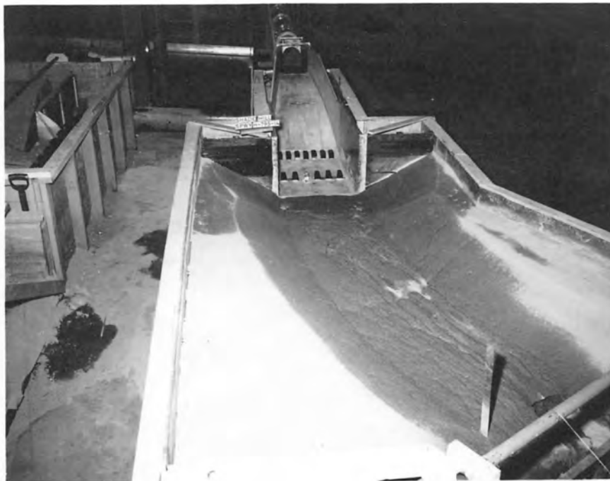
A. Scour after 7 hours at 5,000 second-feet with stabilized sand--overall view Tailwater elevation 2204.5
