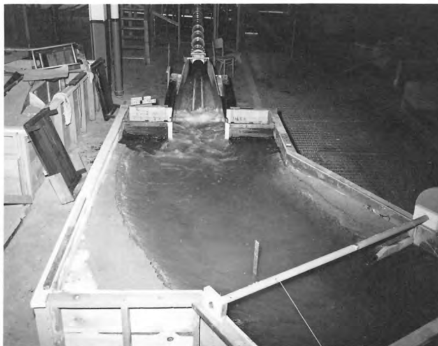
A. Operation at 5,000 second-feet Tailwater elevation 2204.5
