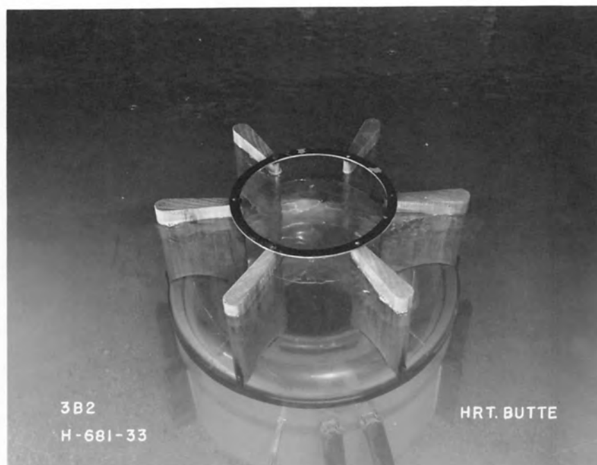
B. Crest with Pier No. 5--Recommended Discharge 3,750 second-feet
