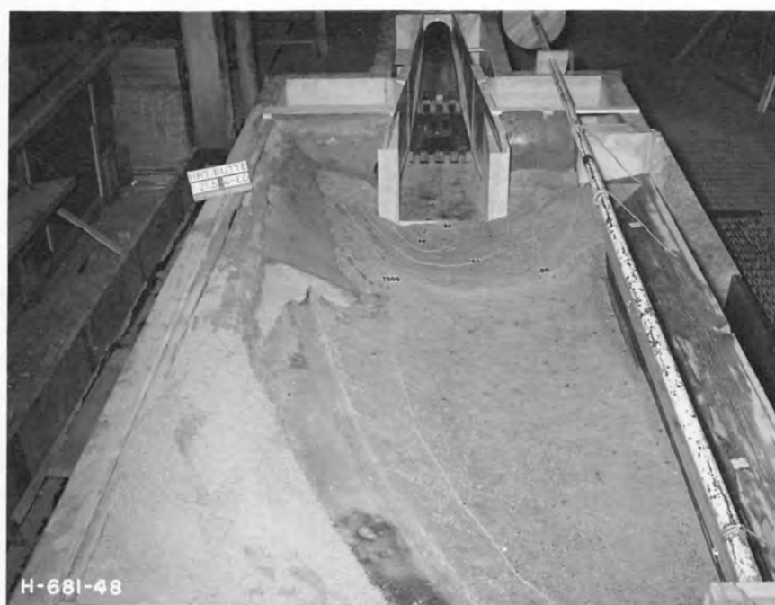
B. Scour after 1/2 hour at 5,600 second-feet T.W. 2012
