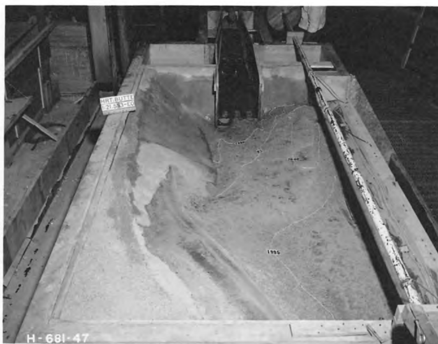
B. Scour after 1/2 hour at 5,600 second-feet T.W. 2012
