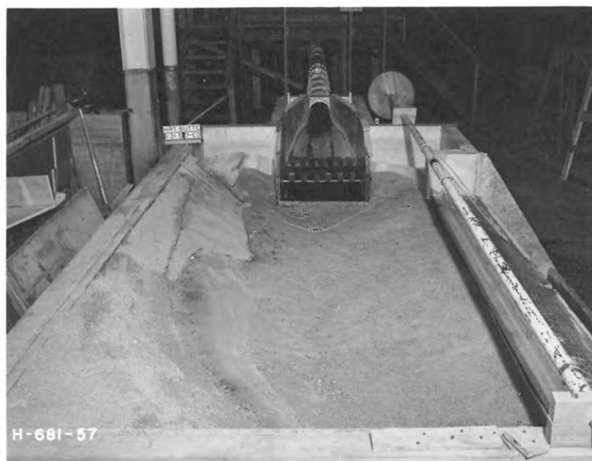
B. Scour after 1/2 hour at 5,600 second-feet T.W. 2012
