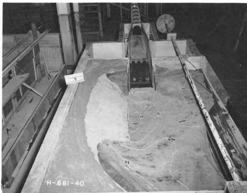
B. Scour after 1/2 hour at 5,600 second-feet T.W. 2012
