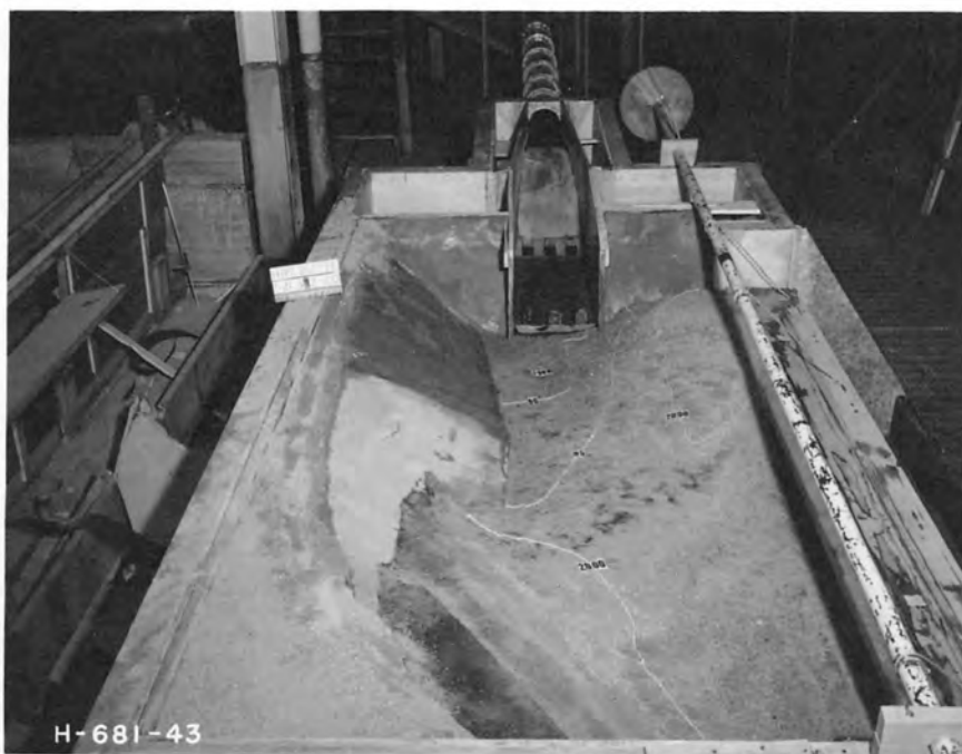
B. Scour after 1/2 hour at 5,600 second-feet T.W. 2012
