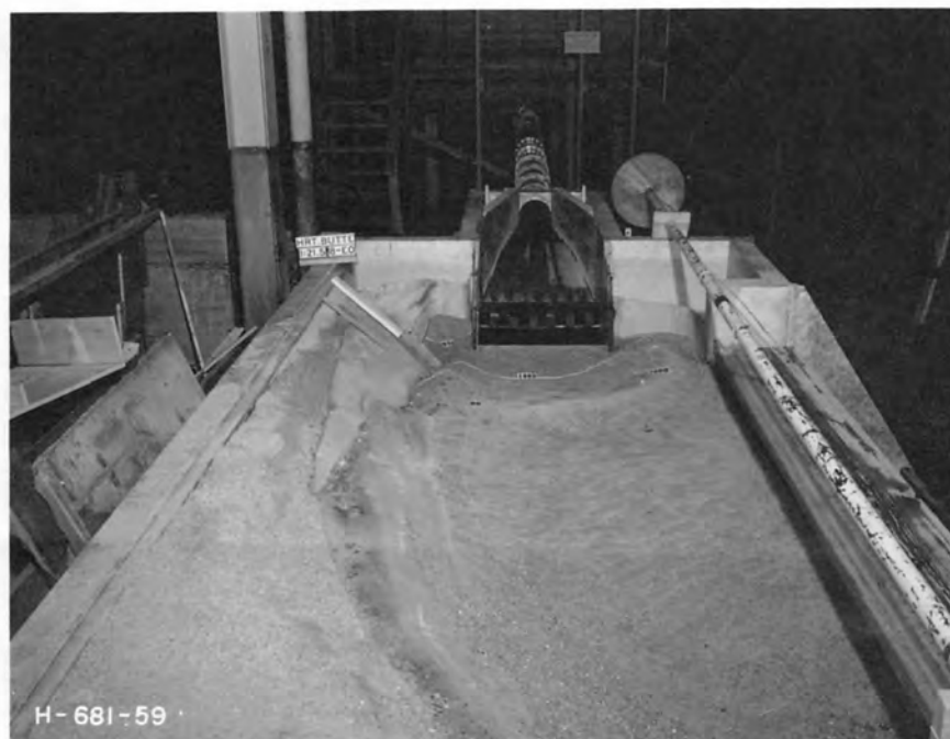
B. Scour after 1/2 hour at 5,600 second-feet T.W. 2012
