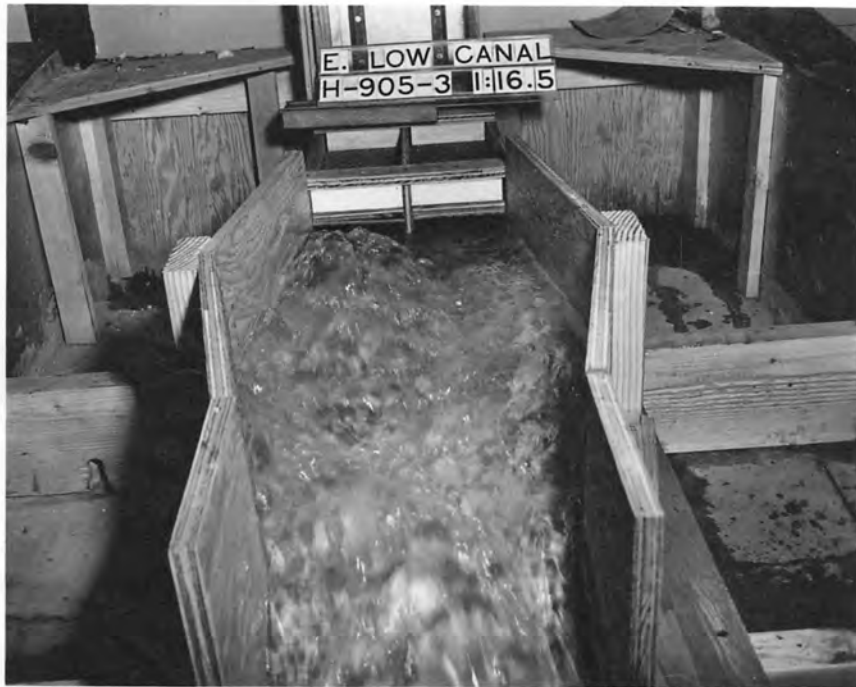
A. Discharge 360 cfs--Note standing wave and uneven distribution of flow.
