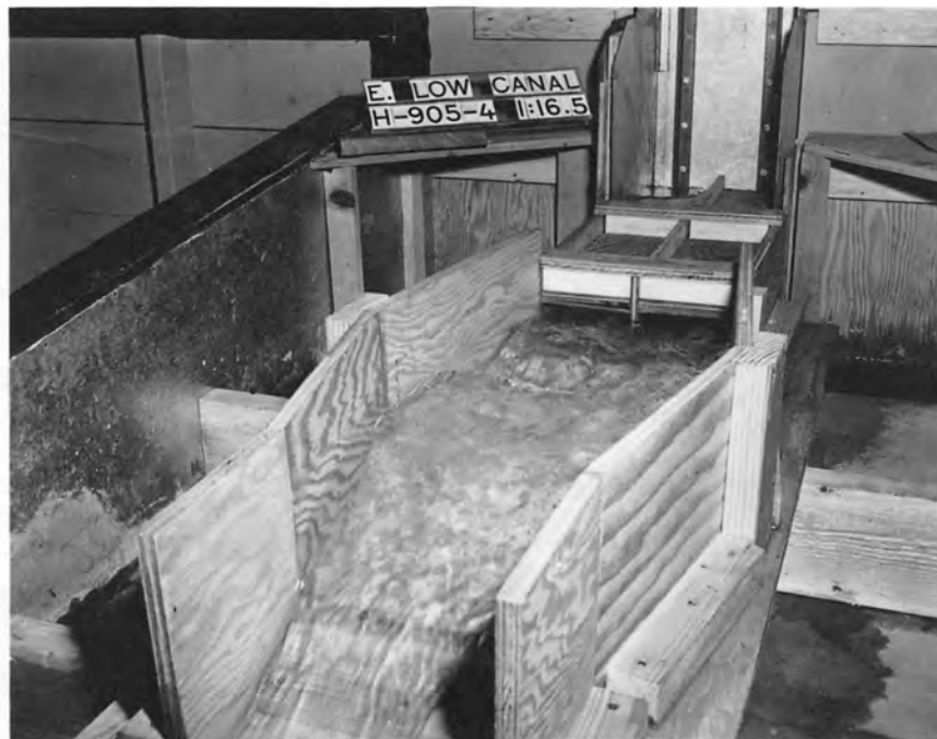
B. Discharge 180 cfs--Wave is smaller
