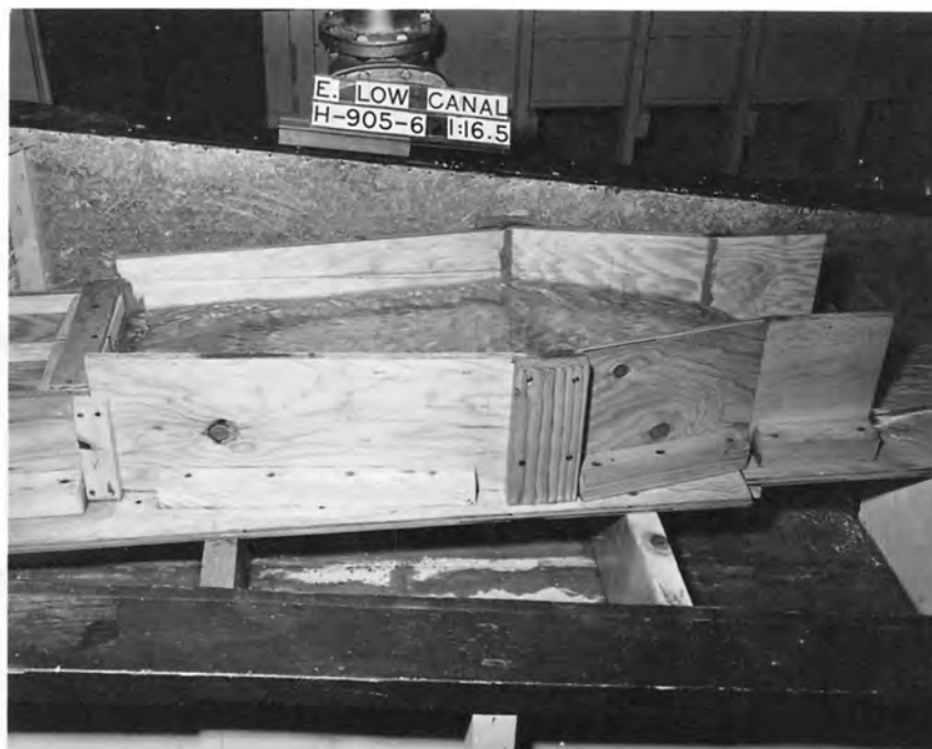
B. Transition No. 3 - No blocks, Discharge 360 cfs.
