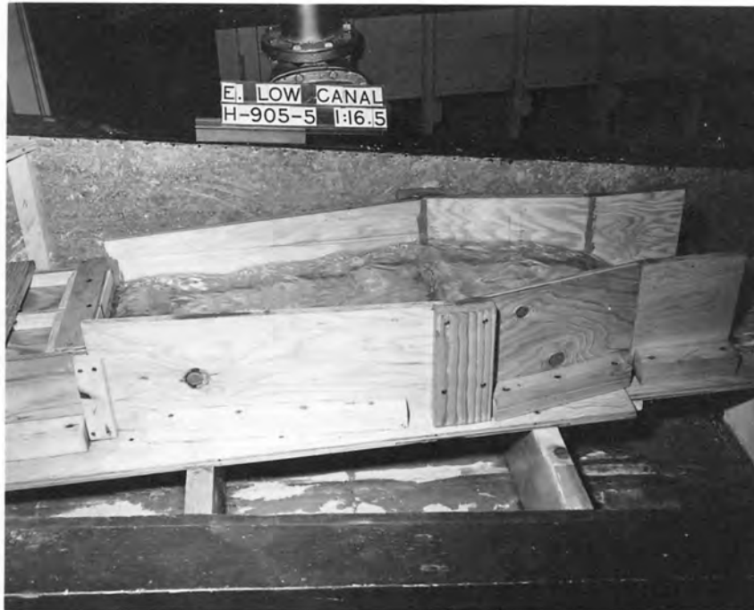
A. Transition No. 2, Discharge 360 cfs.
