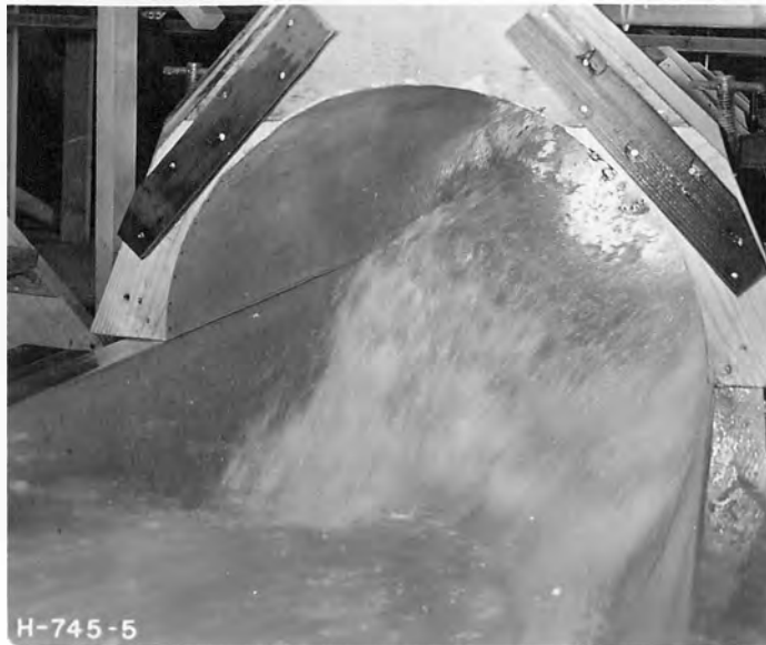
A. Looking Downstream Into the Spillway Tunnel Jet Flow Gate 100 Percent Open Reservoir Elevation 6754
