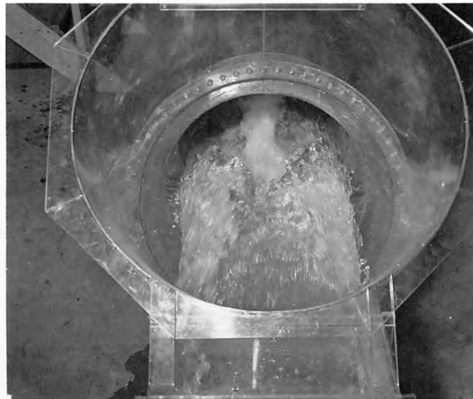
B. Looking Downward into the Spillway Bend Jet Flow Gate 100 Percent Open Reservoir Elevation 6686
