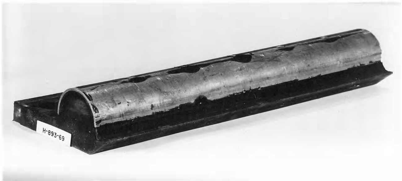
A. Recommended bottom seal with 180 degree, slotted brass shield.
