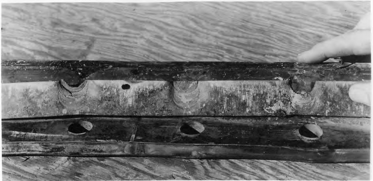
A. Loose 90 degree brass shield showing Allen head clamp plate screw markings, indicating the severe pinching of seal bulb between clamp plate and seat. Same seal as Figure 5.
