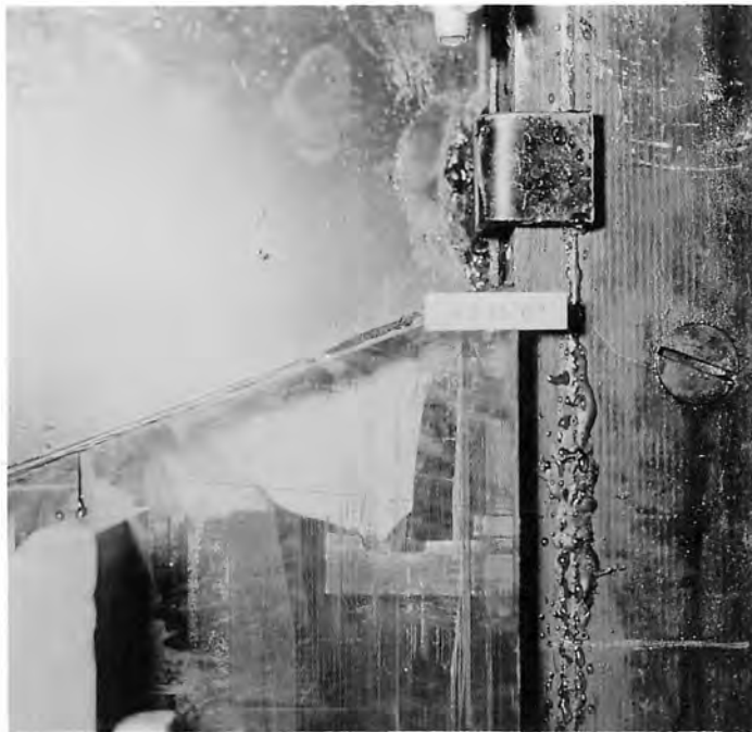
B. Bulb raised above seat at 195 feet head. The bulb showed no tendency to blowout with the minimum compression of beveled stem, \frac{3}{32} inch. This test simulated a failure in the bulb retraction system.
