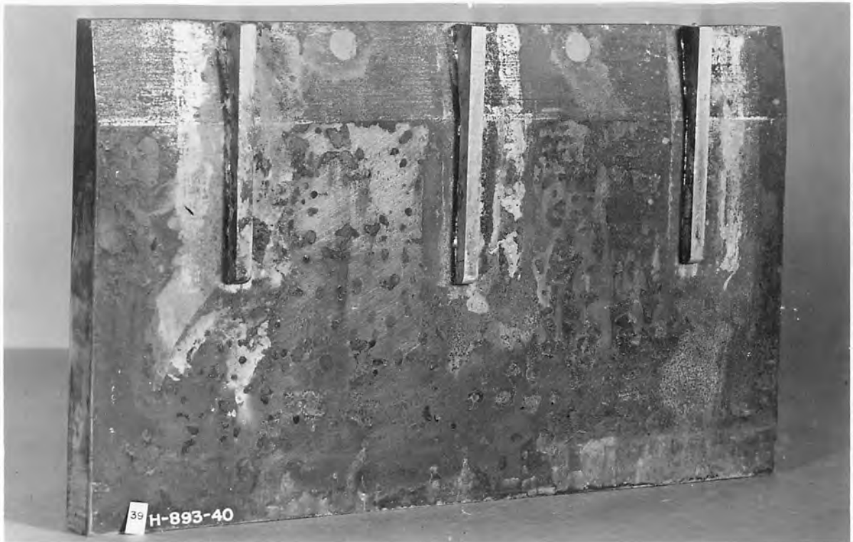
A. Beveled seal seat with brass bars soldered to face. These bars prevented complete sealing, thus decreasing water hammer.
