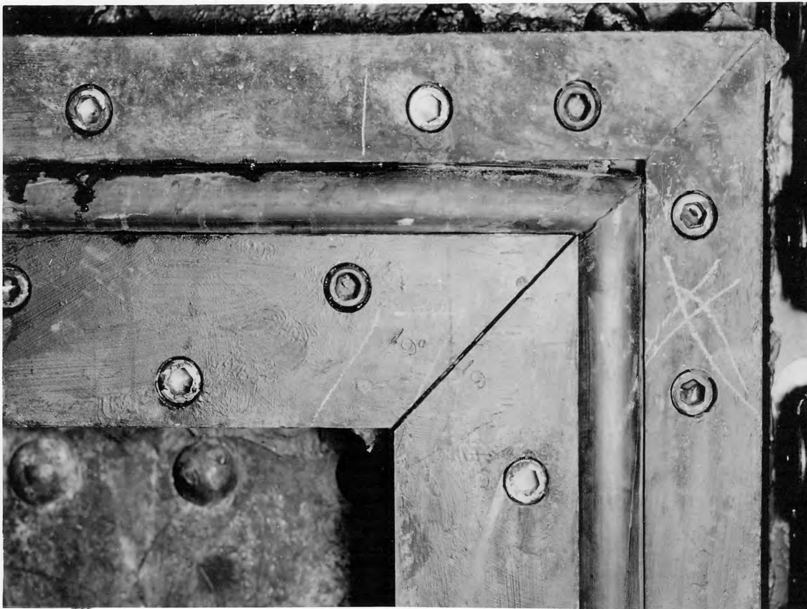
The special rubber seal (Drawing No. 222-D-14970) is shown on the R-6 coaster gate after completion of the simulated emergency closure tests. The photo shows the upper west corner of the seal. The pulled down condition of the seal at the corner was present before the tests and does not appear to have been altered during the tests. October 11, 1950.
