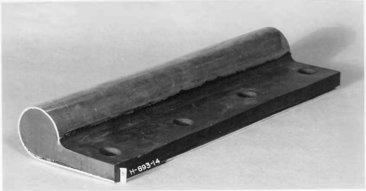
A. Note the poor bond between brass shield and rubber which was typical on seals with large shields.
