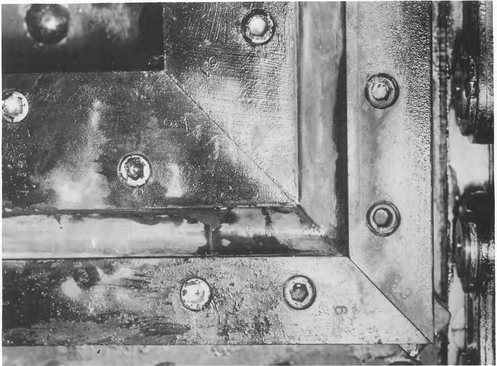
The special rubber seal (Drawing No. 222-D-14970) is shown on the R-6 coaster gate after completion of the simulated emergency closure tests. The photo shows the condition of the lower west corner of the seal. Note the space between the lower clamp bar and the seal. October 11, 1950.
