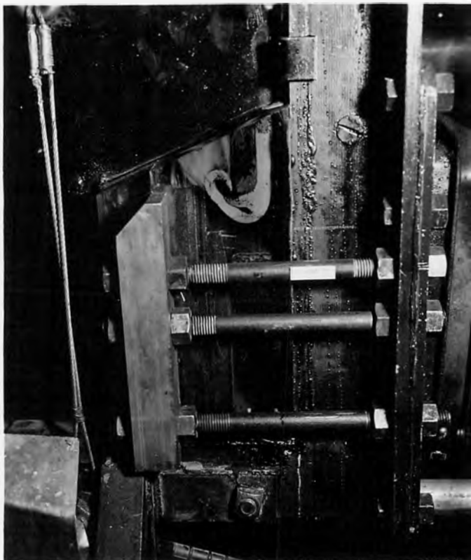
A. End view of seal showing bulb deformation at 195 feet head--no gate movement after applying head. Zero seal-to-seat gap.
