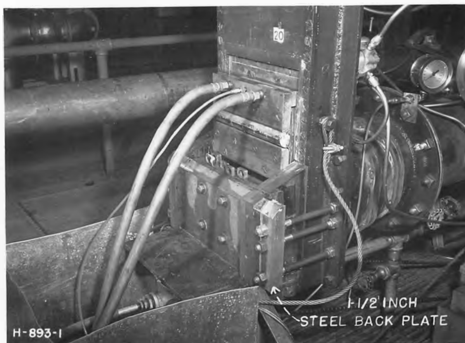
B. View with hood removed showing seal actuating pressure supply hoses, gage line and double stem seal assembly.
