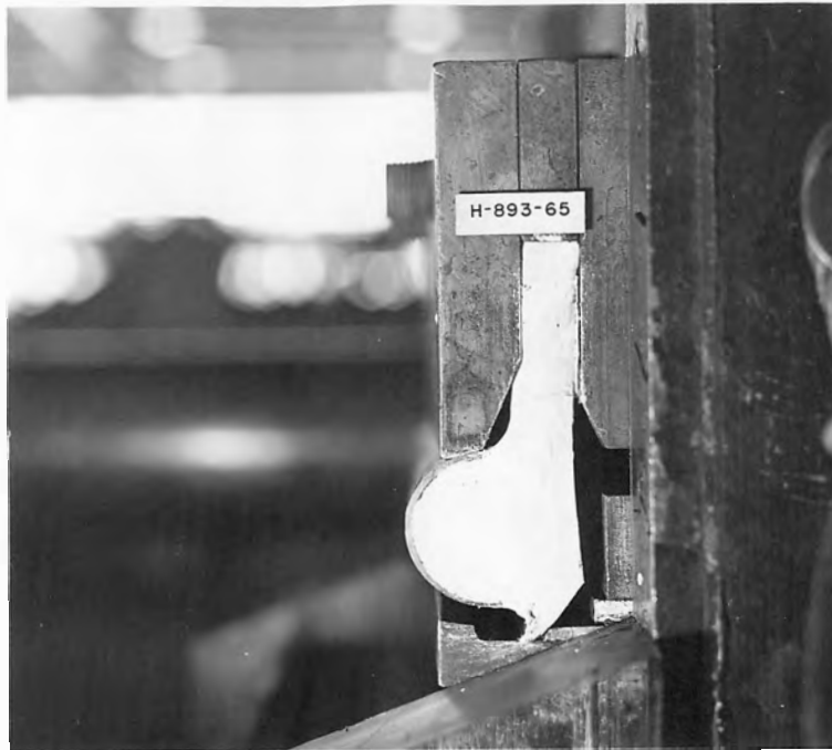
A. Assembly with minimum compression, \frac{3}{32} inch, of beveled stem. Seal end painted white.
