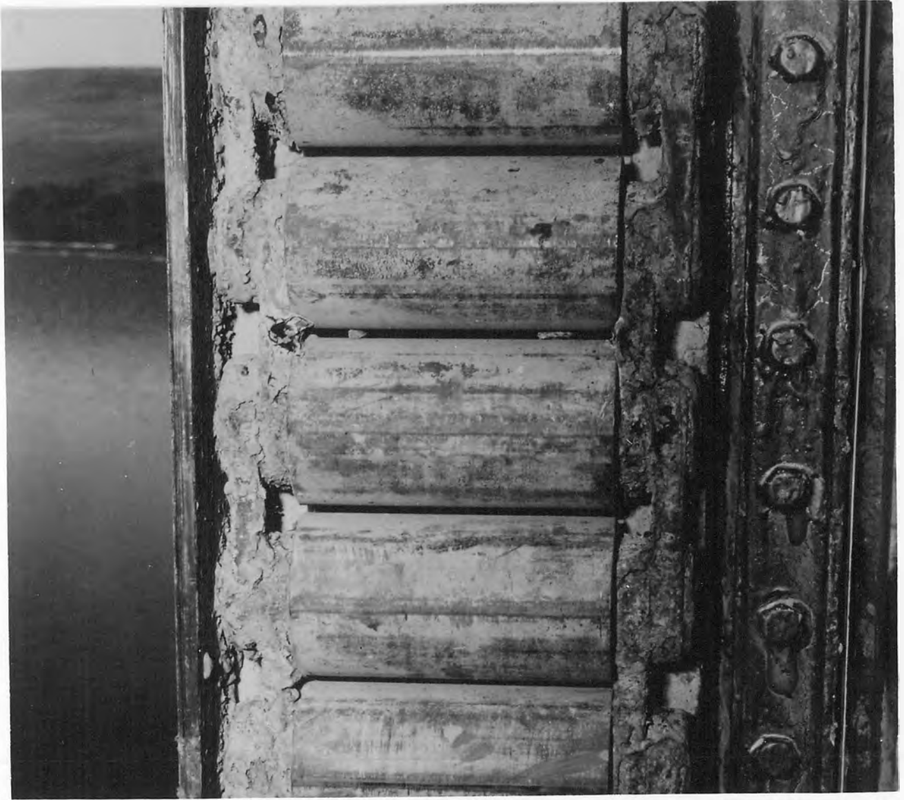
R-6 coaster gate (formerly L-3) lower right roller chain. Photo shows corrosion of the steel chain links. This gate was in service from June, 1941 until November, 1949, and from April, 1950 until August, 1950. The chains are in an inoperable condition, and it may be noted that their sliding action in operation has slightly flattened the contact surface. After removing the rust from the links, many pits were found to be in excess of 1/16 " in depth. August 30, 1950.
