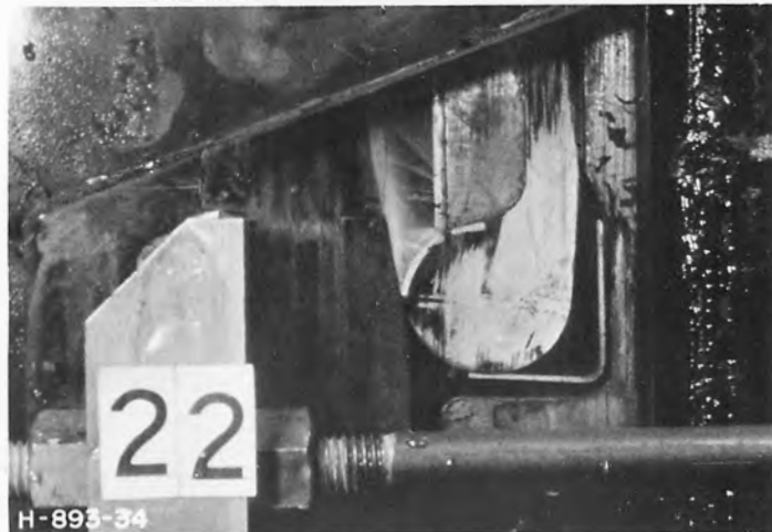
B. Solid bulb music note seal (5/32 inch seal-to-seat gap) with a 90 degree shield which retards bulb deformation and loss of contact with the spring; however, at 195 feet head, the pressure behind the seal bulb was 150 feet which is too high for dependable retraction.
