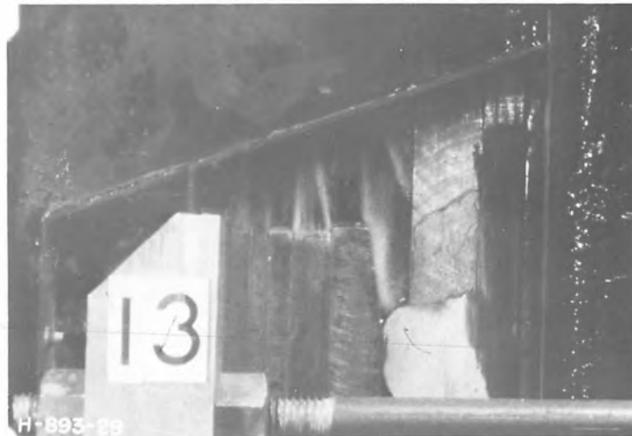
B. Satisfactory gate closure with 1/8-inch seal-to-seat gap.
