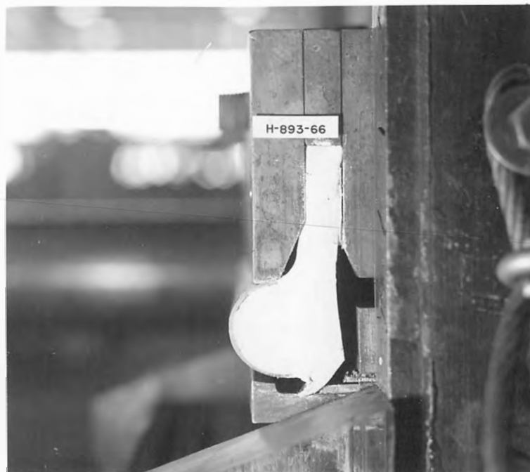
B. Assembly with maximum compression, \frac{7}{32} inch, of beveled stem. Seal end painted white.
