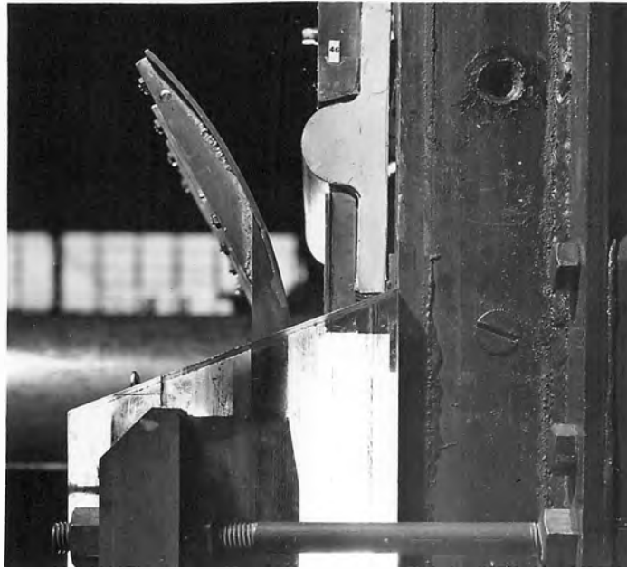
A. Side view of seal assembly showing penstock entrance transition section.
