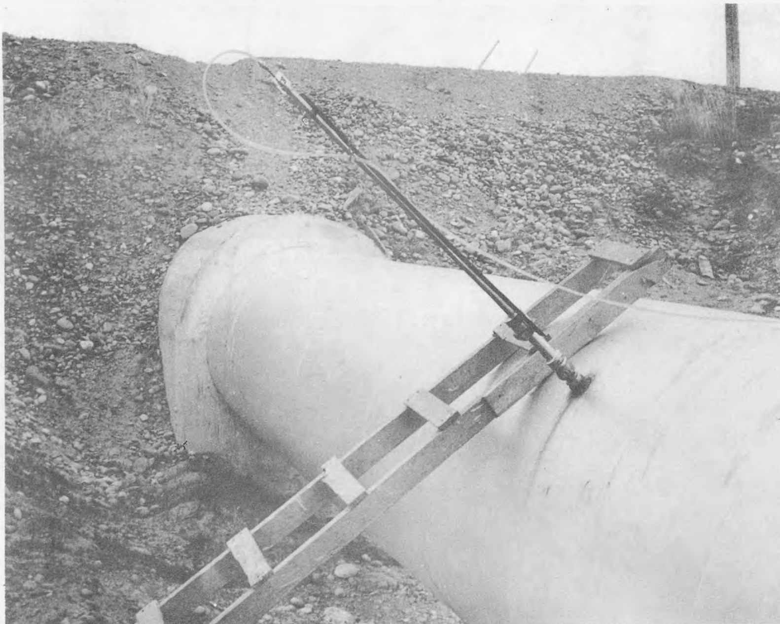
FIGURE 1 Cole Pitometer being used on 60-inch Internal Diameter steel pump discharge line to determine rate of flow.
