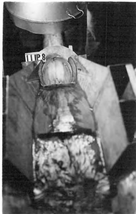
C. FLOW CONDITIONS IN CHUTE WITH DISCHARGE 600 SECOND-FEET
