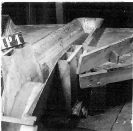
C. REVISED SPILLWAY WITH DIVIDING WALL AND STEPS ON OVERFLOW SECTION
