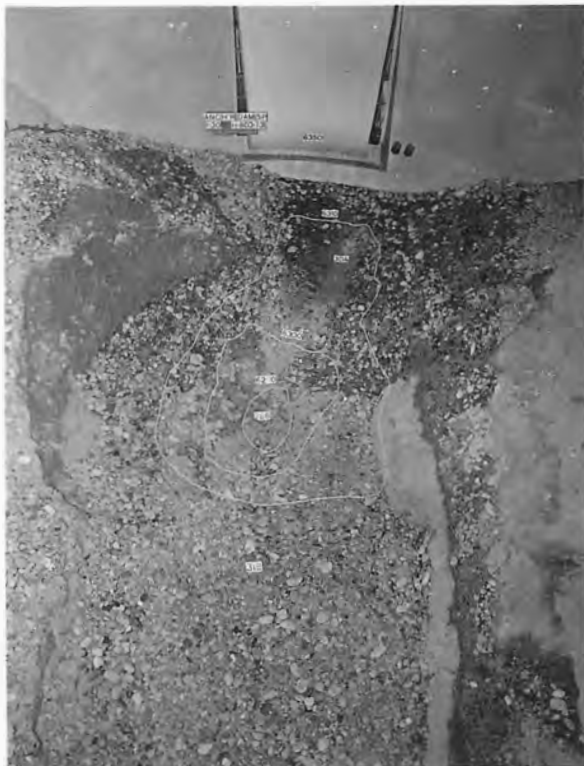
B. Scour after 30 minutes' operation at 5,000 cfs.
