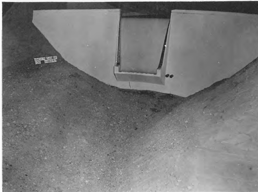
A. Sand and gravel overburden placed on bedrock to elevation 6365.00.
