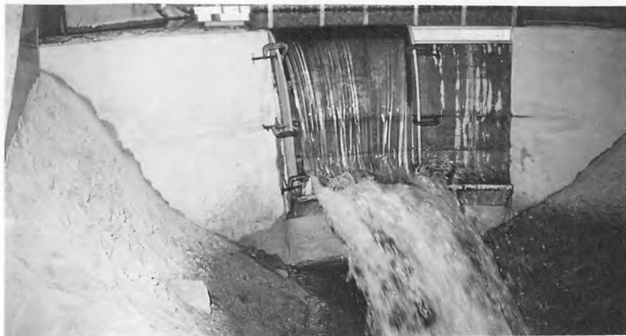
A. Spillway Face Slope = 0.20. 20-foot radius bucket.
