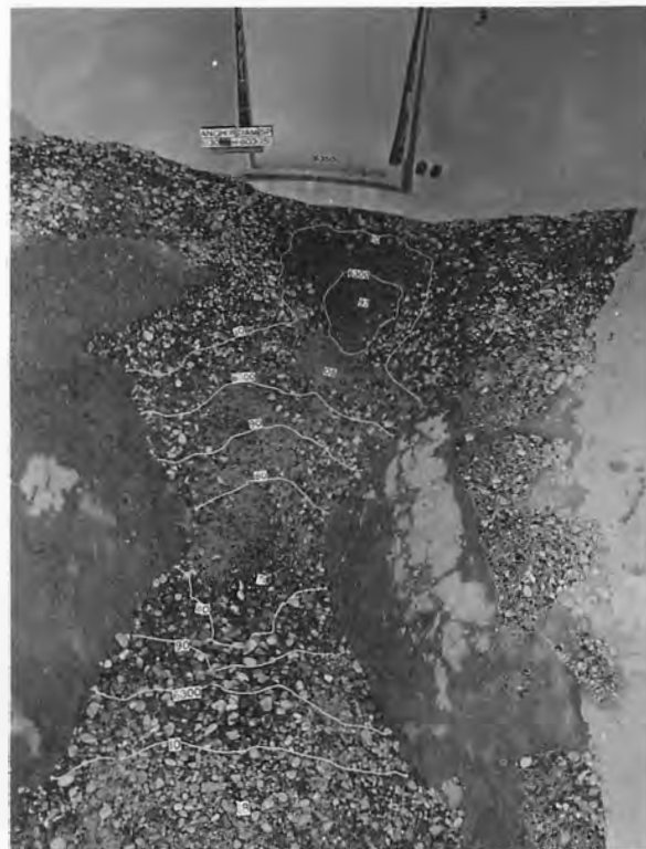
C. Scour after 30 minutes' operation at 13,500 cfs.
