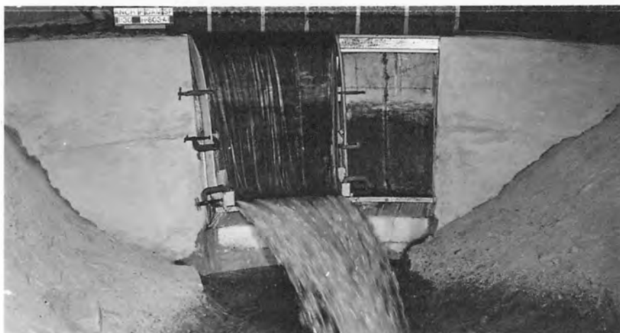
B. Spillway Face Slope = 0.37. Parabolic bucket with the drain slots shown below.
