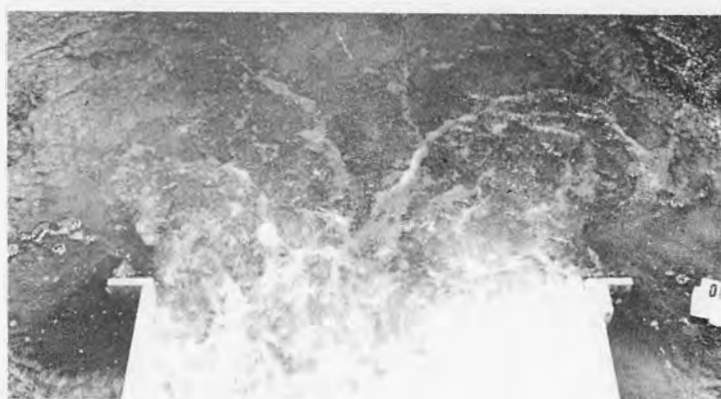
b. Scour Test in Progress after 14 minutes of Model Operation.
