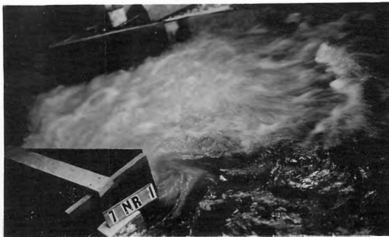
(C) POOL SHAPE "C" — MAXIMUM DISCHARGE TAILWATER ELEVATION 56.0 FEET
