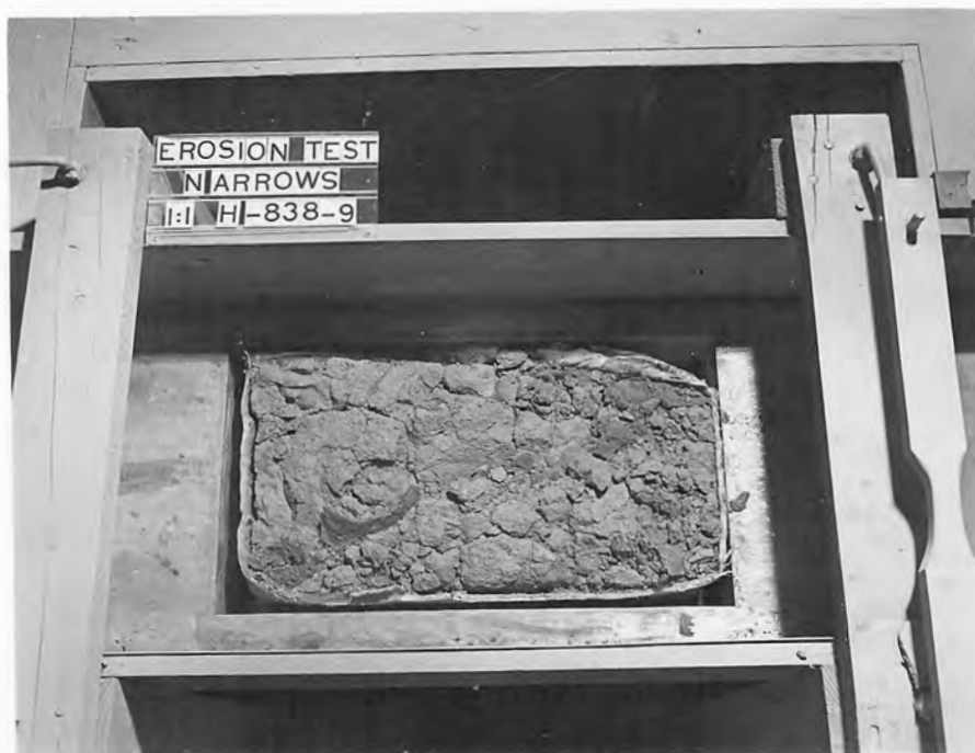
B. Erosion after 2 minutes' exposure at 1.5 fps velocity.
