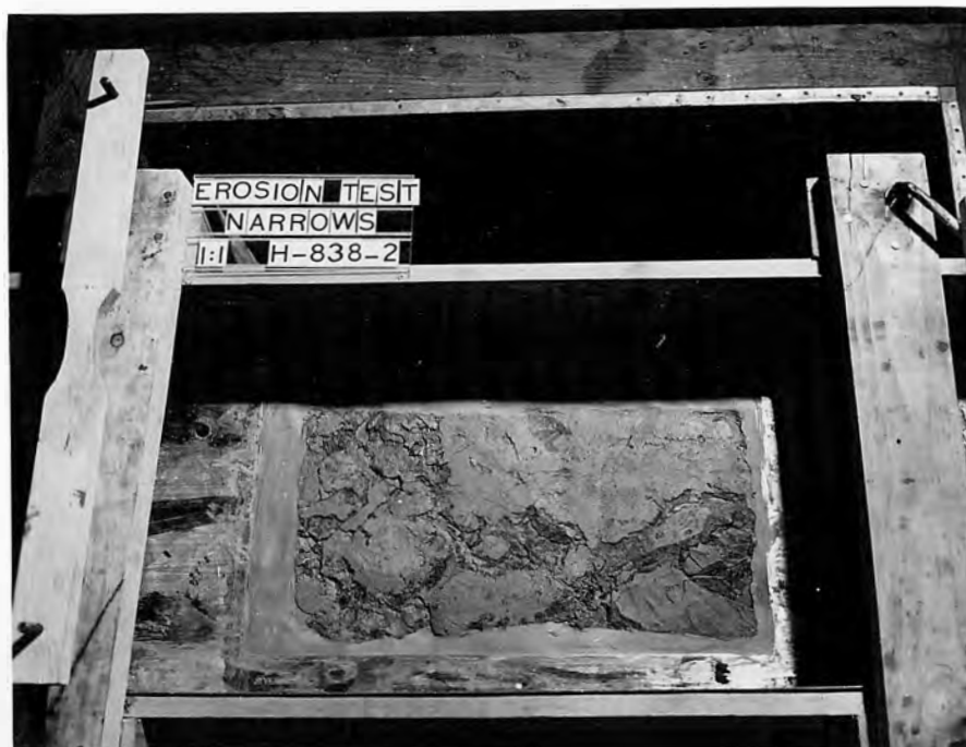
B. Erosion after 1 hour and 40 minutes' exposure at 2 fps velocity.
