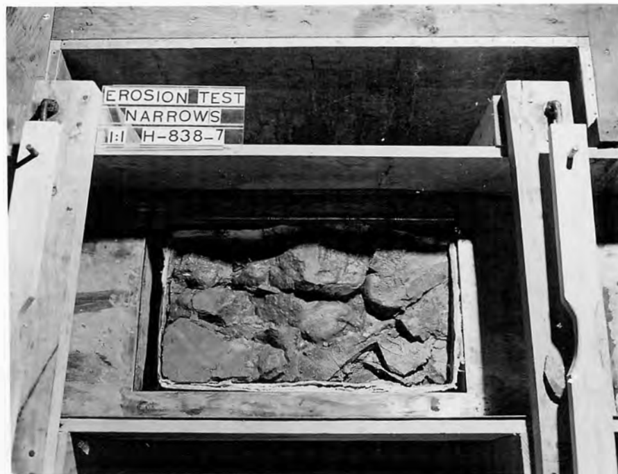
B. Erosion after 3 minutes' exposure at velocities ranging from 12 to 16 fps.
