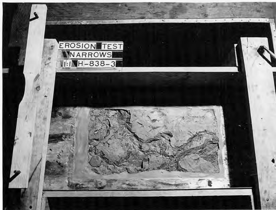
A. Erosion after 1 hour and 40 minutes' exposure at 2 fps, and 1 hour at 4 fps velocity.
