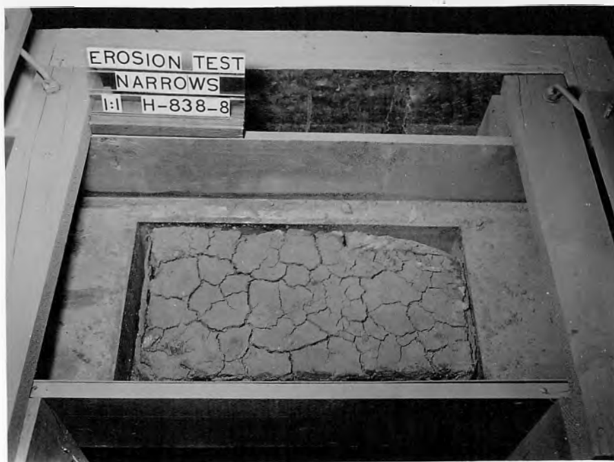
A. Appearance of Test Specimen No. 2 after "weathering" period.
