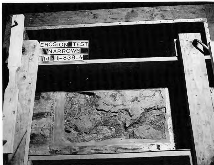
B. Erosion after 1 hour and 40 minutes' exposure at 2 fps, 1 hour at 4 fps, and 1/2 hour at 6 fps velocity.
