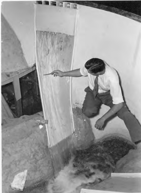
C. Flow climbs training- wall. Gates 4, 5, 6 open.
