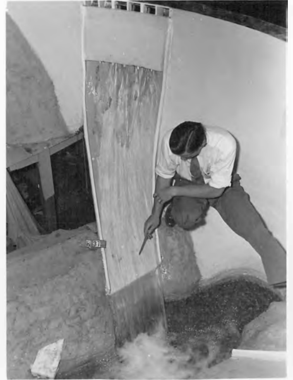
D. Flow well distributed. Gates 4, 3, 2 open.
