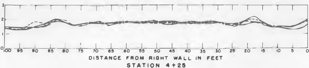
WATER SURFACE PROFILES - COMPARISON OF TAILPIECE DESIGNS USED ON ORIGINAL PIERS
