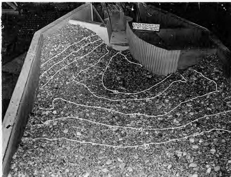
B. Scour after 15 minutes model operation at 4210 cfs.
