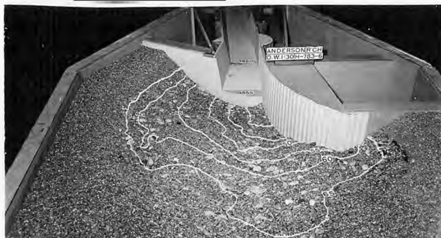
B. Flow in diversion and river channels of model with a discharge of 4210 cfs at 80 f/s velocity.
