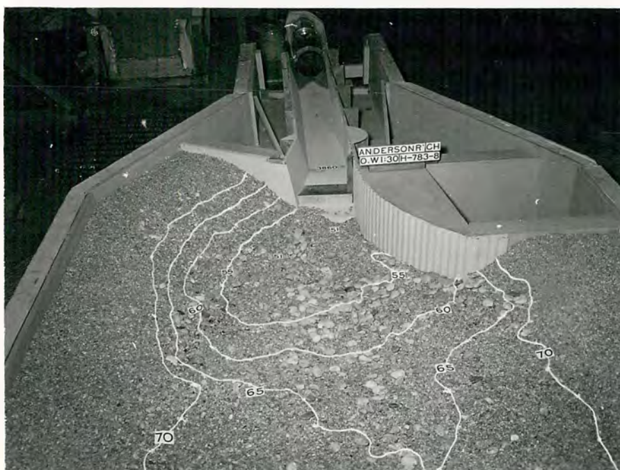
B. Scour after 15 minutes model operation at 4210 cfs.
