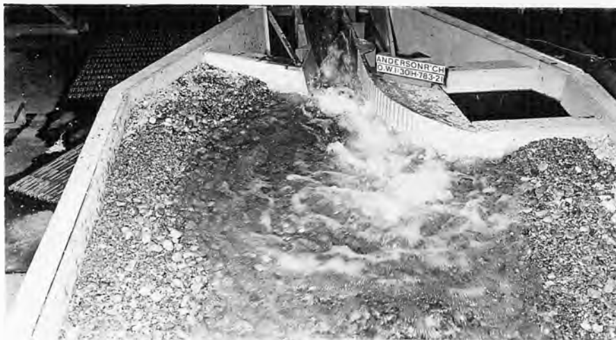
B. Flow in diversion and river channels of model with a discharge of 4210 cfs at 80 f/s velocity.
