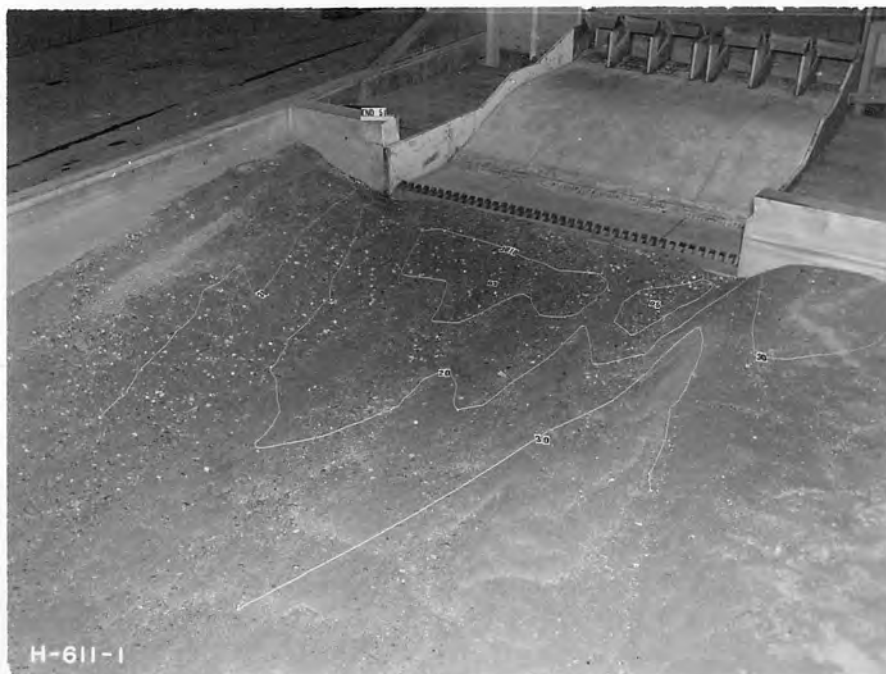
B. Scour after 45 minutes operation at 200,000 second-foot
