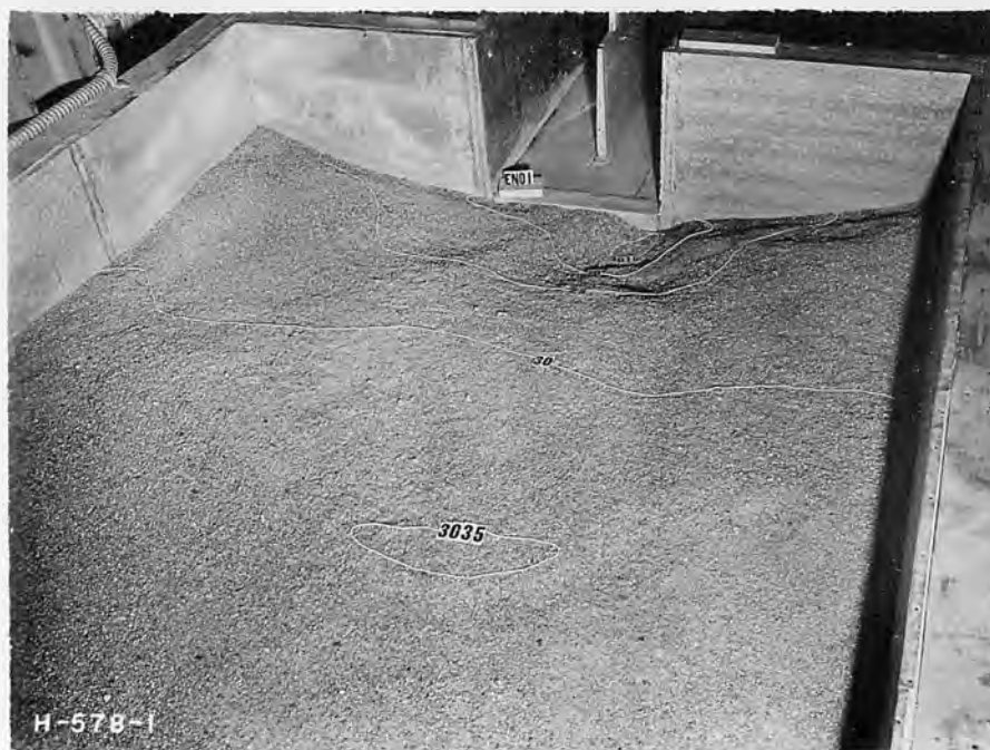
A. Scour after 1 hour operation at left valve at 930 second-feet
