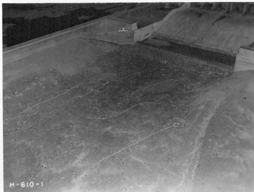
B. Scour after 45 minutes operation at 200,000 second-feet
