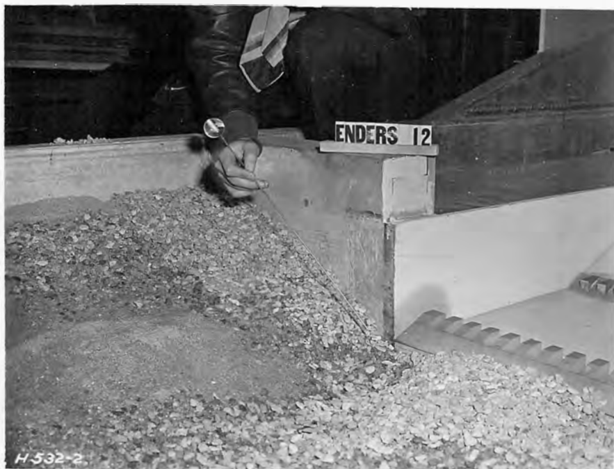
B. Scour at end of right training wall after 95 minutes operation at 200,000 second-feet, tailwater curve A
