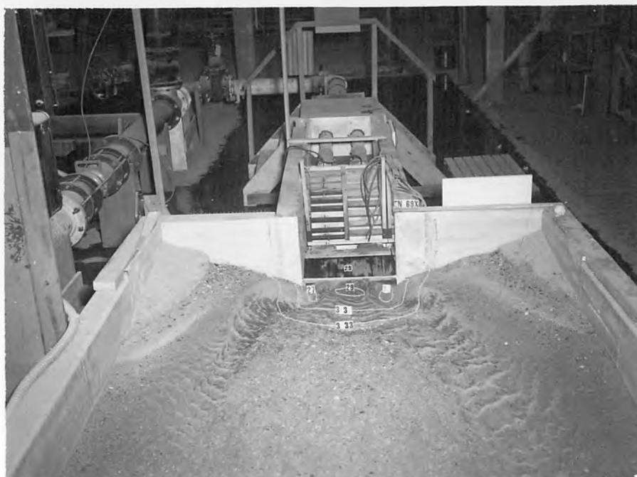
A. 50 - 100 mesh-sand - Both valves, discharge 1360 second-feet
