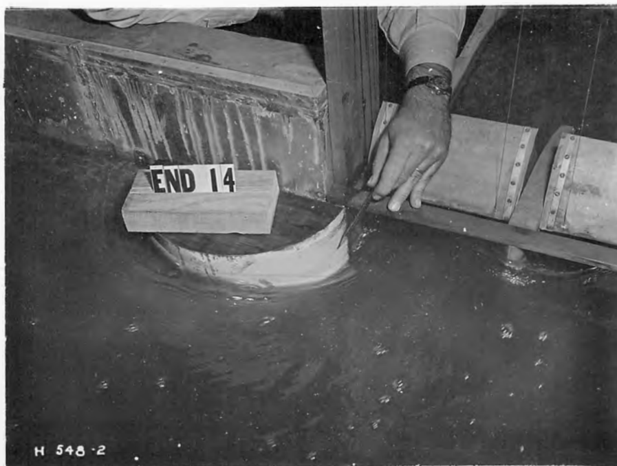
B. Drawdown at left training wall nose with a discharge of 200,000 second-feet
