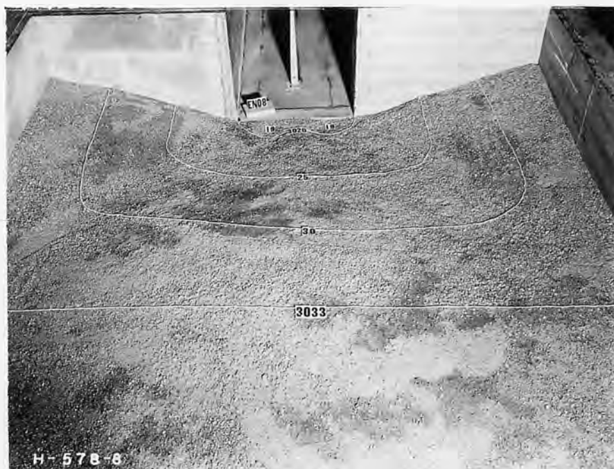
B. Scour after 1 hour operation of both valves at 1360 second-feet
