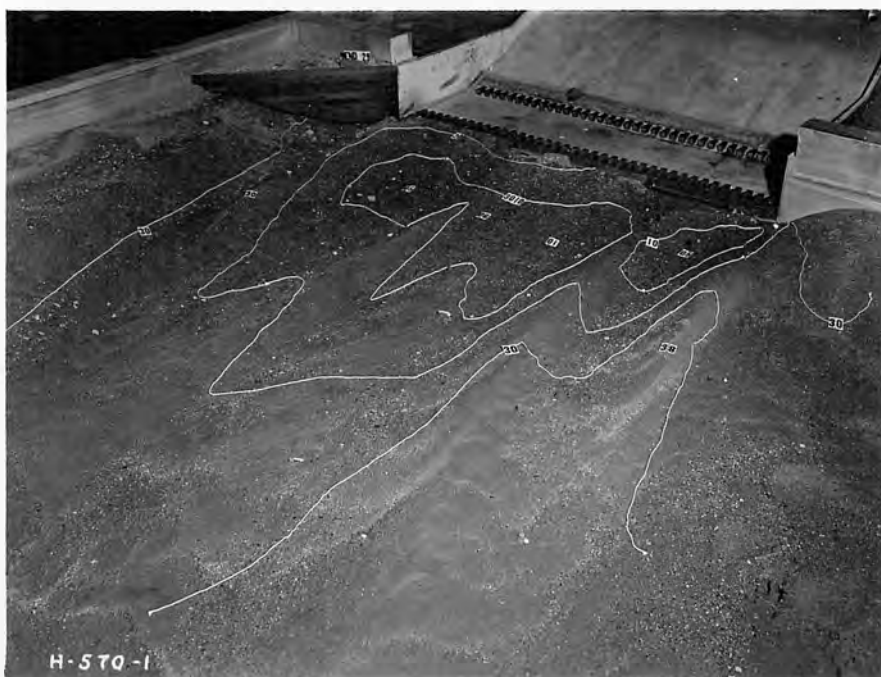
B. Scour after 45 minutes operation at 200,000 second-feet
