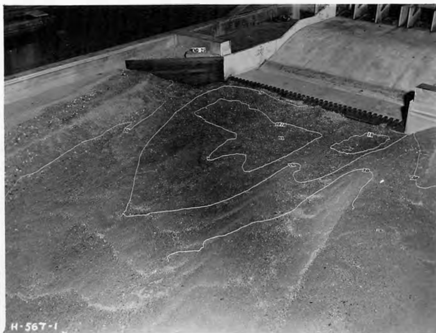
B. Scour after 45 minutes operation at 200,000 second-feet
