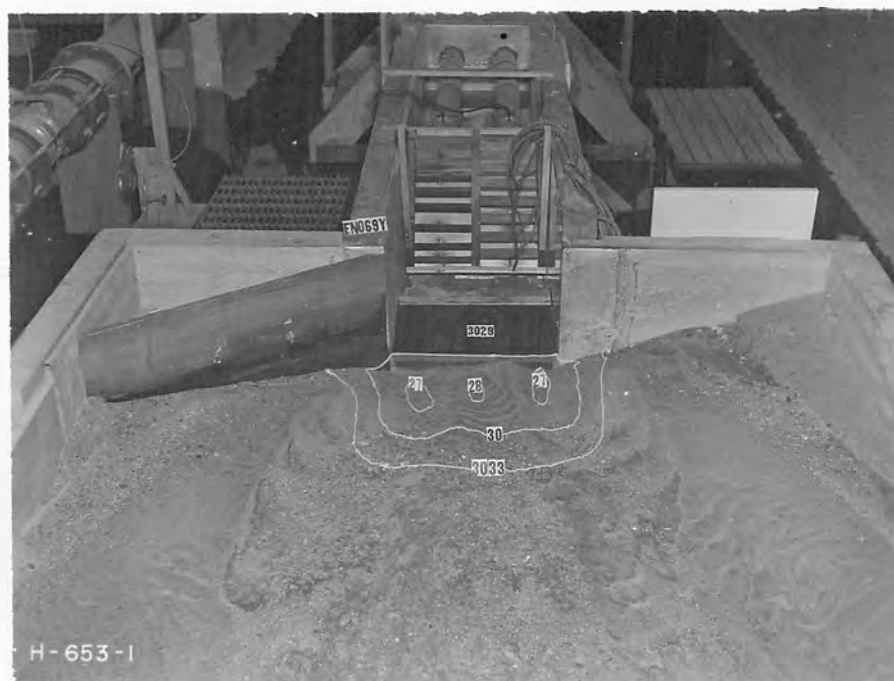
B. 100 - 200 + mesh-sand - Both valves, discharge 1360 second-feet
