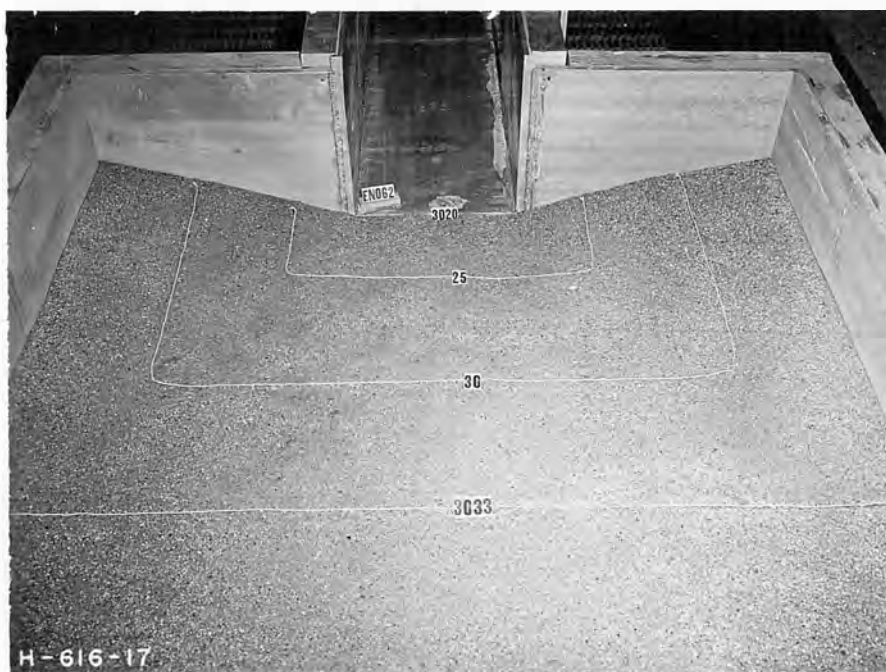
B. Scour after 1 hour operation of both valves at 1360 second-feet
