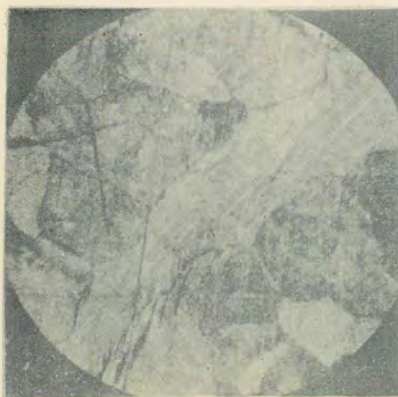
Fig. 81. Antimony specimen slightly cavitated; 250 times enlarged.
