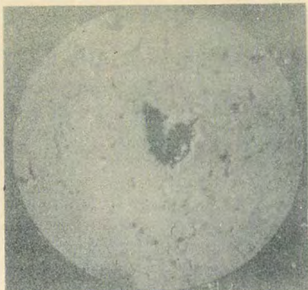
Fig. 100. Glass specimen weakly cavitated in water; 220 times enlarged. (The strong damage in the center deserves special attention; the material behaved as though it had become plastic. The sharp edges ordinarily present in fractured glass are not present.)
