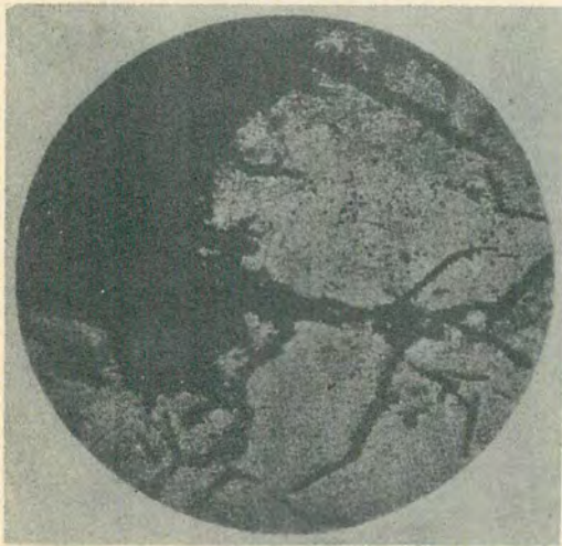
Fig. 7. Destruction in cast iron (according to Engleson [19]); 150 times enlarged.
