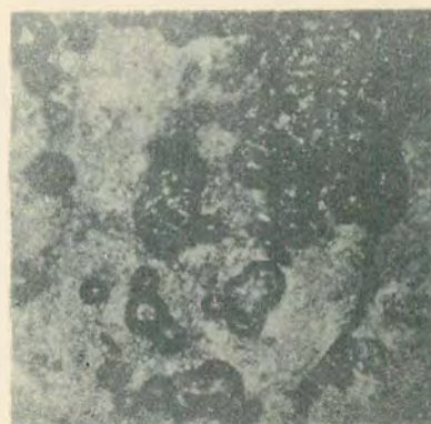
Fig. 97. Magnesium specimen cavitated in water 20 min; about 130 times enlarged. (Within the existing larger cavitation pits, smaller points of attack are visible.)
