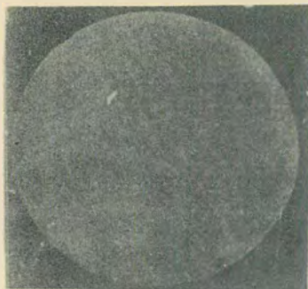
Fig. 54. Aluminum specimen cavitated in ethyl ether for 17 minutes; two times enlarged.
