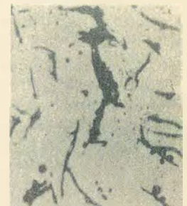
Fig. 16. Attack upon gray cast iron after 60,000 impacts with impact apparatus. 16a before test; 16b after test. (According to Ackeret and de Haller [5]); 120 times enlarged.
